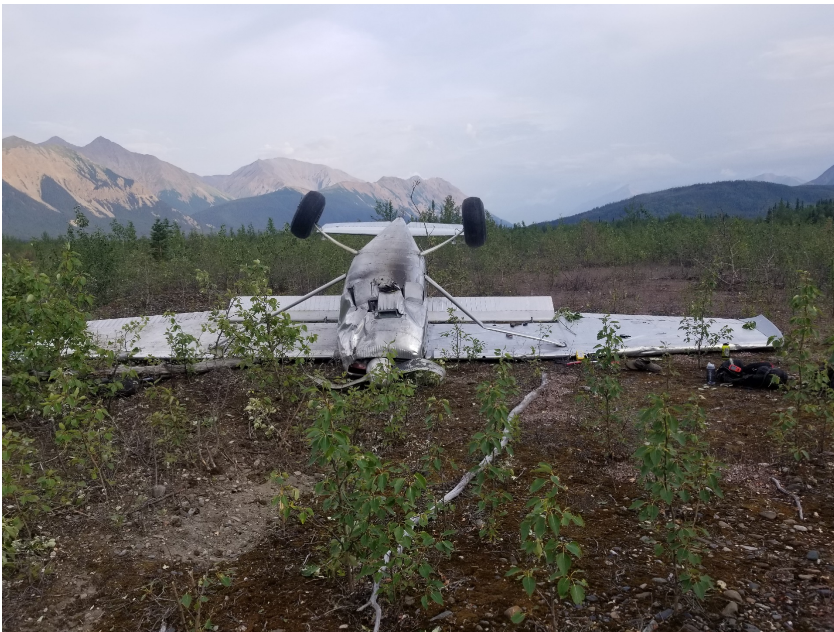
Photo 2 - Wreckage exhibiting damage to the fuselage, right wing, lift strut and propeller. (Photograph courtesy of the owner.)
