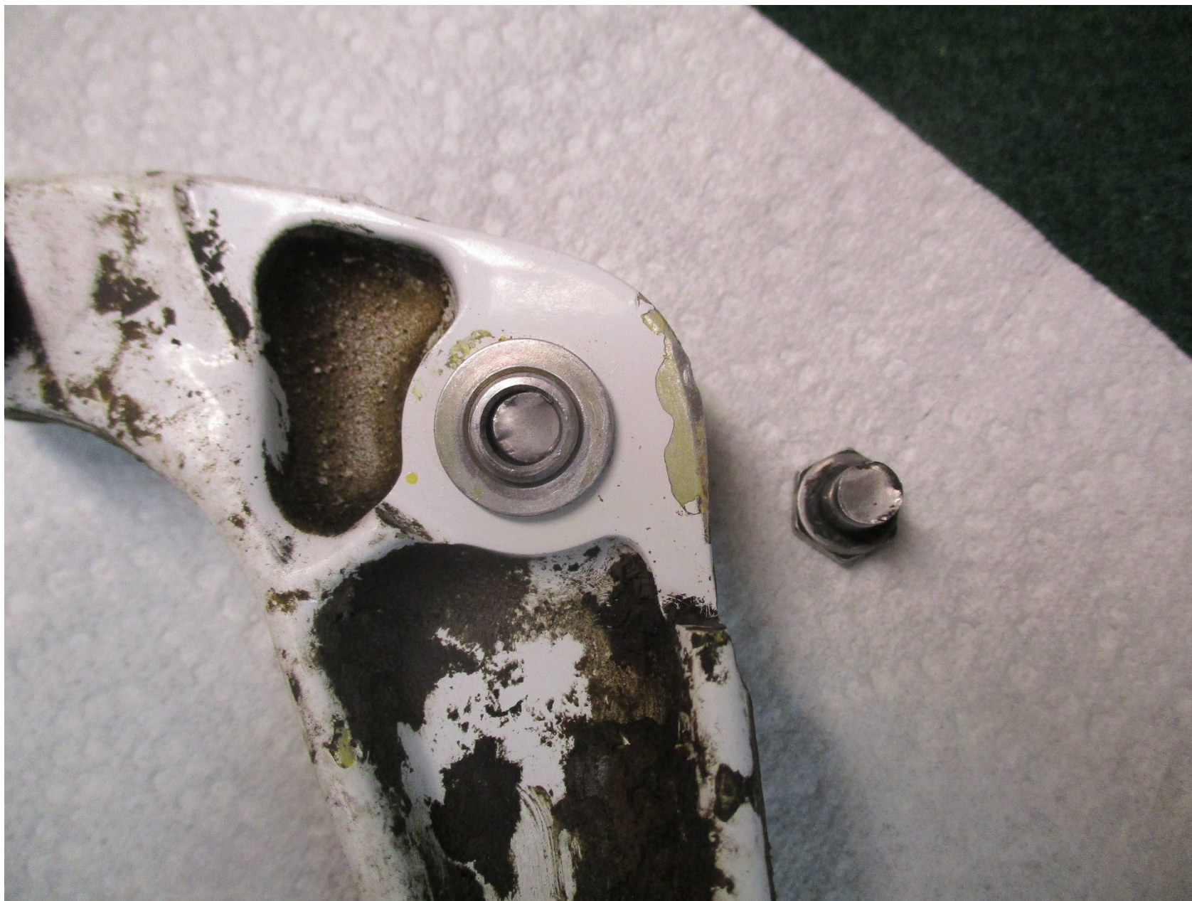
Photo 2 – Accident airplane's sheared bellcrank pivot bolt with smeared fracture features and deformation consistent with ductile overstress fracture from shear loading.
