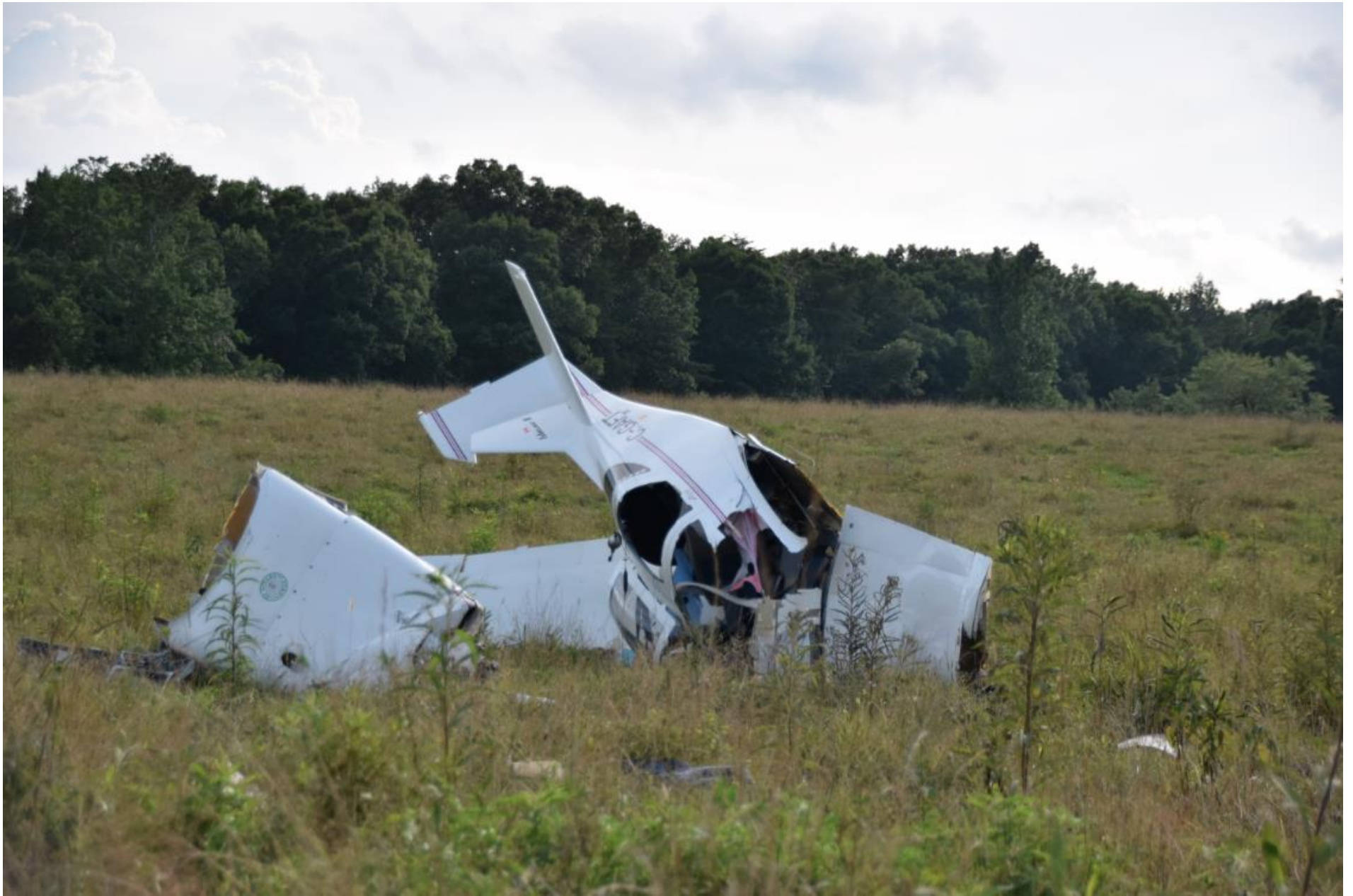
Photo 1 – Front view of damaged airplane with engine displaced (Photo courtesy of the local law enforcement)
