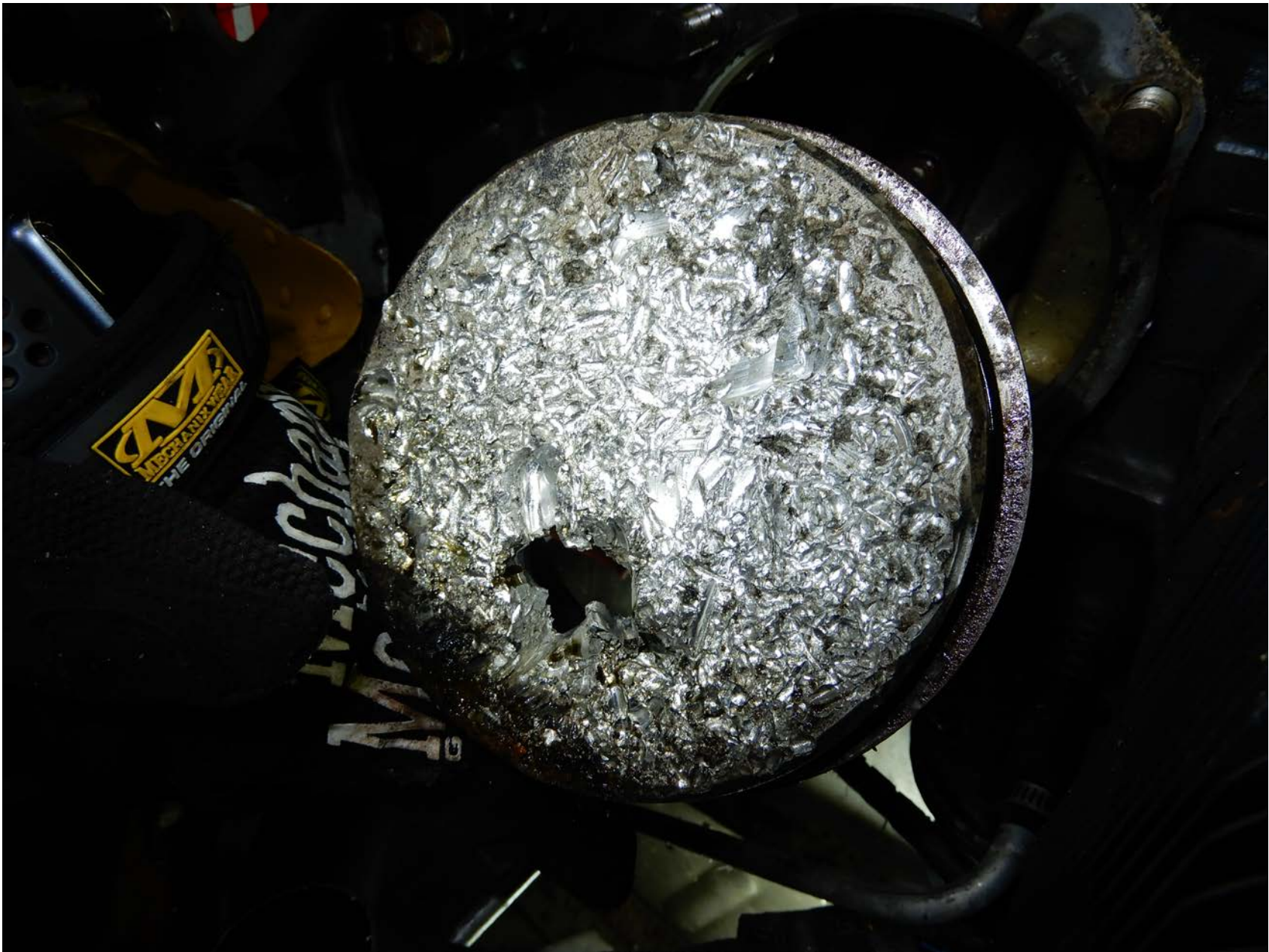
Photo 4 – Number 2-cylinder's piston face.
