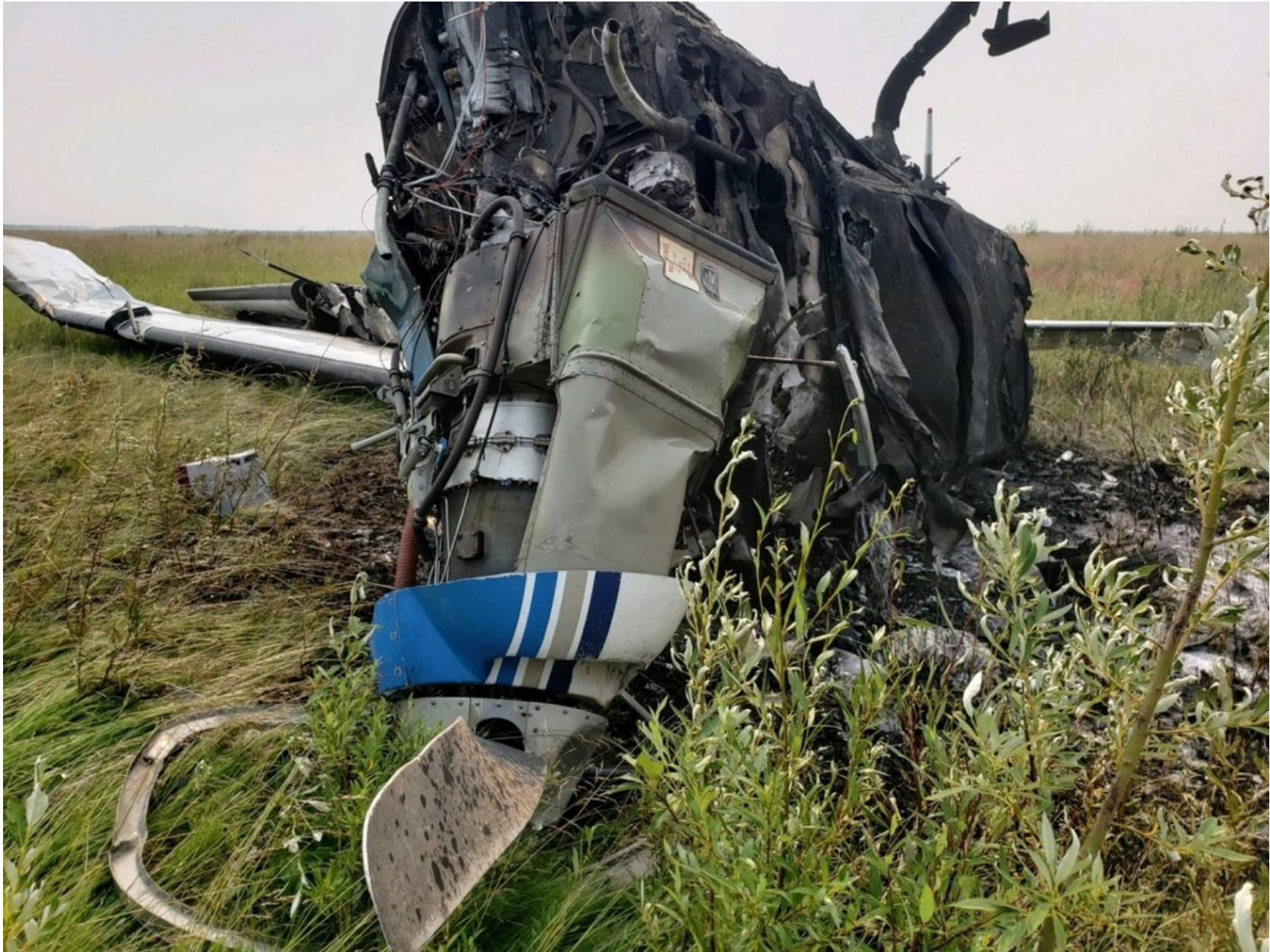
Photo 5 - Propeller, engine and front fuselage exhibiting significant impact deformation. (Source: Grant Aviation)
