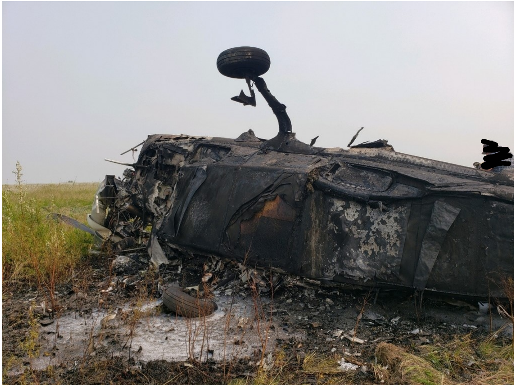
Photo 6 - Bottom fuselage exhibiting extensive fire damage. (Source: Grant Aviation)
