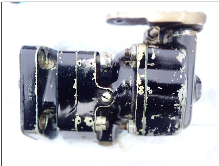
Figure 6. Propeller governor after removal.
