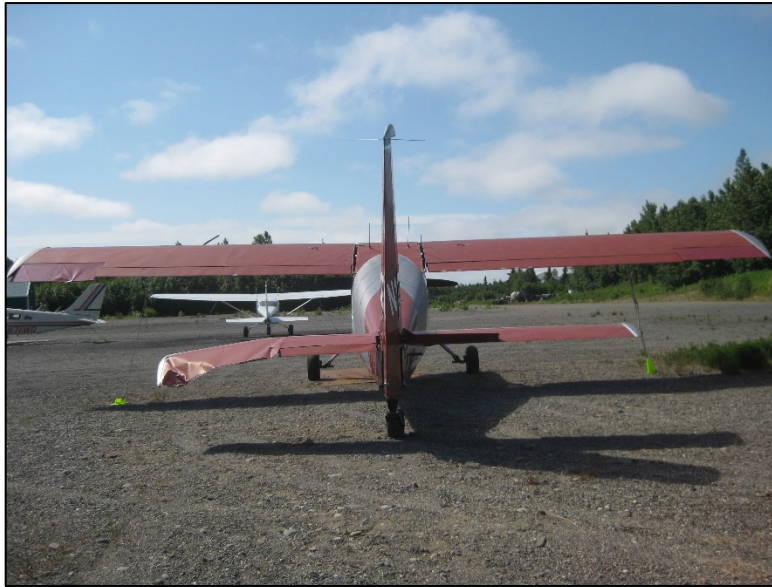
Figure 2. The airplane before the examination exhibiting substantial damage to the stabilator and left aileron.
