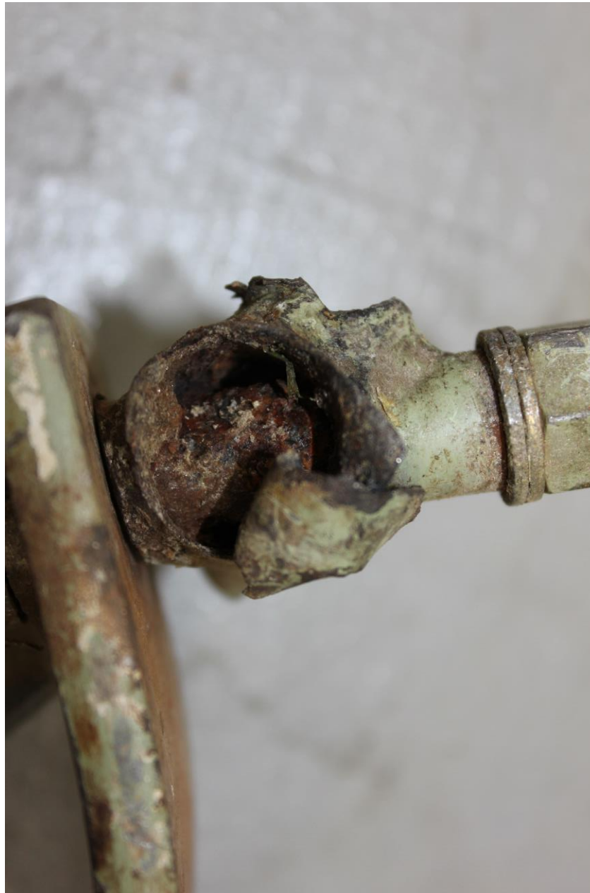
Photo 4 – View of corroded tailwheel attach bolt (Photo courtesy of the NTSB)
