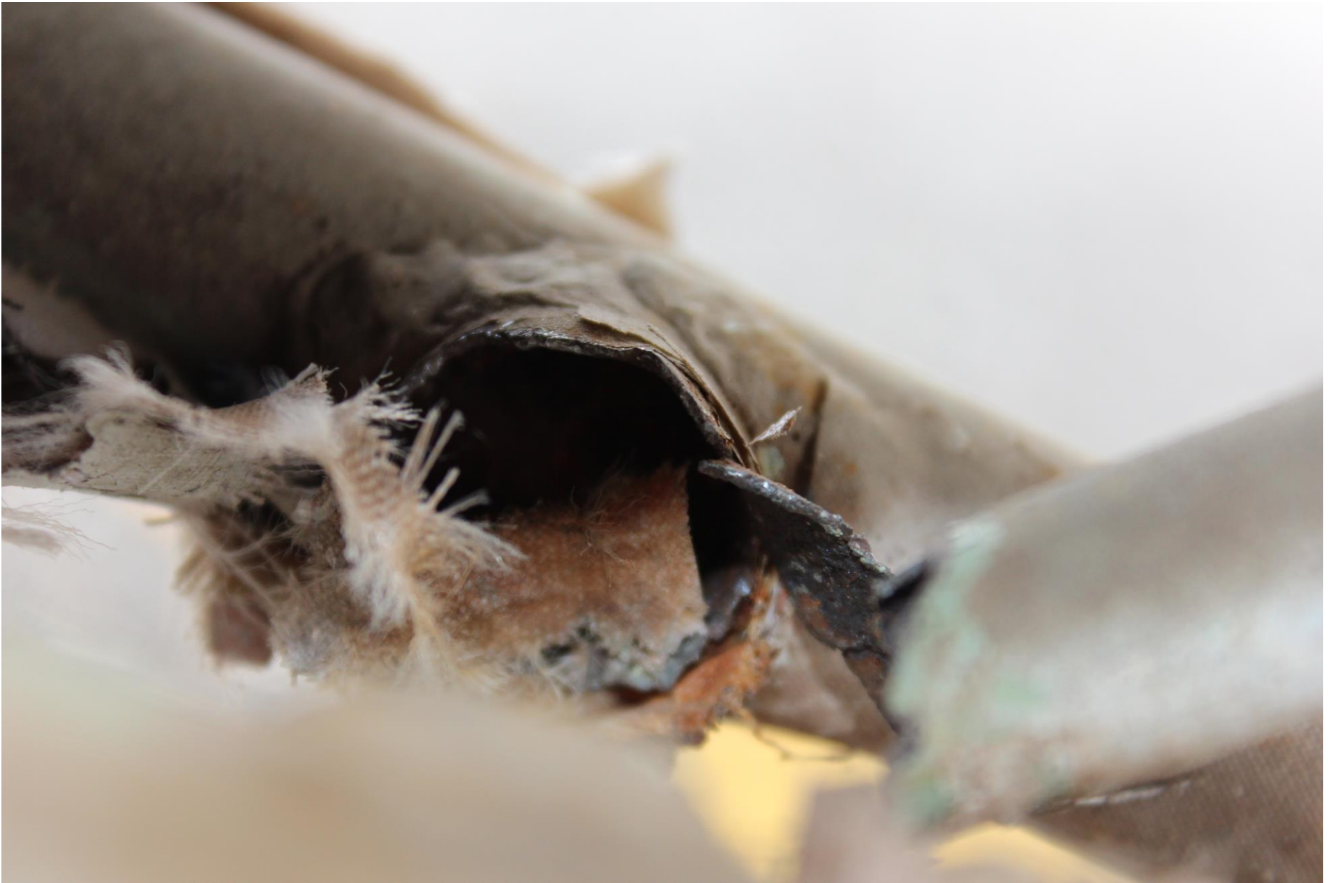
Photo 3 – View of corroded tailwheel mount cross-tube (Photo courtesy of the NTSB)
