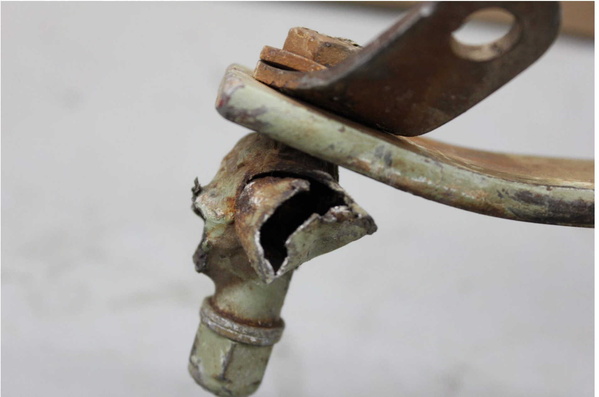
Photo 5 – Additional view of corroded tailwheel attach bolt (Photo courtesy of the NTSB)
