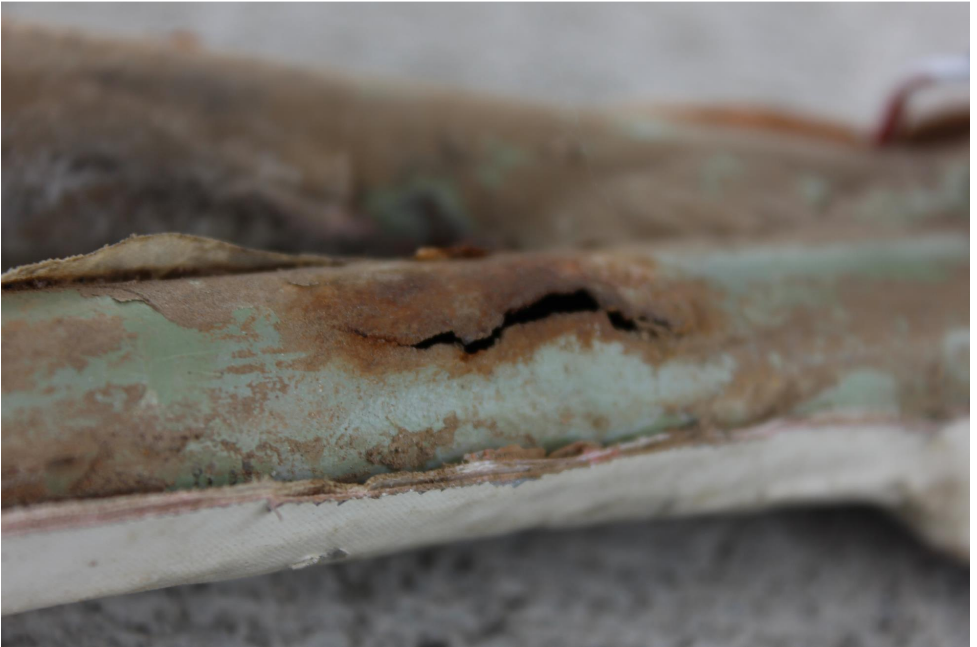
Photo 2 – View of corroded aft lower fuselage tube (Photo courtesy of the NTSB)
