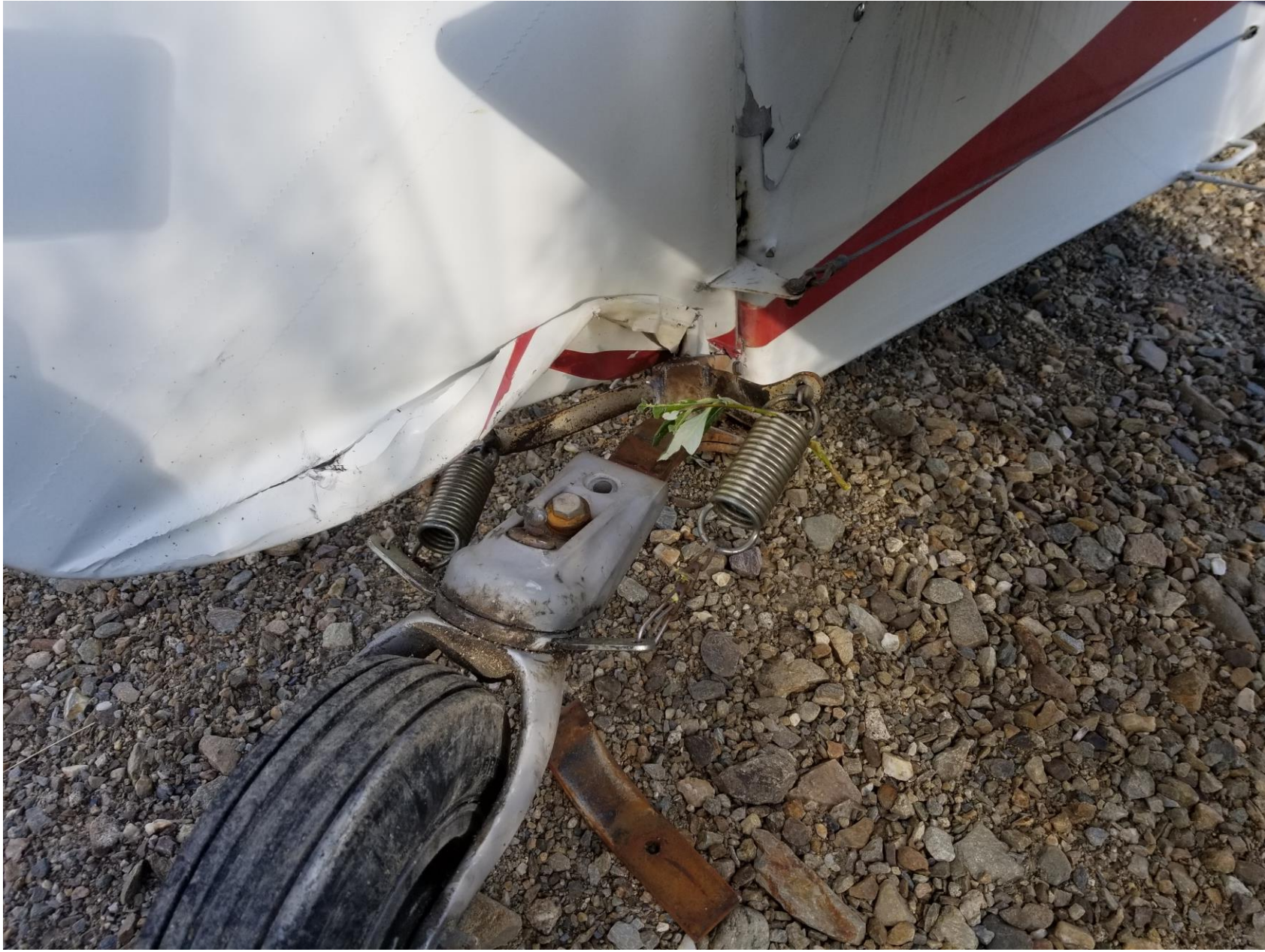
Photo 6 - View of damaged rudder (Photo courtesy of the FAA)
