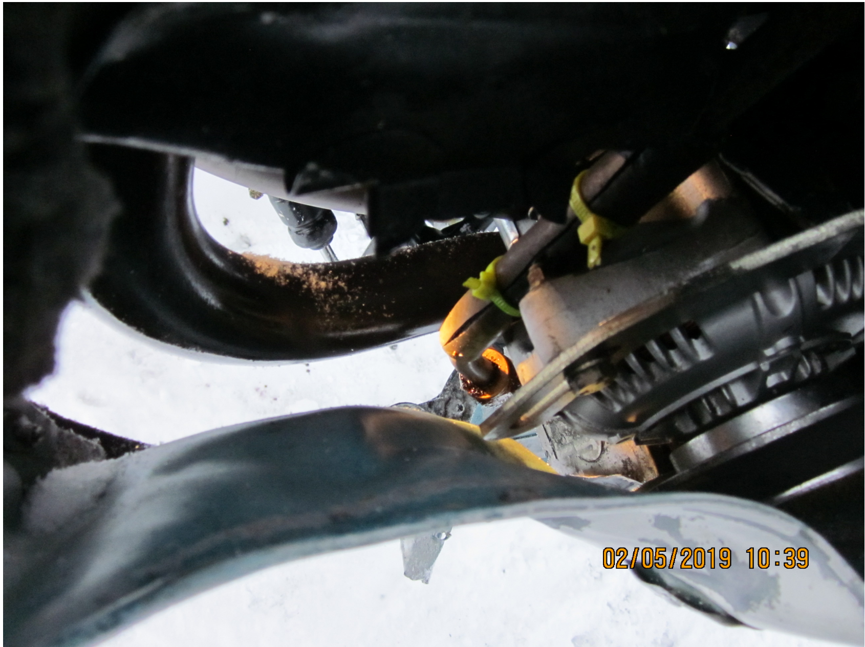
Photo 3 - Loose B-Nut Looking Down through Engine (FAA Photo)
