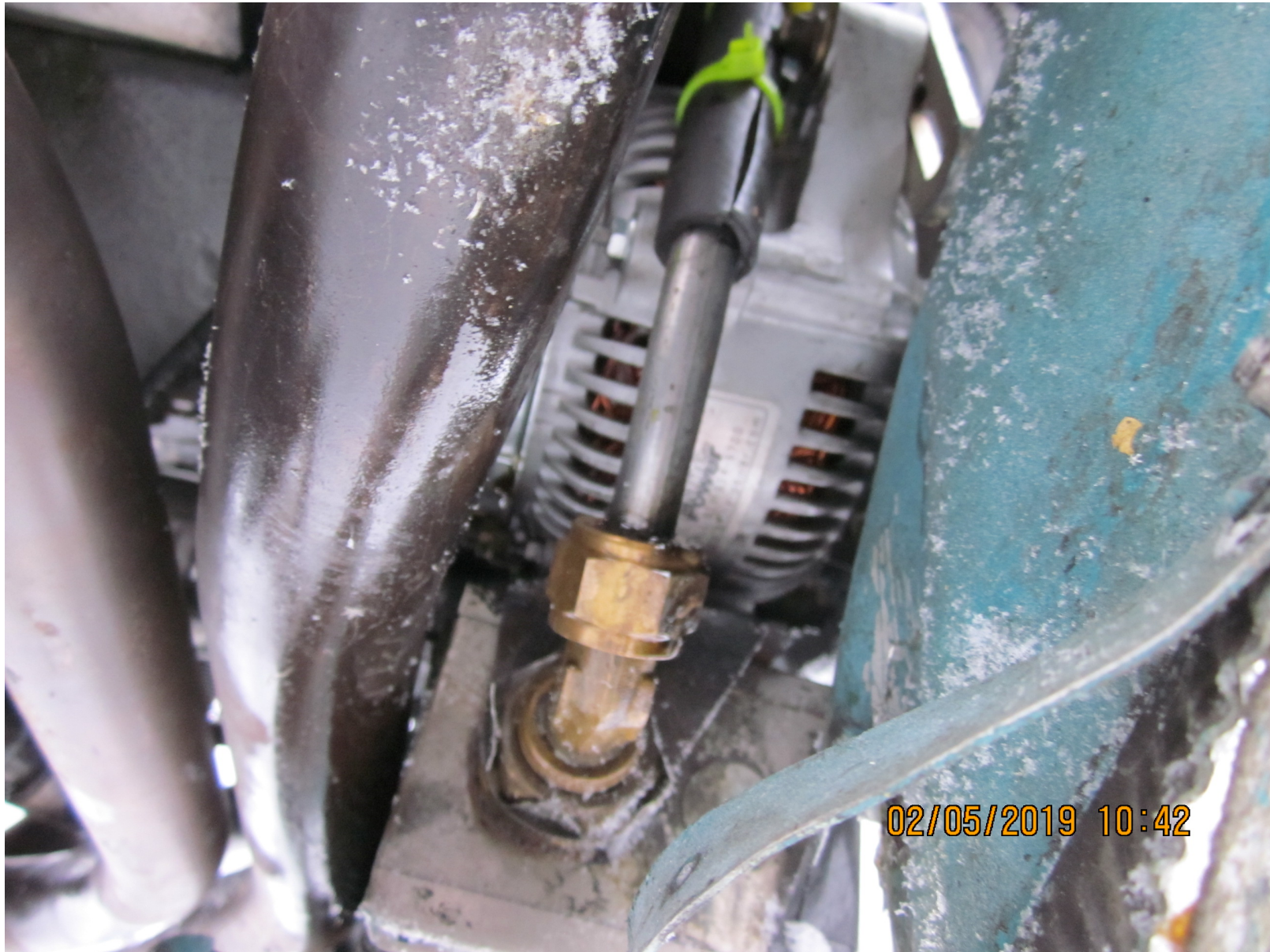
Photo 1 – Loose B-Nut Found on Oil Cooler, Looking Up (FAA Photo)
