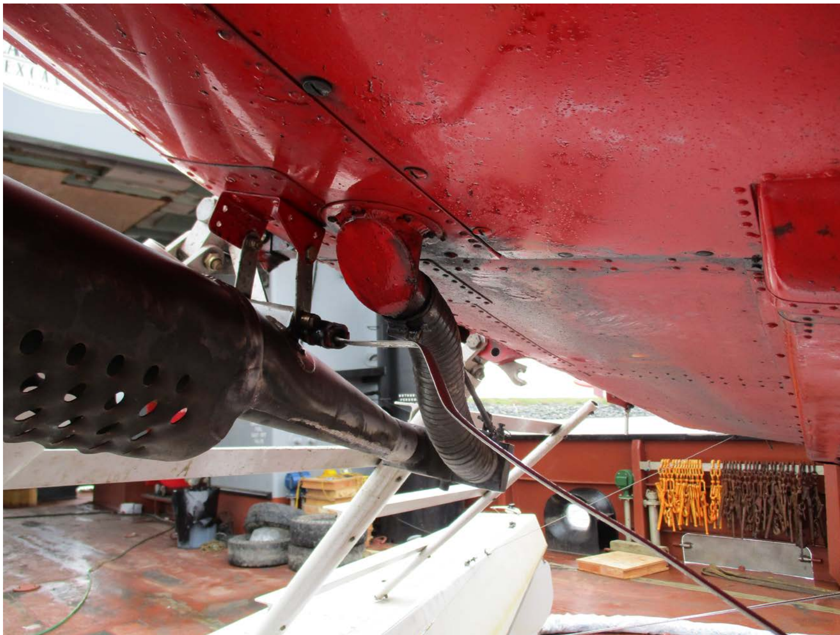
Photo 6 – Left float attach forward flying wire compression signature.
