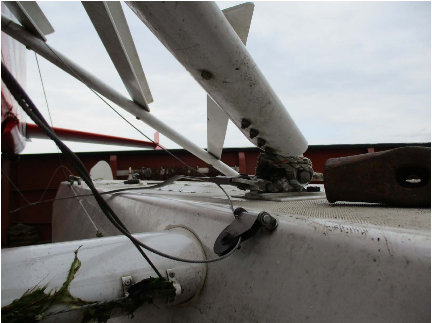
Photo 7 – Left float attach rear flying wire compression signature.
