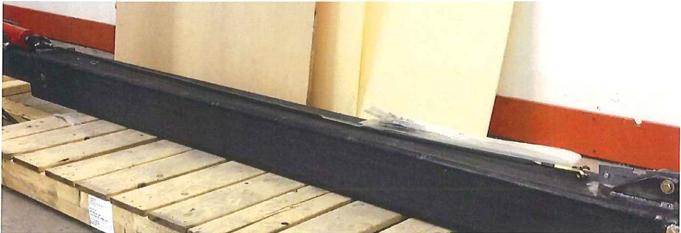
Figure 15 – Showing Test Specimen (Pull Fuse) Failure at 3600 psi (9003 lbf.) NOTE: Clevis end failed prior to pull fuse limit.
