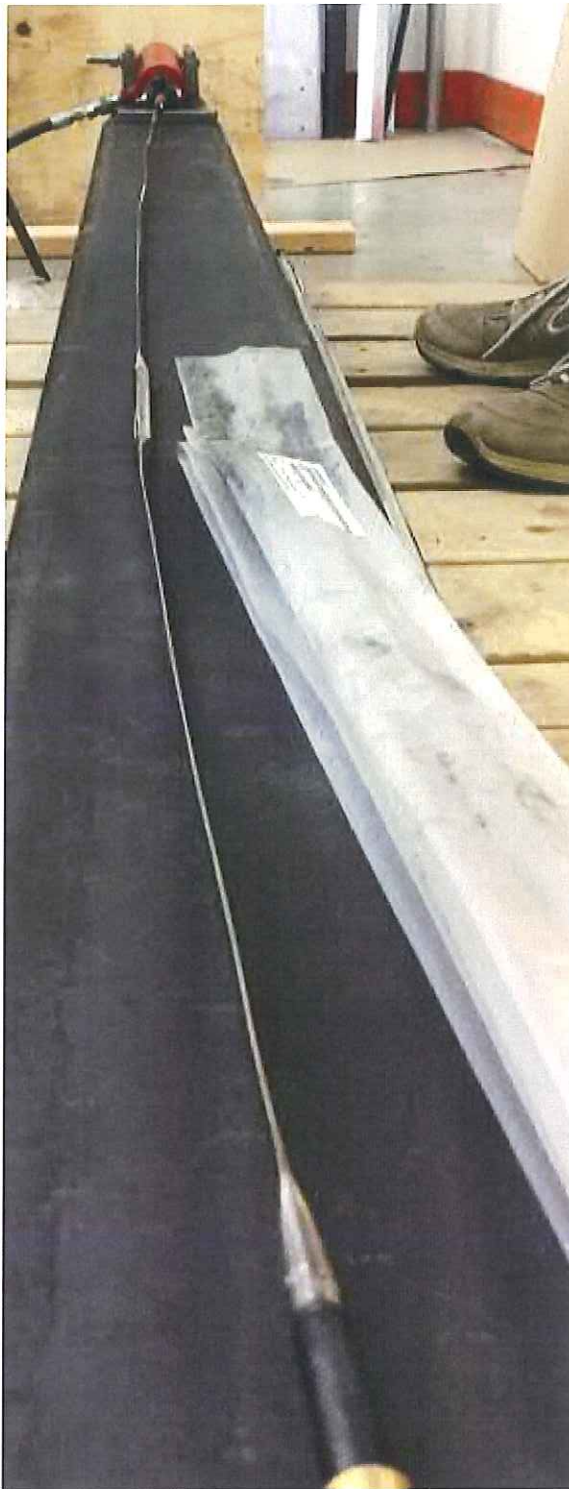
Figure(s) 17 – Showing Test Specimen (Pull Fuse) Failure at 3600 psi (9003 lbf.) NOTE: Clevis end failed prior to pull fuse limit.
