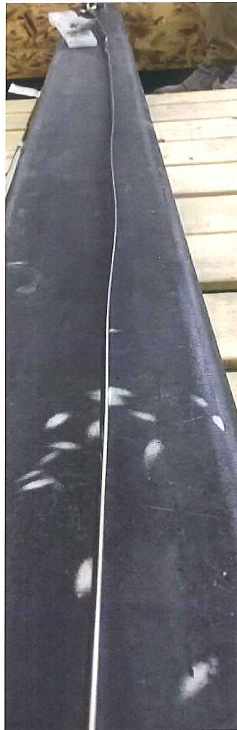
Figure(s) 17 – Showing Test Specimen (Pull Fuse) Failure at 3600 psi (9003 lbf.) NOTE: Clevis end failed prior to pull fuse limit.
