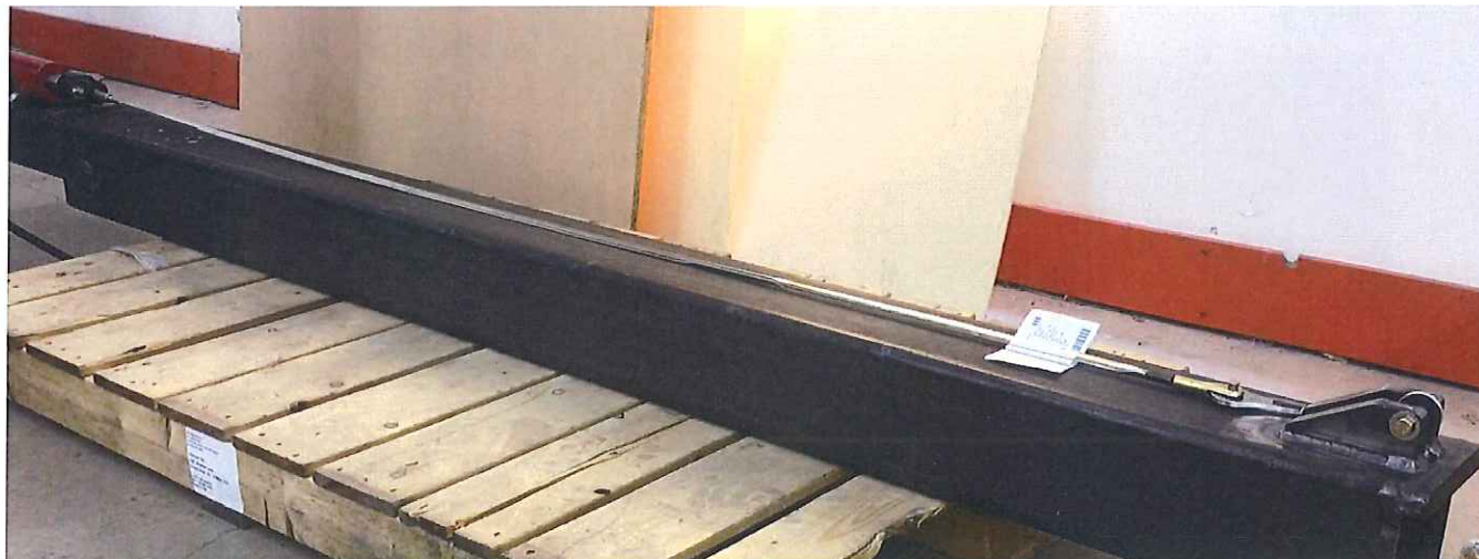
Figure 7 – Showing Test Specimen (Pull Fuse) Failure at 1550 psi (3877 lbf.)
