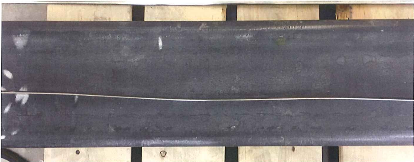
Figure 16 – Showing Test Specimen (Pull Fuse) Failure at 3600 psi (9003 lbf.) NOTE: Clevis end failed prior to pull fuse limit.
