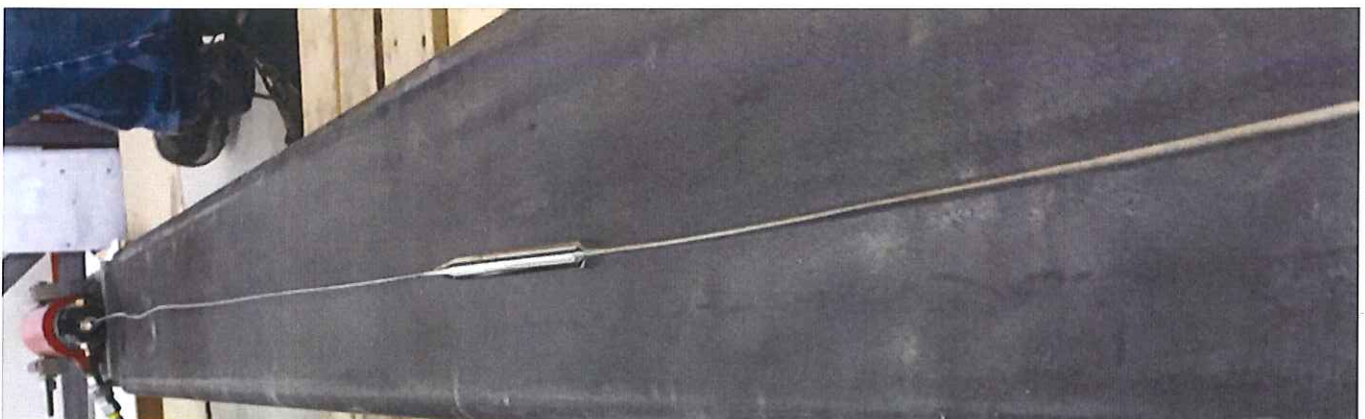
Figure 13 – Showing Test Specimen (Pull Fuse) Failure at 2800 psi (7002 lbf.)
