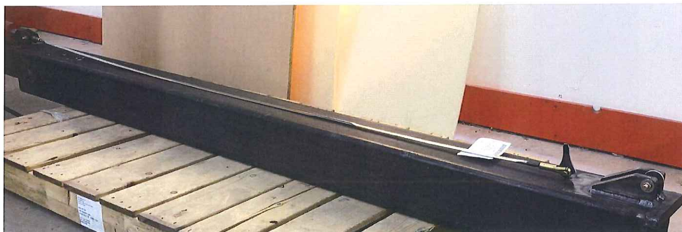
Figure 5 – Showing Test Specimen (Pull Fuse) Failure at 1000 psi (2500 lbf.)
