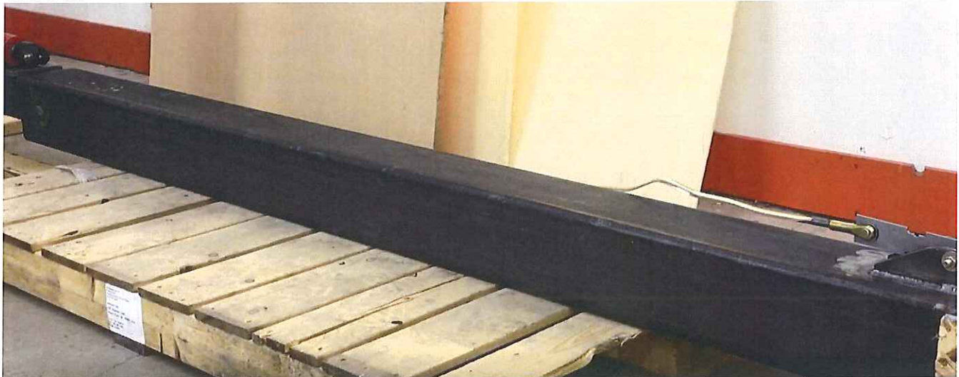
Figure 19 – Showing Test Specimen (Pull Fuse) Failure at 4000 psi (10,004 lbf.) NOTE: Clevis end failed prior to pull fuse limit.
