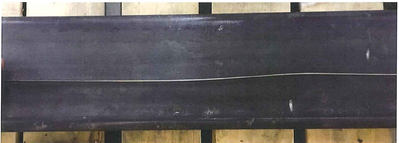
Figure 12 – Showing Test Specimen (Pull Fuse) Failure at 2800 psi (7002 lbf.)
