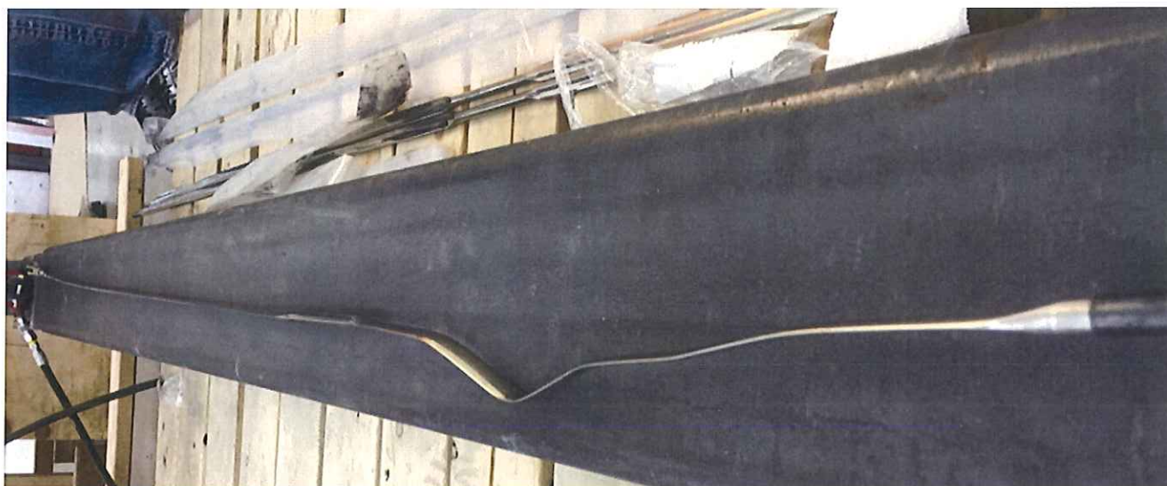
Figure 21 – Showing Test Specimen (Pull Fuse) Failure at 4000 psi (10,004 lbf.) NOTE: Clevis end failed prior to pull fuse limit.
