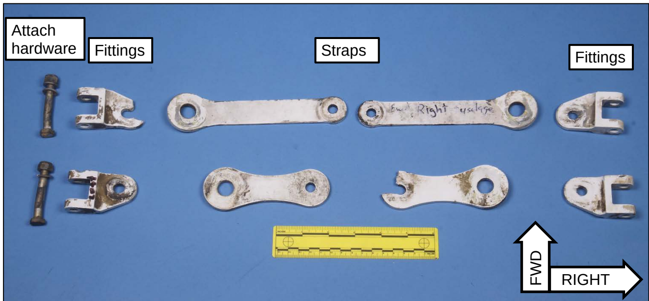
Figure 1. Overall view of the submitted left middle and left rear struts with attachment fittings and hardware (upper image) and flying wire attachment straps and fittings with attachment hardware for the lower left fittings (lower image).
