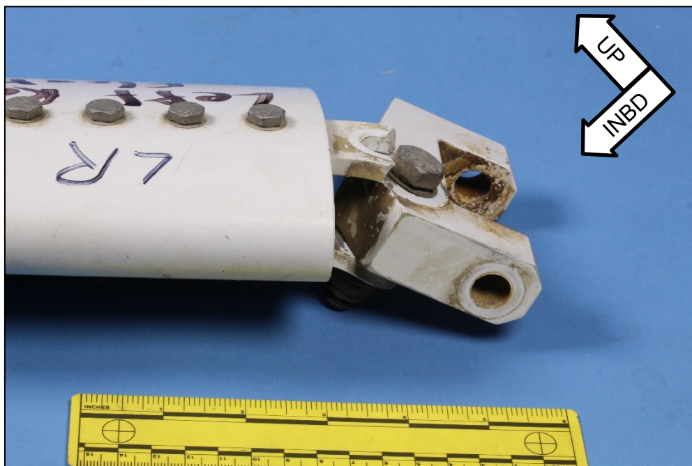
Figure 4. Lower end of the left rear strut. The inboard strap was bent downward, and the outboard strap was fractured.
