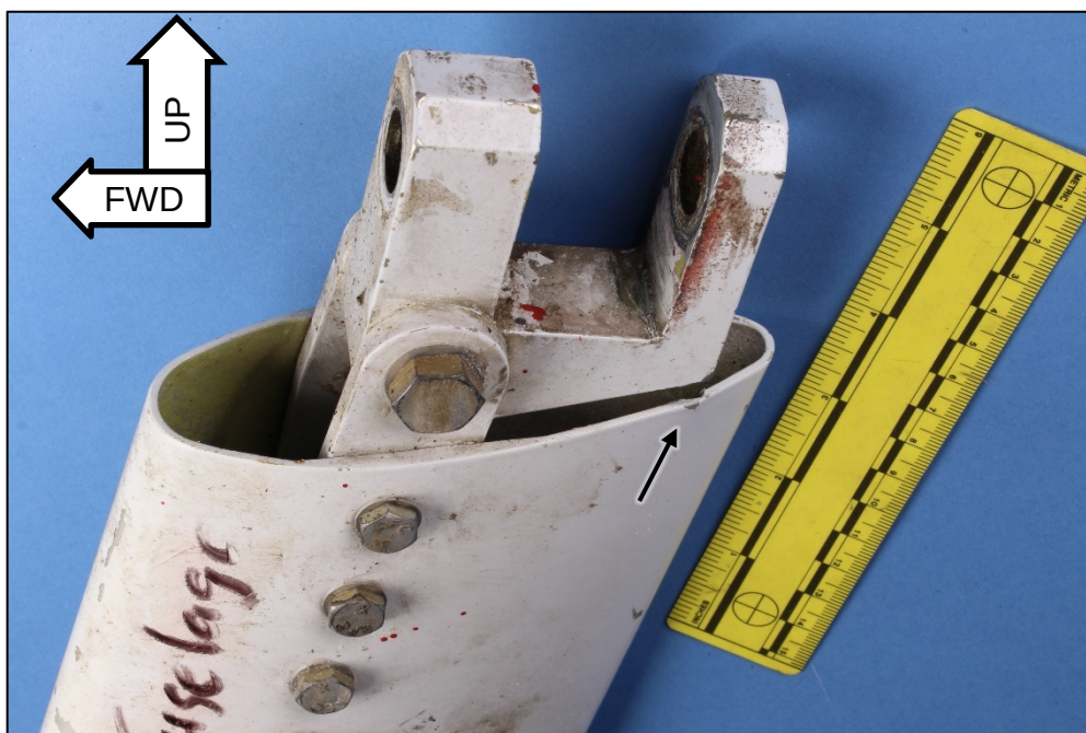
Figure 3. Intact upper end of the left middle strut. An unlabeled arrow indicates damage corresponding to contact between the strut and the aft corner of the clevis fitting.
