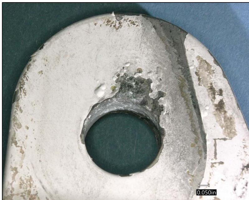
Figure 11. Optical image of the inboard side of the right rear lower flying wire attachment fitting showing corrosion with blistered paint around the flying wire attachment hole.
