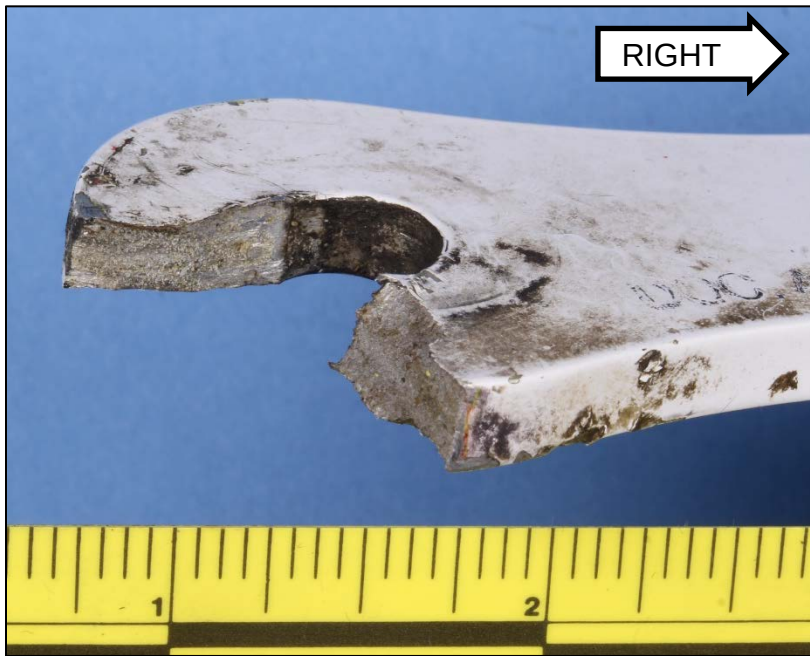
Figure 6. Fractured end of the right rear flying wire attachment strap.
