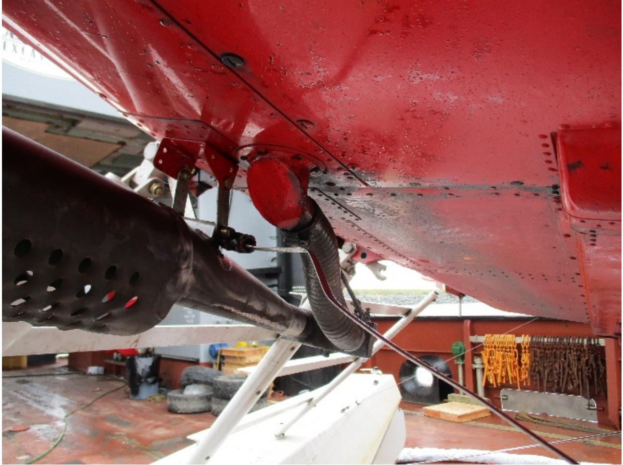
Figure 12 - Accident airplane's damaged forward streamlined tie rod.
