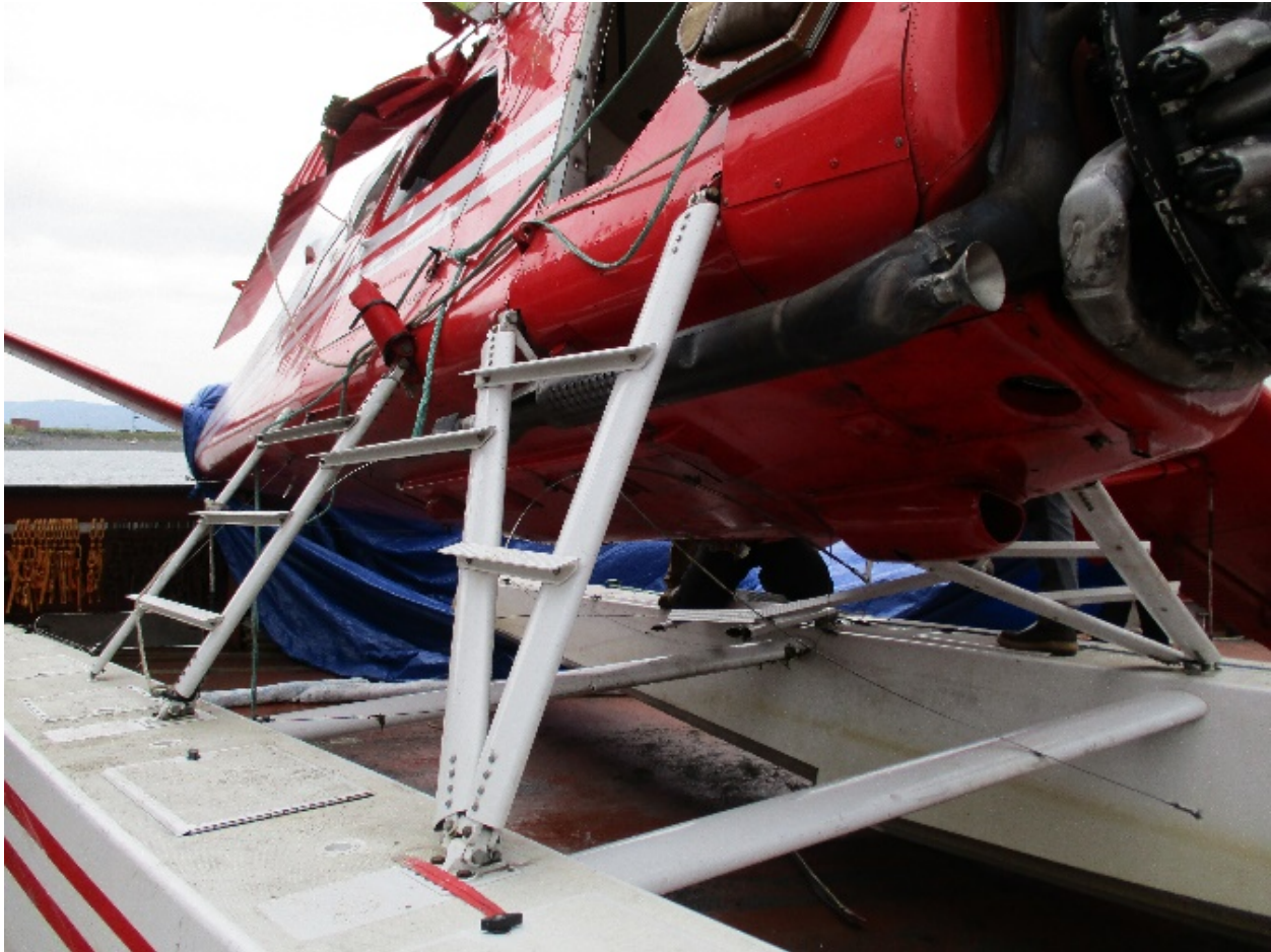
Figure 11 - Accident airplane's left side float struts.
