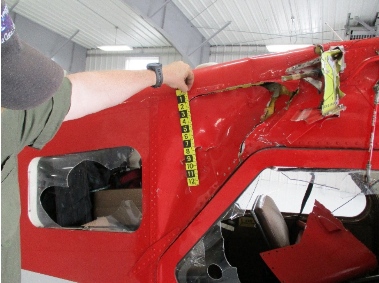
Figure 6 - Right side fuselage damage consistent with the flap and wing root impacting the fuselage during the accident sequence.
