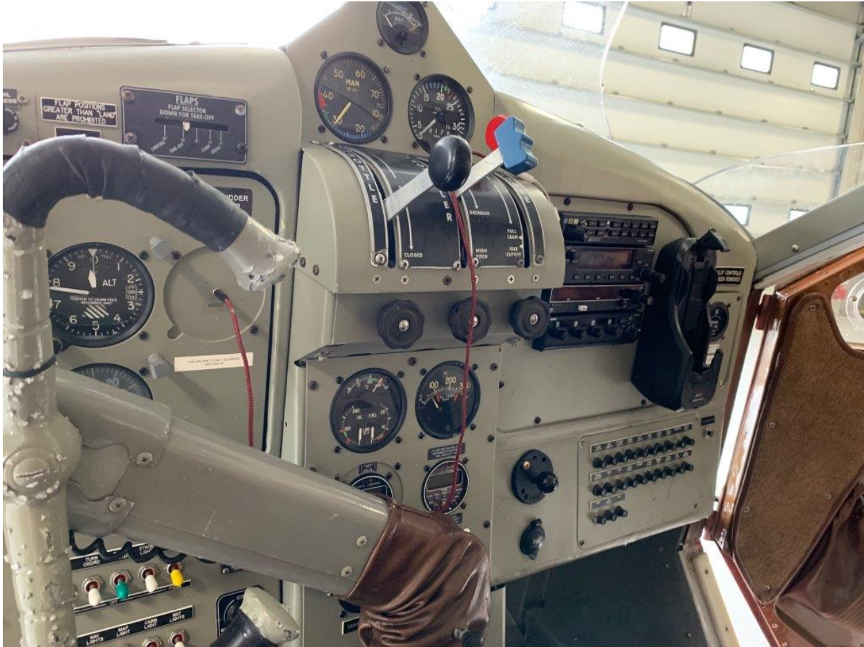
Figure 3 - Throttle quadrant and wing flap indicator of accident airplane.
