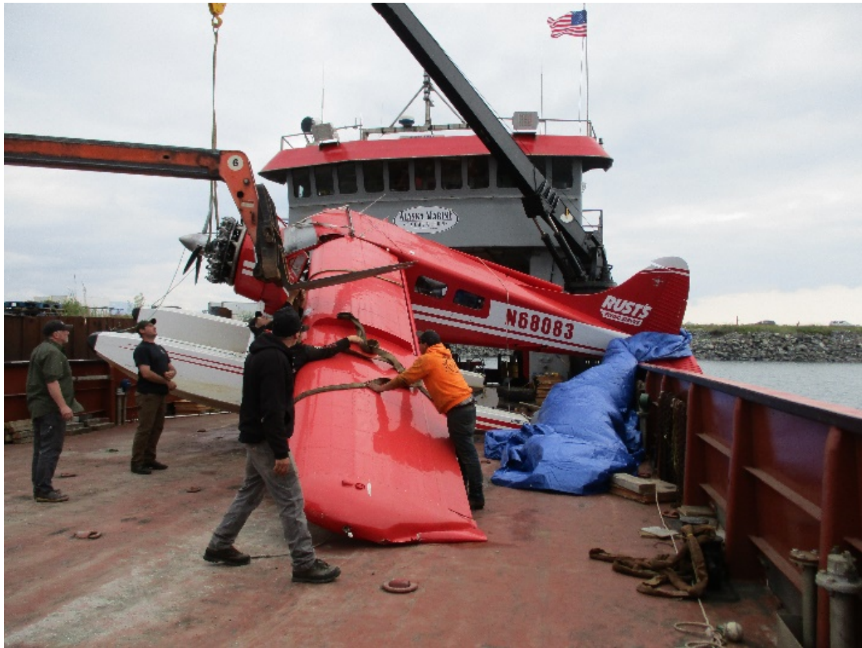
Figure 9 - Accident airplane's left wing, flap, and aileron.
