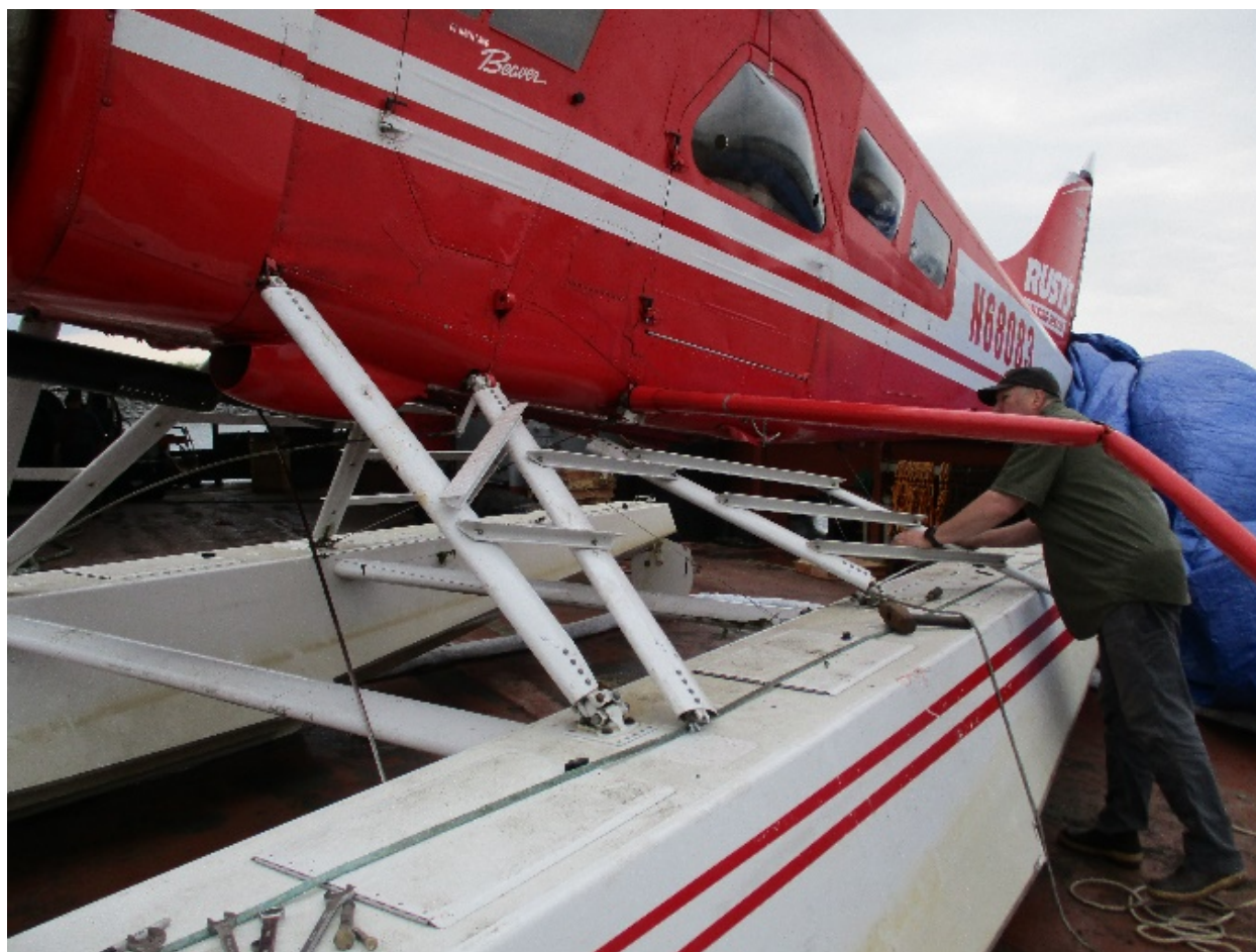
Figure 10 - Accident airplane's left side float struts.
