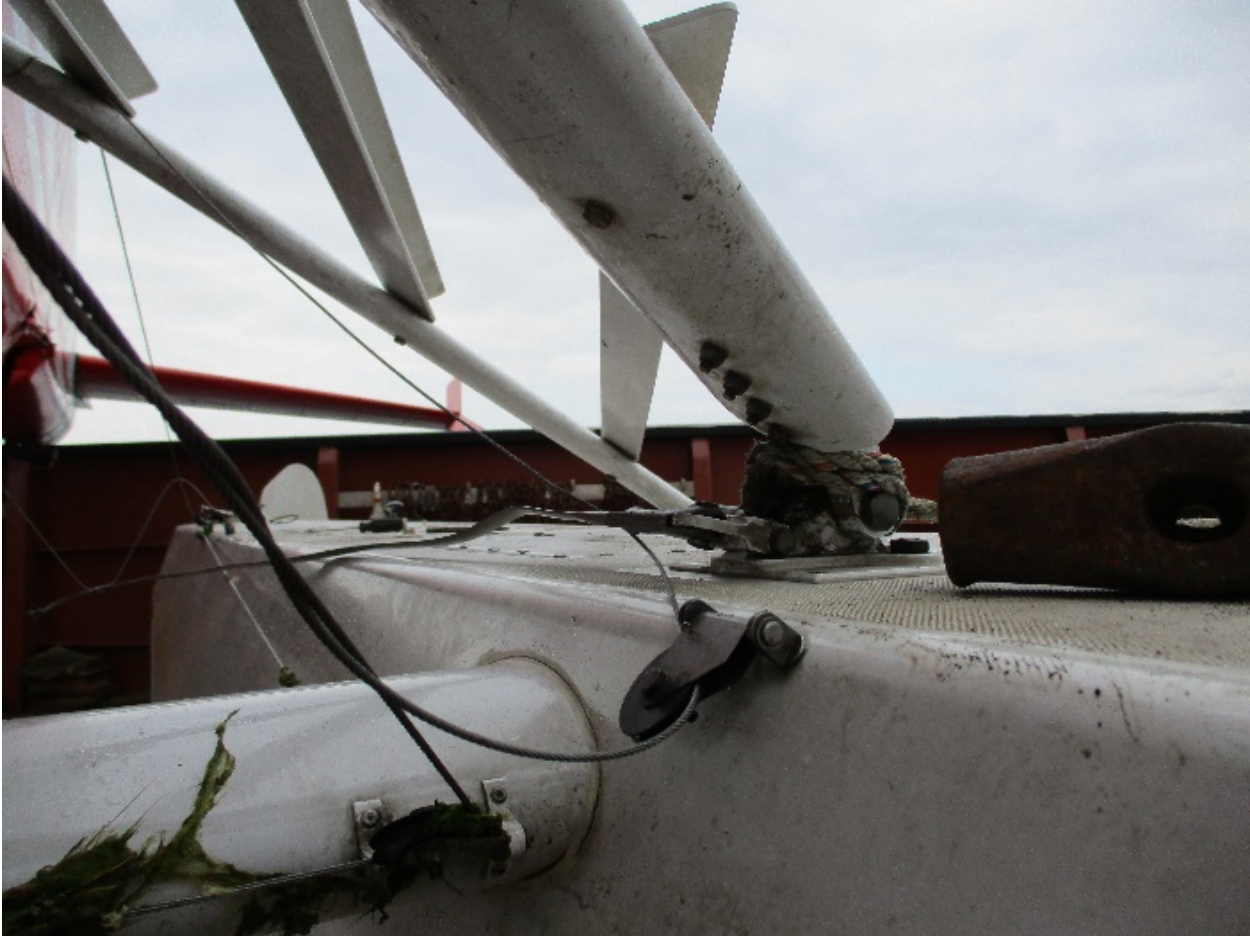
Figure 13 - Accident airplane's damaged rear streamlined tie rod.
