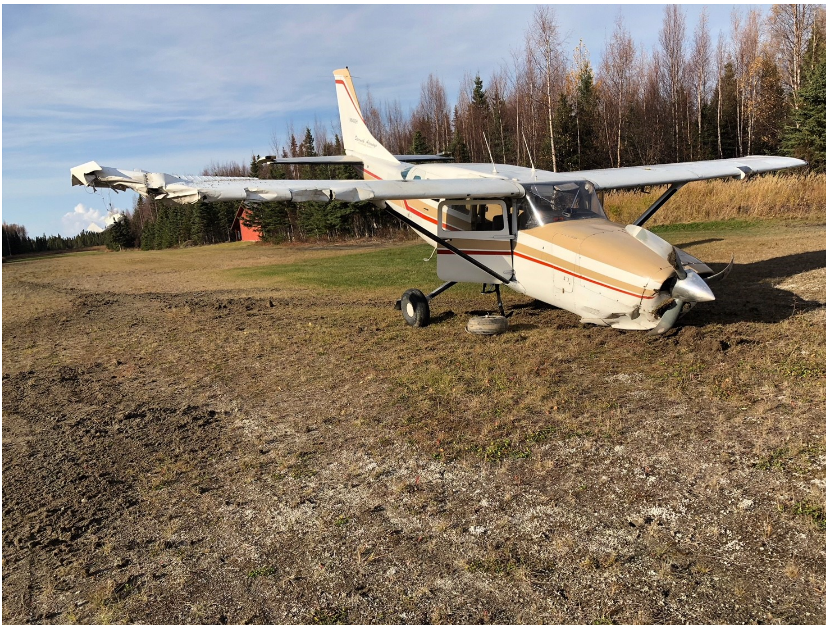
Photo 2 - Right wing and fuselage damage to N6492H Cessna 207. (Photograph compliments of Spernak Airways, Inc.)
