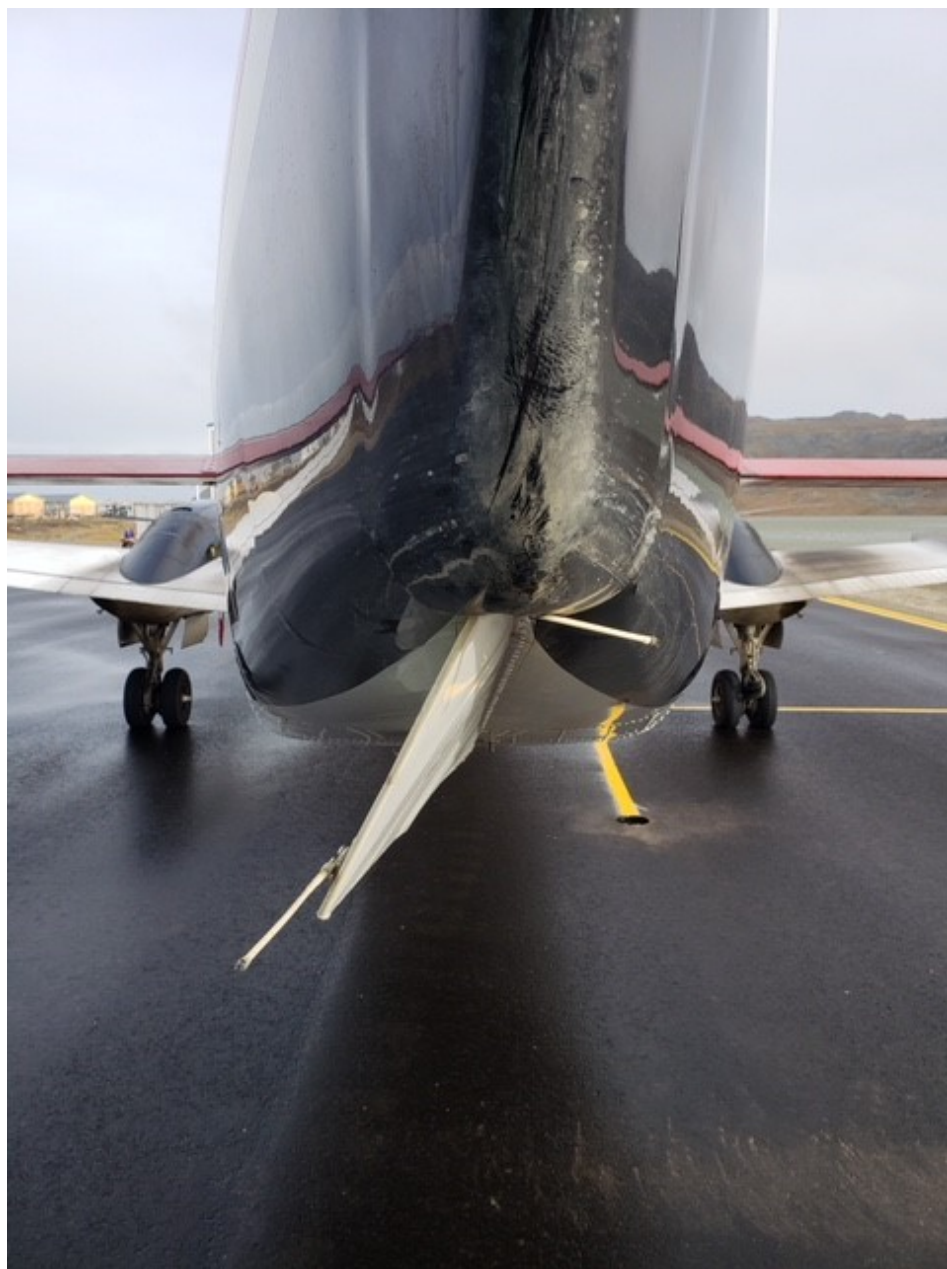
Photo 1 – Exterior damaged area of accident airplane.
