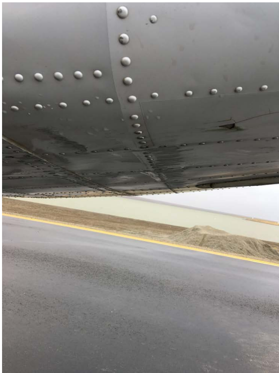
Photo 2 – Aft fuselage skin damage to accident airplane.
