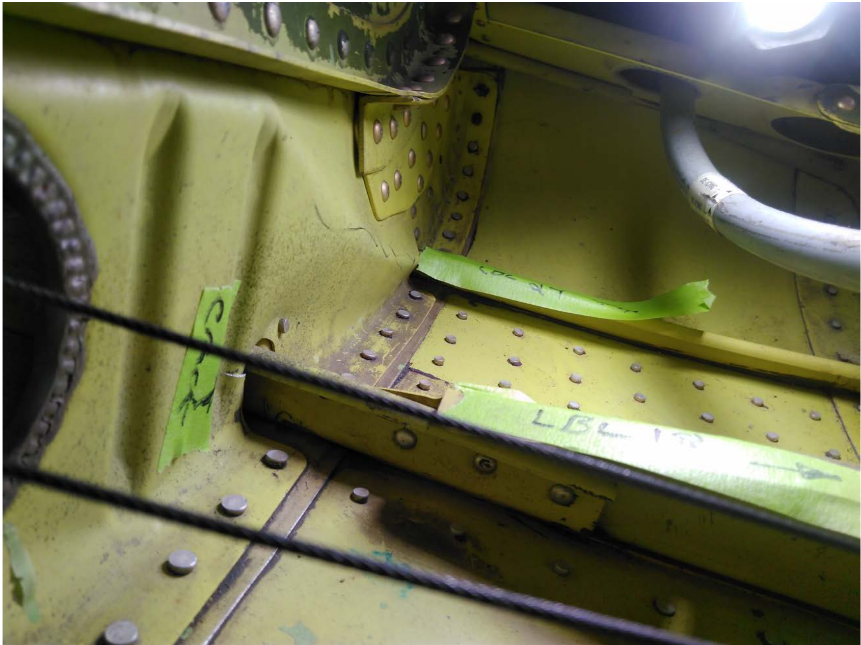
Photo 3 – Damaged bulkhead on accident airplane.
