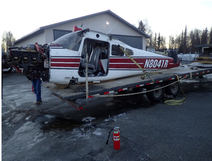
Figure 3. The airplane post-recovery with the wings, doors, cowling and empennage removed.
