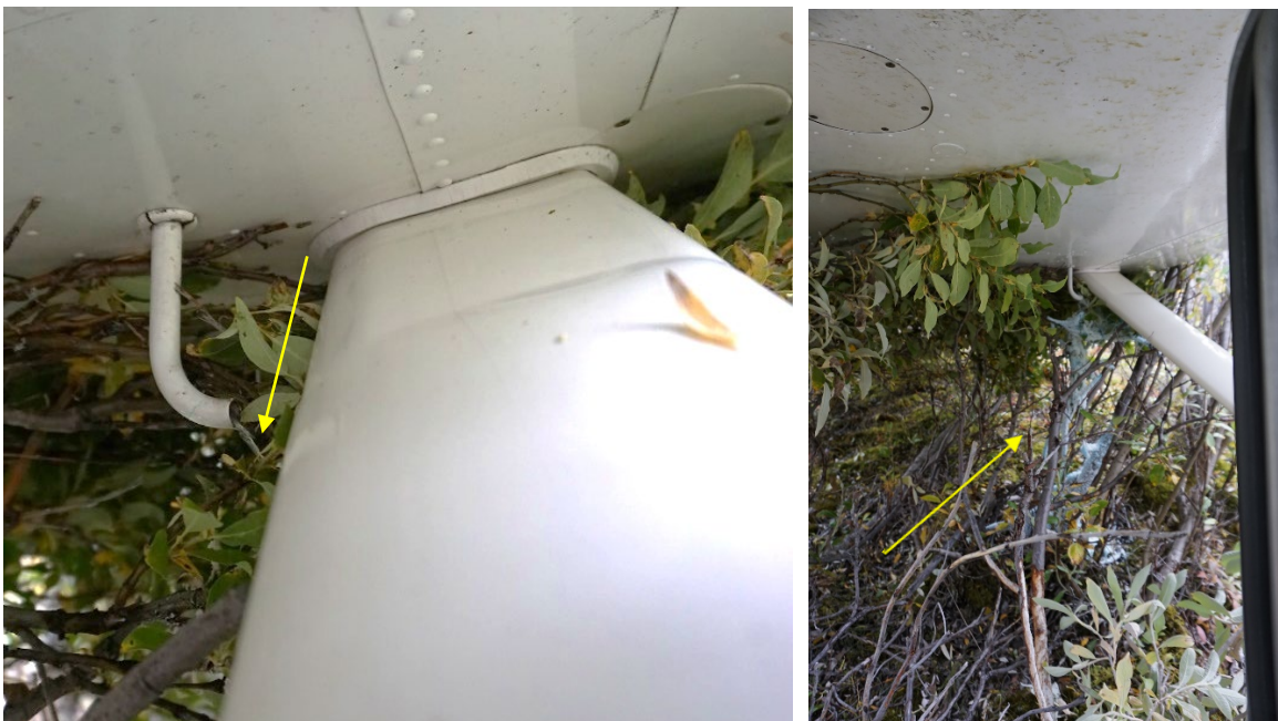
Figure 2. Postaccident left wing fuel leak from vent (source: pilot)
