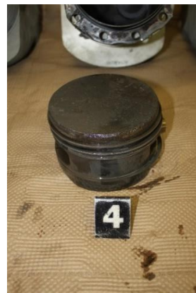
#4 : Mechanical damage, likely #2 cylinder parts that traveled through induction
