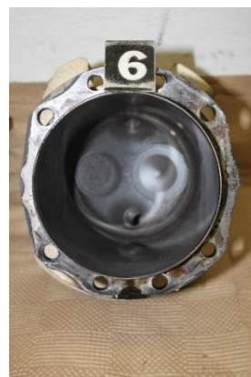
#6 : Light mechanical damage
