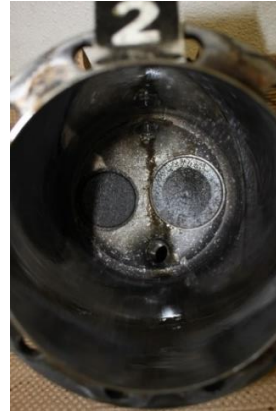
#4 : Mechanical damage around top spark plug bay
