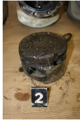
#4 : Mechanical damage, likely #2 cylinder parts that traveled through induction
