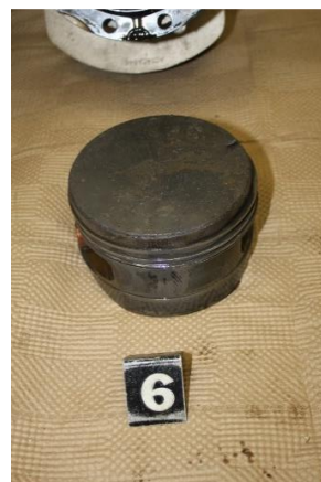
#6 : Mechanical damage, debris on piston, likely pieces from #2 cylinder
