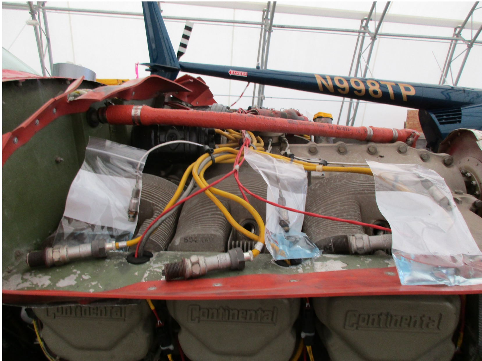
Photo 6 - Sparkplugs and fuel injectors with fuel from fuel lines captured in bags. (Source: FAA)
