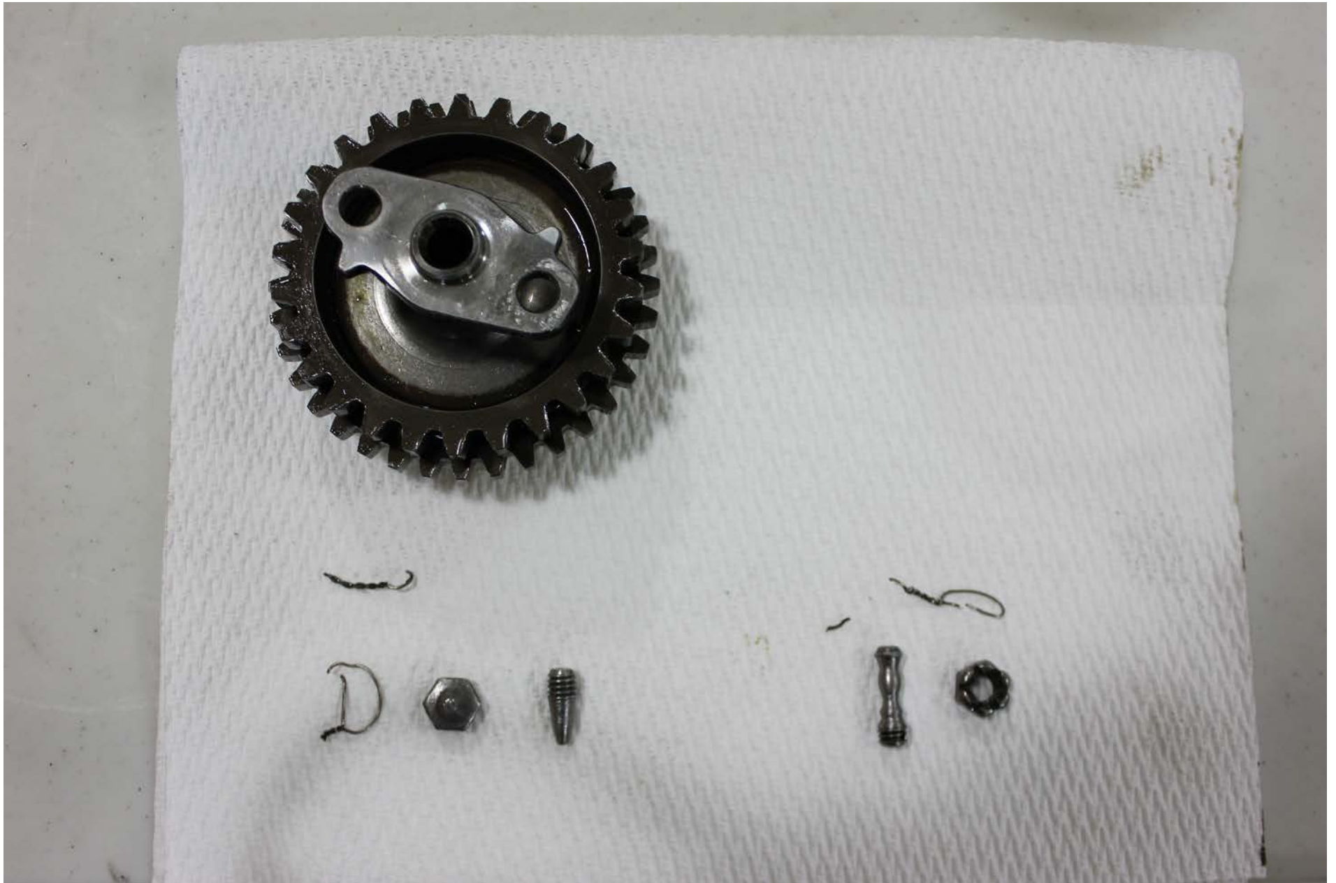
Photo 5 – Image of idler gear, idler gear shaft and flange, mounting bolt pieces, and mounting stud pieces with nut.
