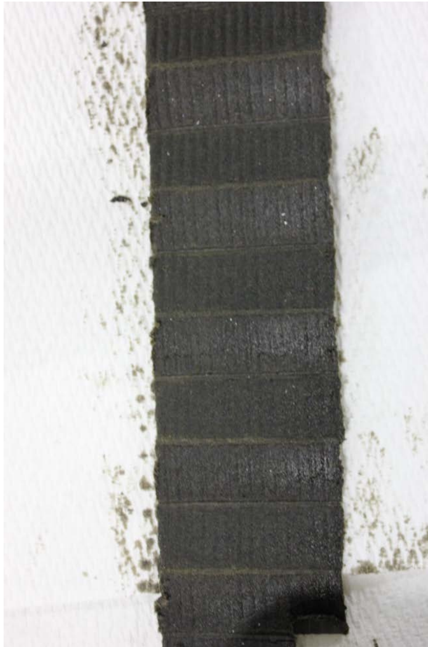
Photo 6 – Oil filter element with shiny flake like metal material from previous 100 hour, 18.1 hours prior to the accident.
