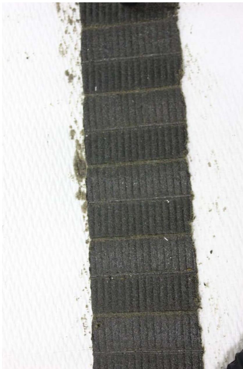
Photo 7 - Oil filter element with shiny flake like metal material from previous 100-hour inspection, with some flakes estimated to be greater than 1/16 of an inch.
