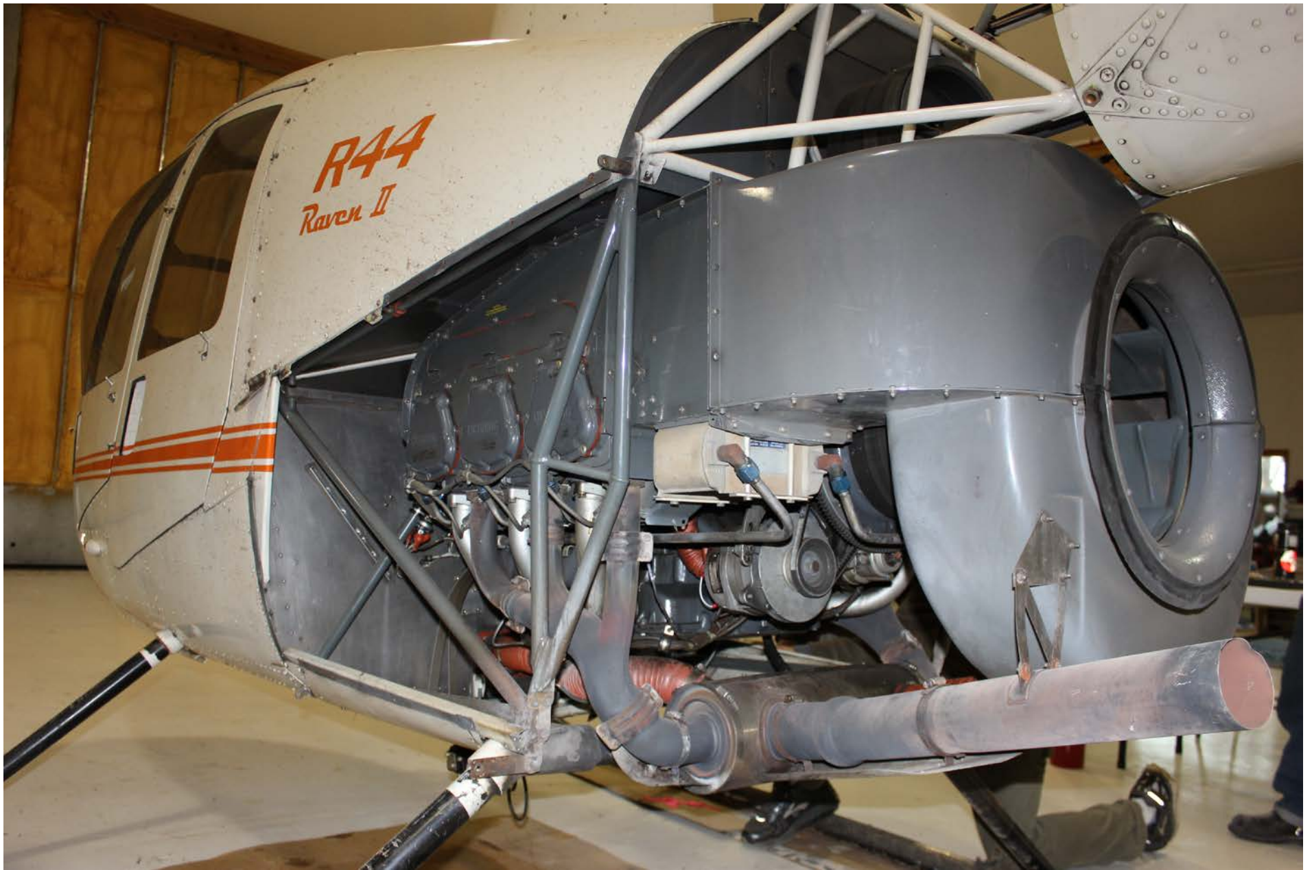
Photo 1 – Accident helicopter after recovery with the engine installed.
