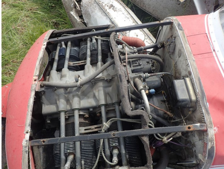
Figure 2. Lycoming O-320 engine at the accident scene with the cowling removed.
