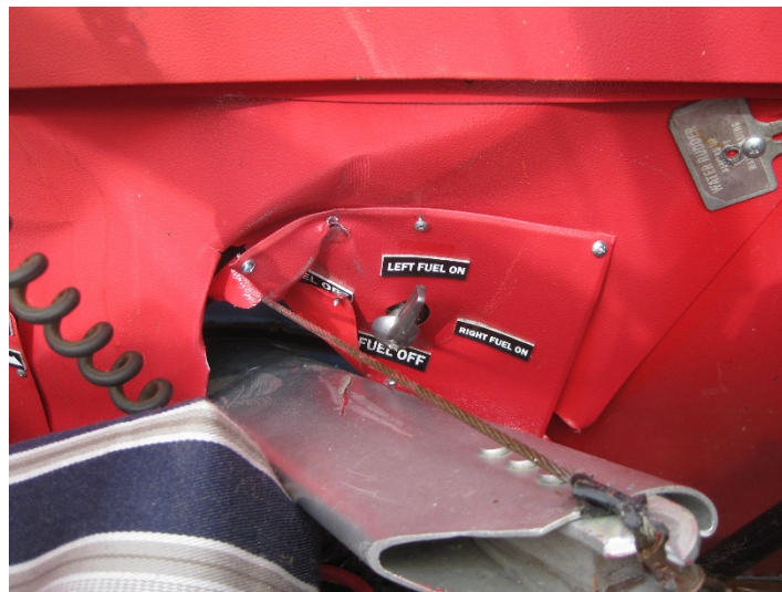
Figure 3. Front cockpit fuel selector in Left Fuel On position and float strut intrusion into the cockpit.
