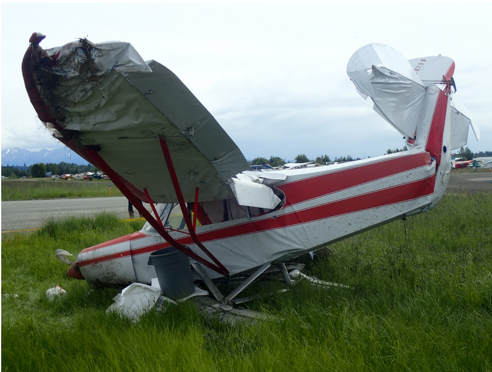
Photo 1 – N7675D Piper PA-18-150 at the accident scene.
