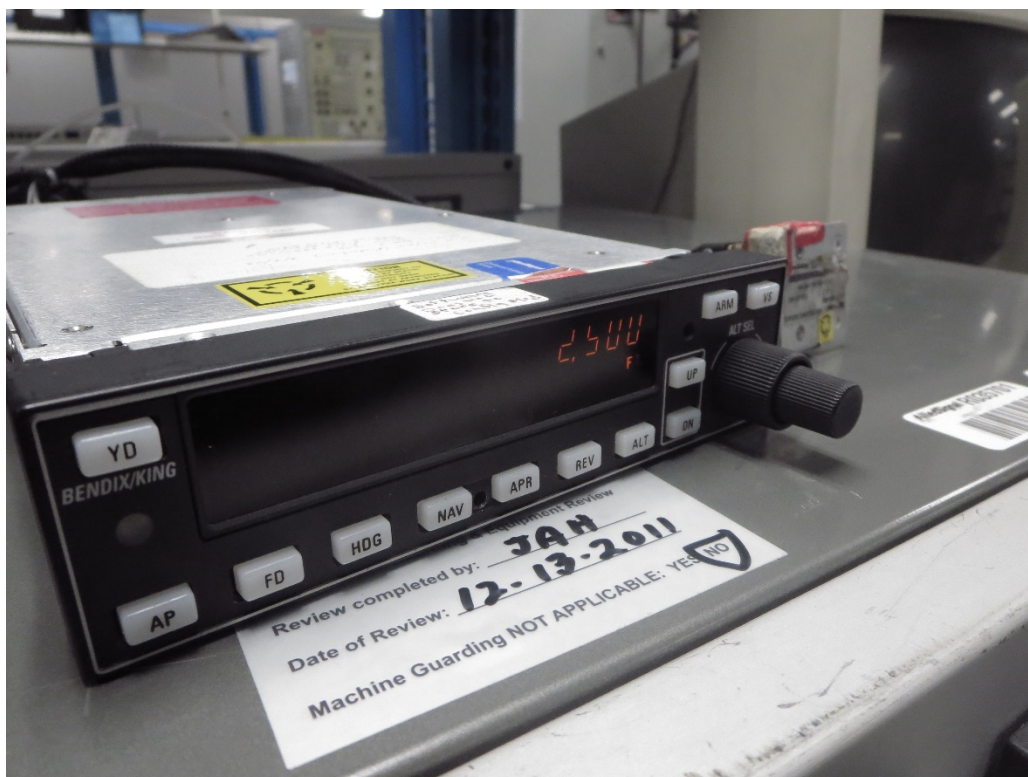
Figure 3 – KC 225 Autopilot Computer with 2,500 altitude value displayed after power was applied.
