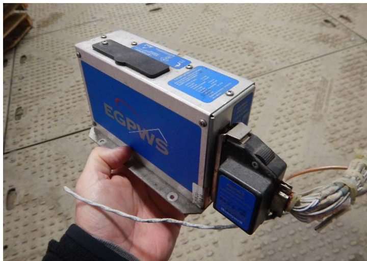
Figure 2 - The airplane's TAWS Unit, as removed.
