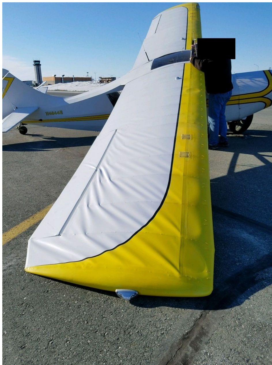
Photo 3 – View of the substantial damage to the right wing and the right aileron (courtesy of the pilot).
