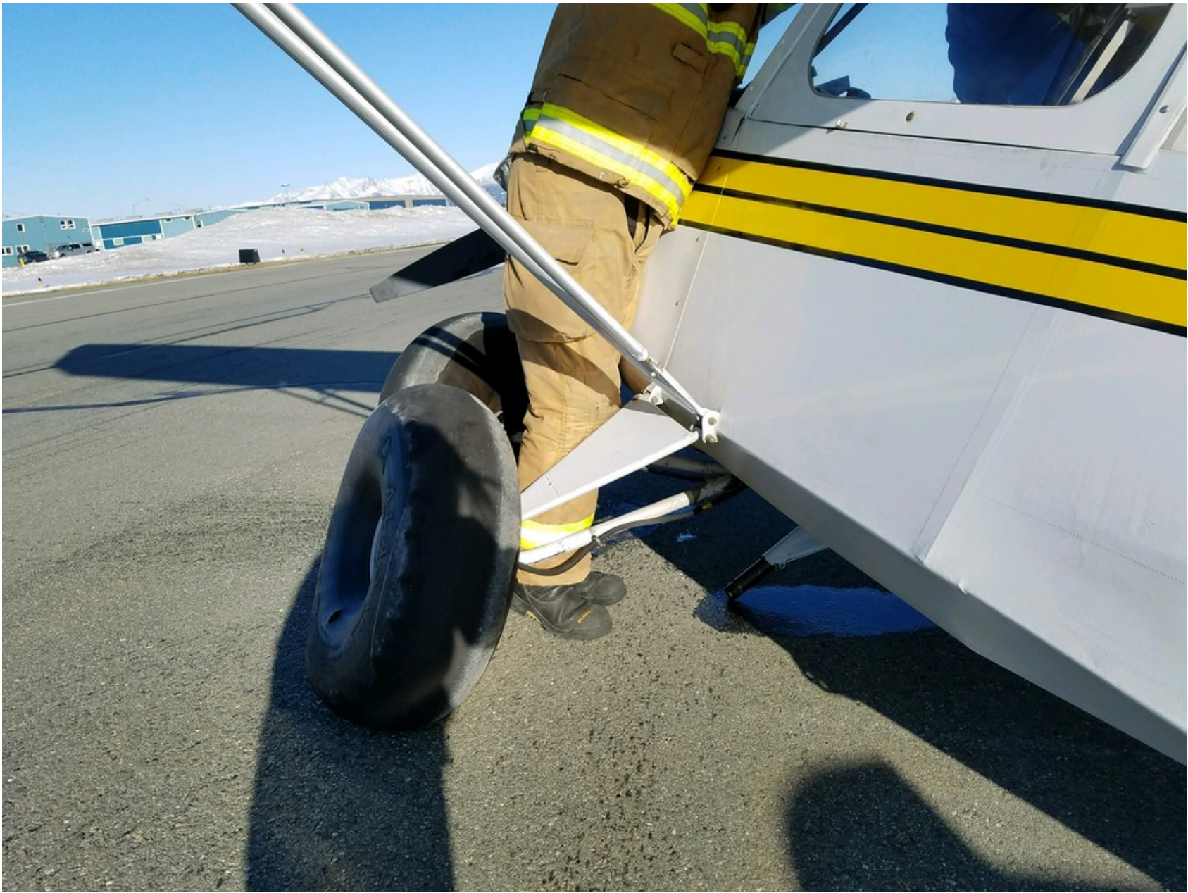
Photo 1 – View of the intact left main landing gear and the separated right main landing gear (courtesy of the pilot).
