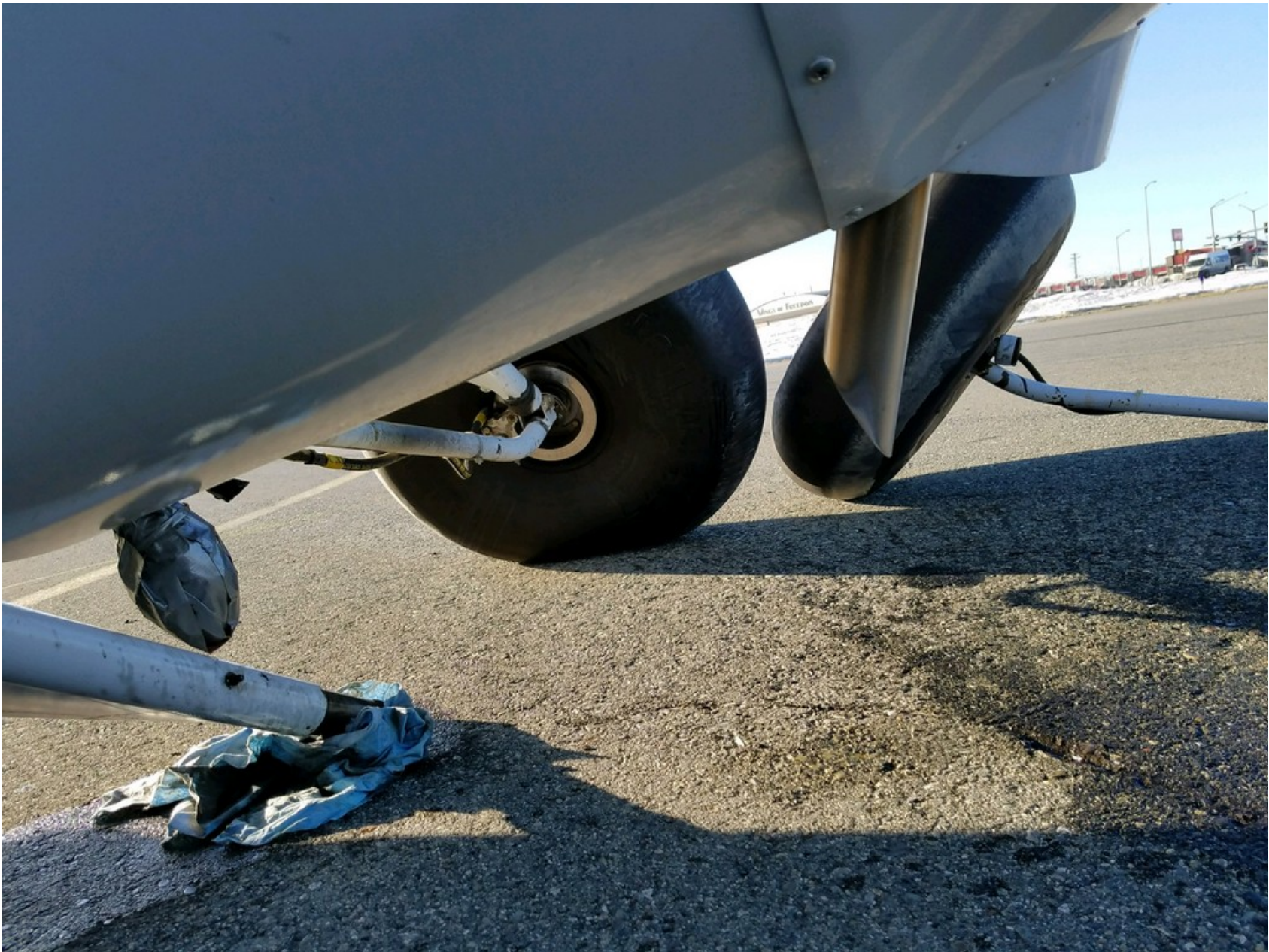
Photo 2 – View of the intact left main landing gear and the separated right main landing gear (courtesy of the pilot).
