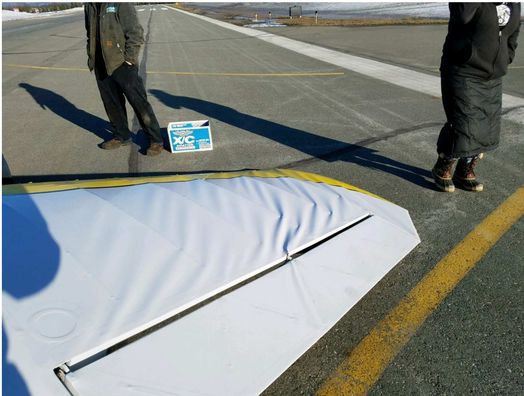
Photo 4 – View of the substantial damage to the right wing and to the right aileron (courtesy of the pilot).
