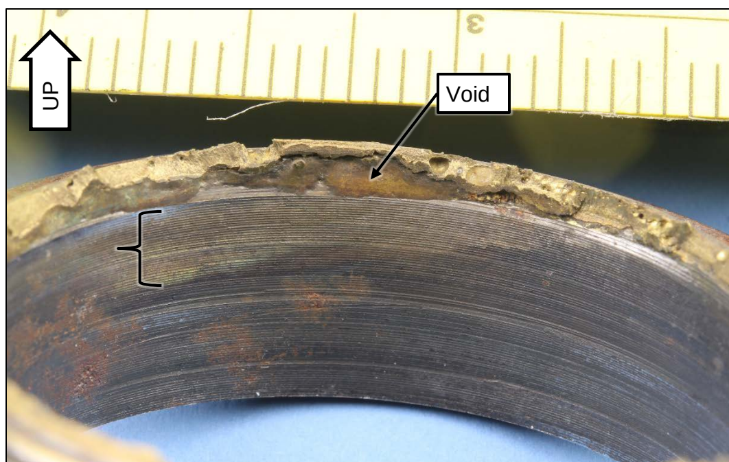
Figure 5. Interior face of the sleeve showing a void across most of the fillet radius. An unlabeled bracket indicates a gold-colored surface appearance adjacent to the braze fillet.
