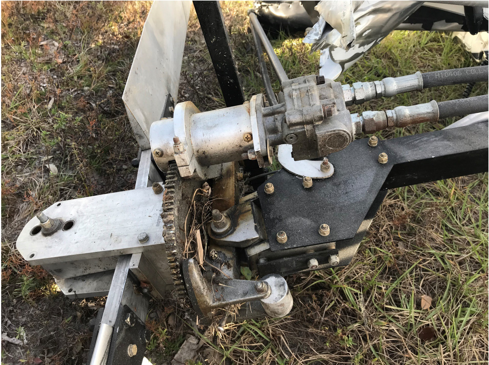
Photo 7 - Close image of rotor system and prerotator. (Source: FAA)
