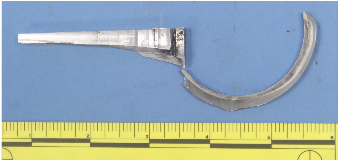
Figure 16 – The fracture surfaces of the circumferential fatigue and overstress fracture and the longitudinal fracture, after disassembly, sectioning, and cleaning.
