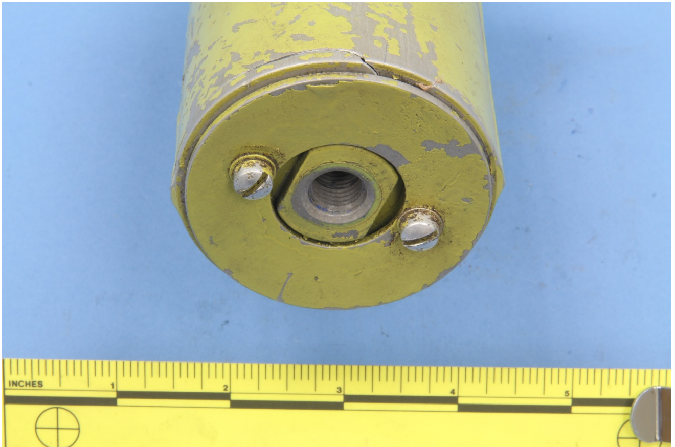
Figure 3 – The end of the hydraulic actuator, showing the circumferential portion of the crack.
