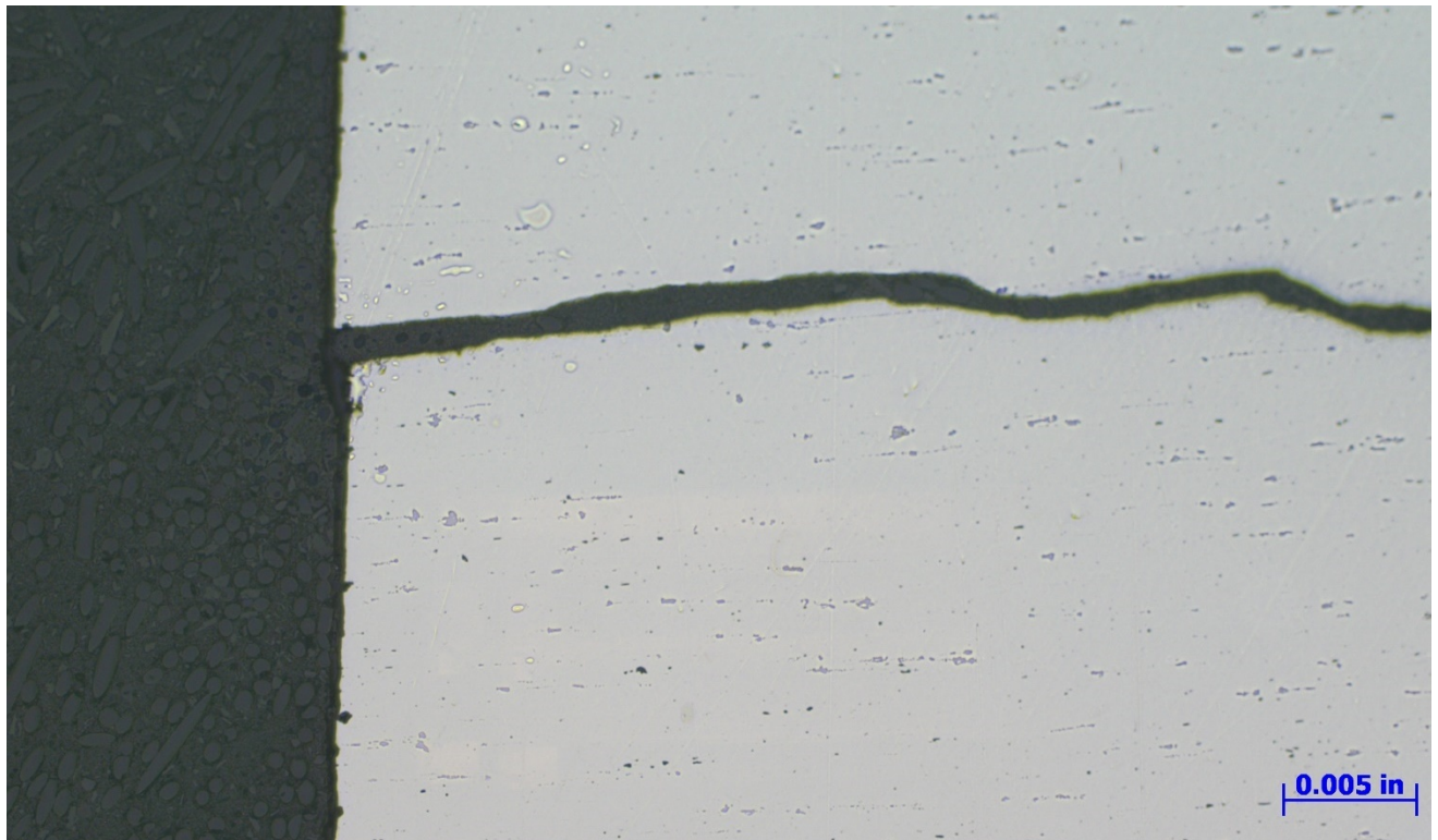
Figure 19 – BF optical metallograph showing a closer view of the right crack from Figure 16 (~100X, as polished).
