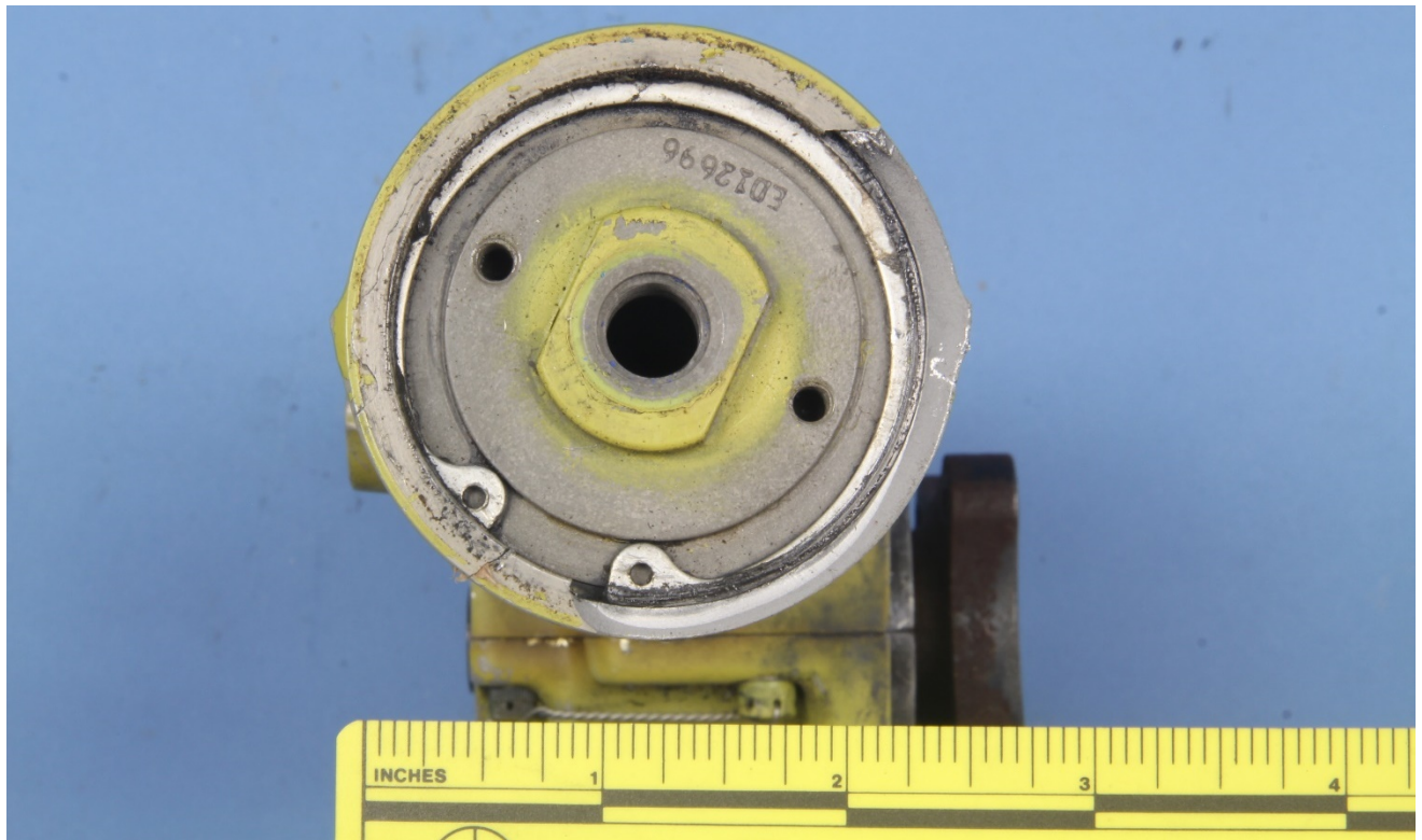
Figure 6 – The fractured end of the actuator, after disassembly. The retaining ring was still in place in the groove.
