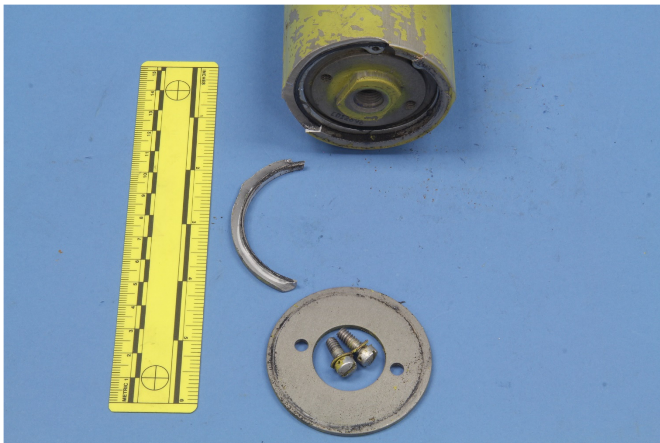
Figure 5 – The cracked end of the actuator pictured in Figure 3, after removal of the screws and the end cap.
