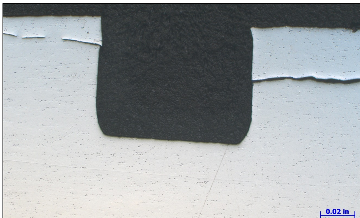
Figure 18 – Bright-field (BF) optical metallograph cross-section of the actuator retaining ring showing a horizontal crack through the groove (~25X, as polished).
