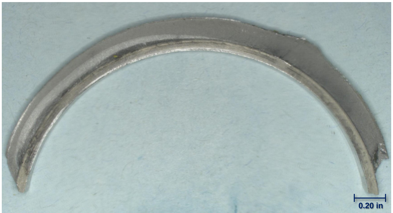
Figure 7 – Montage of magnified images of the crack face of the circumferential crack, showing indications of progressive cracking.
