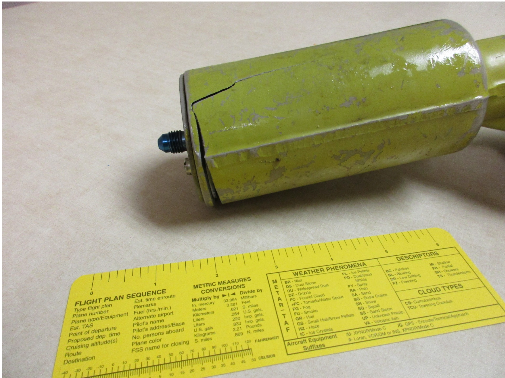
Photo 4 - Landing gear actuator exhibiting circumferential fracture.
