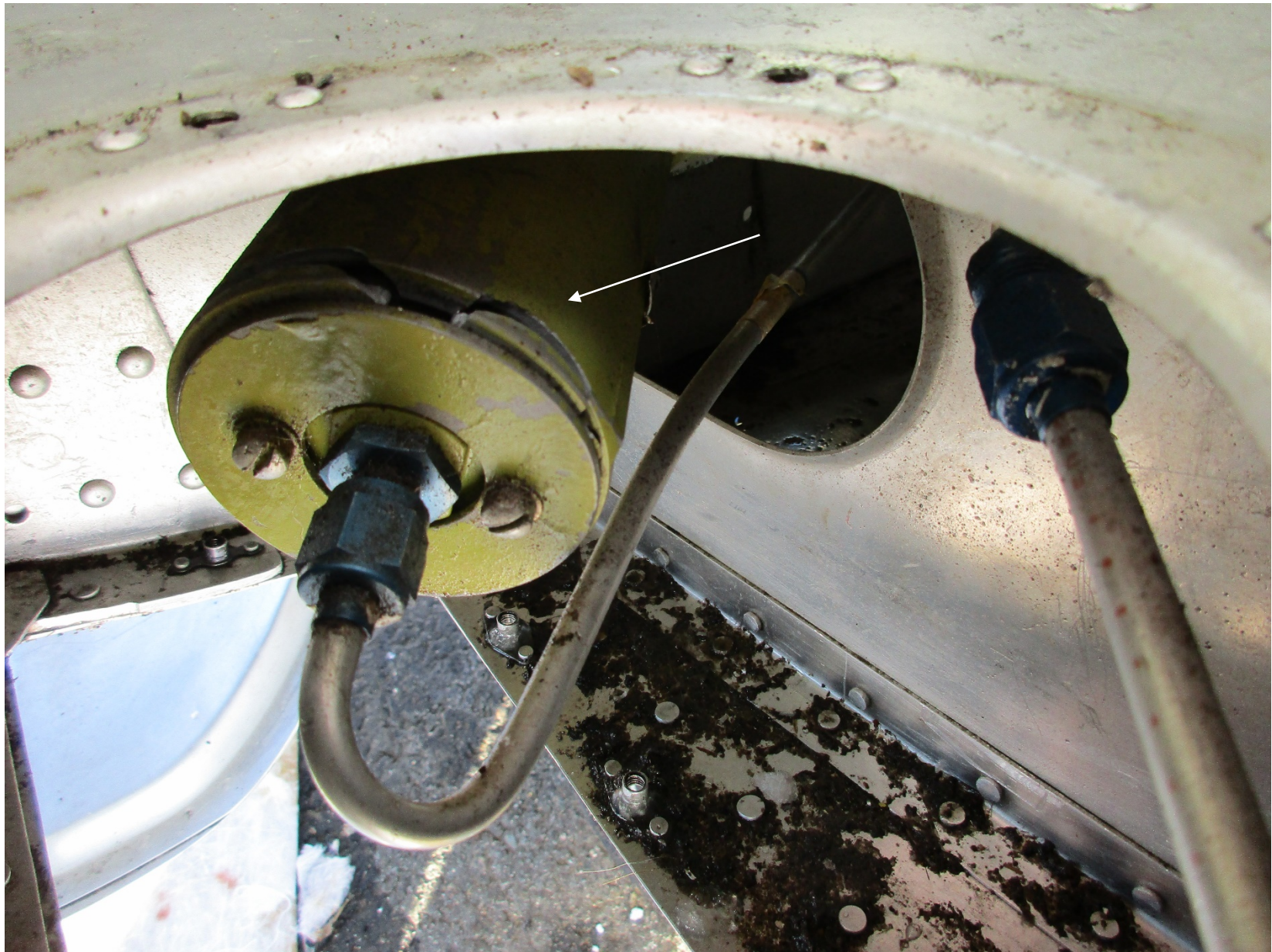
Photo 3 - Landing gear actuator exhibiting fractures. (Source: Federal Aviation Administration)
