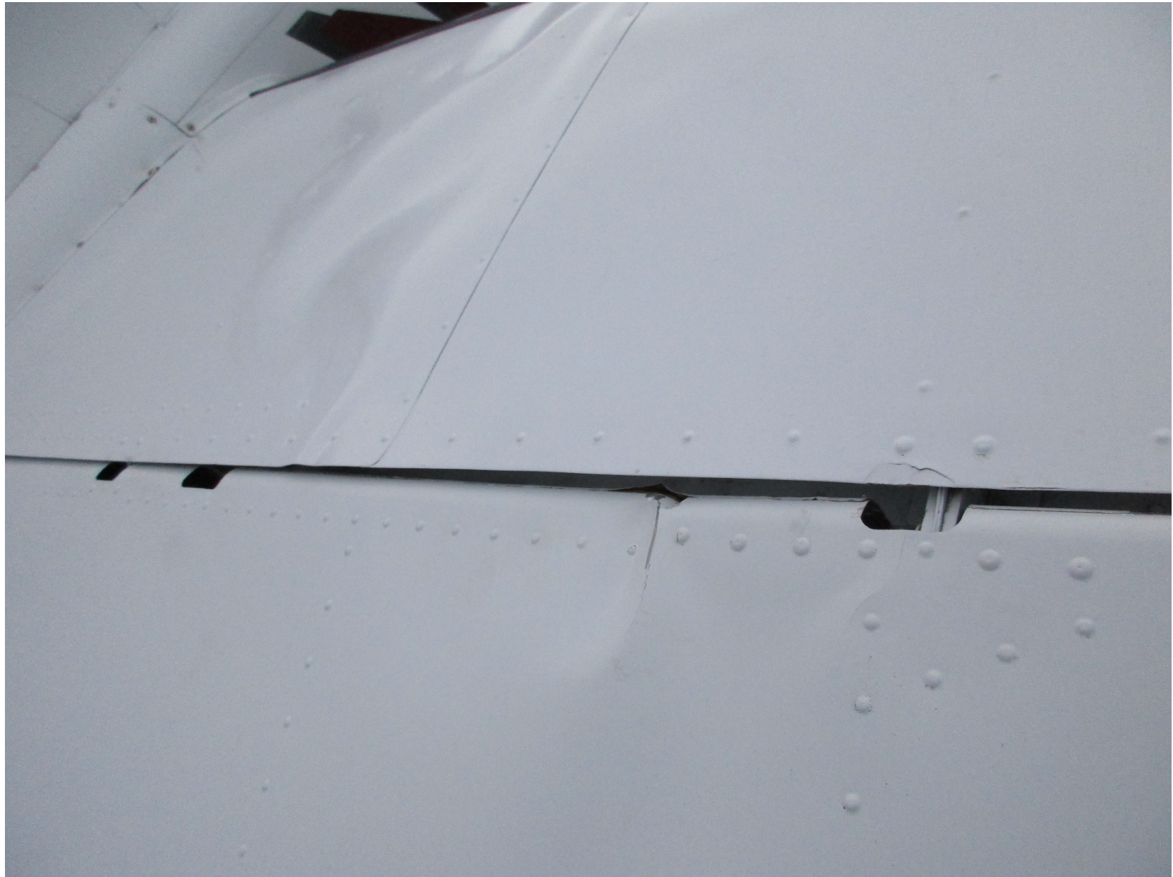
Photo 2 - Right wing and aileron substantial damage. (Source: Federal Aviation Administration)
