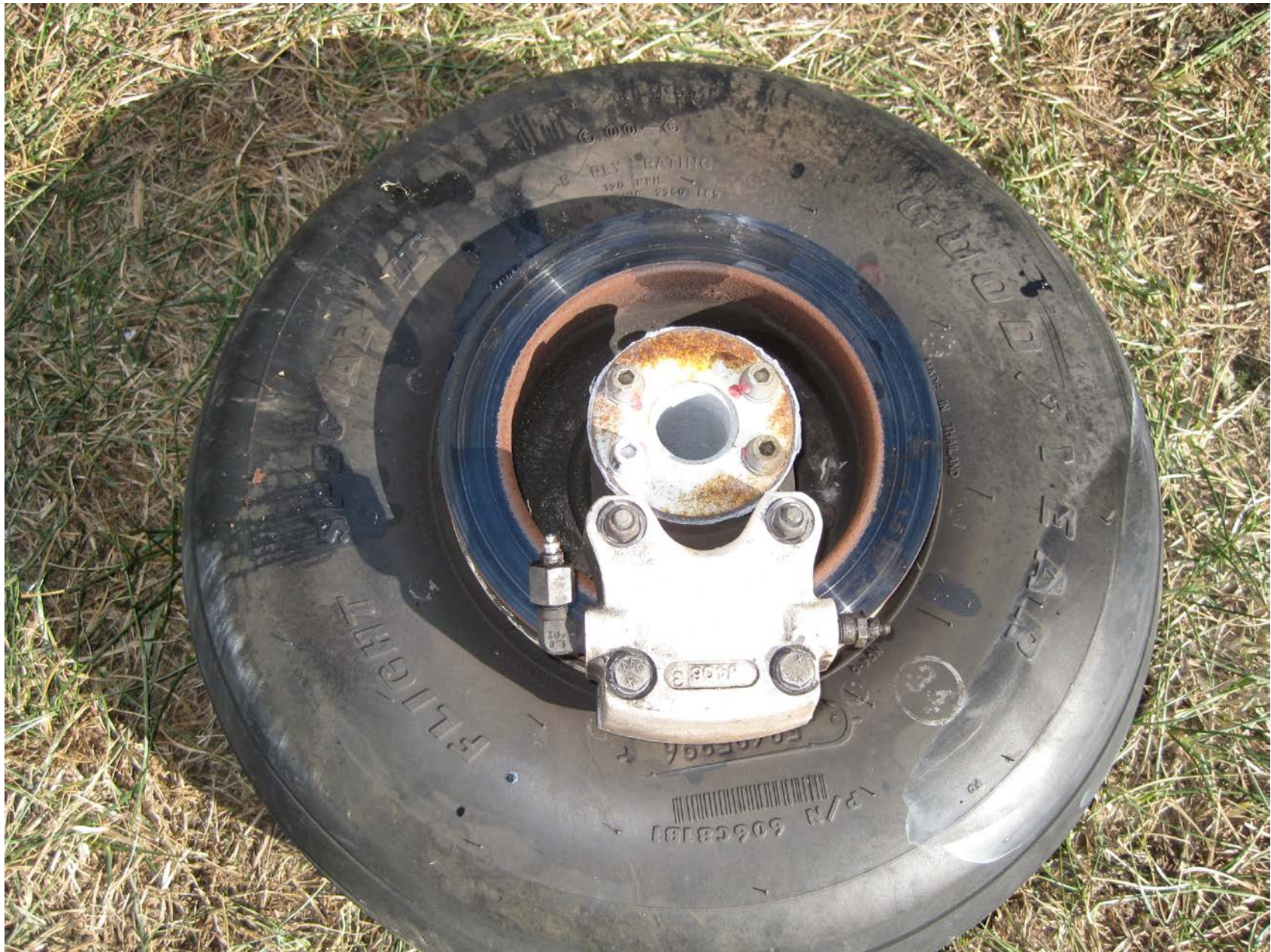
Photo 3 – View of the tire from the fractured left main landing gear assembly (courtesy of the FAA).
