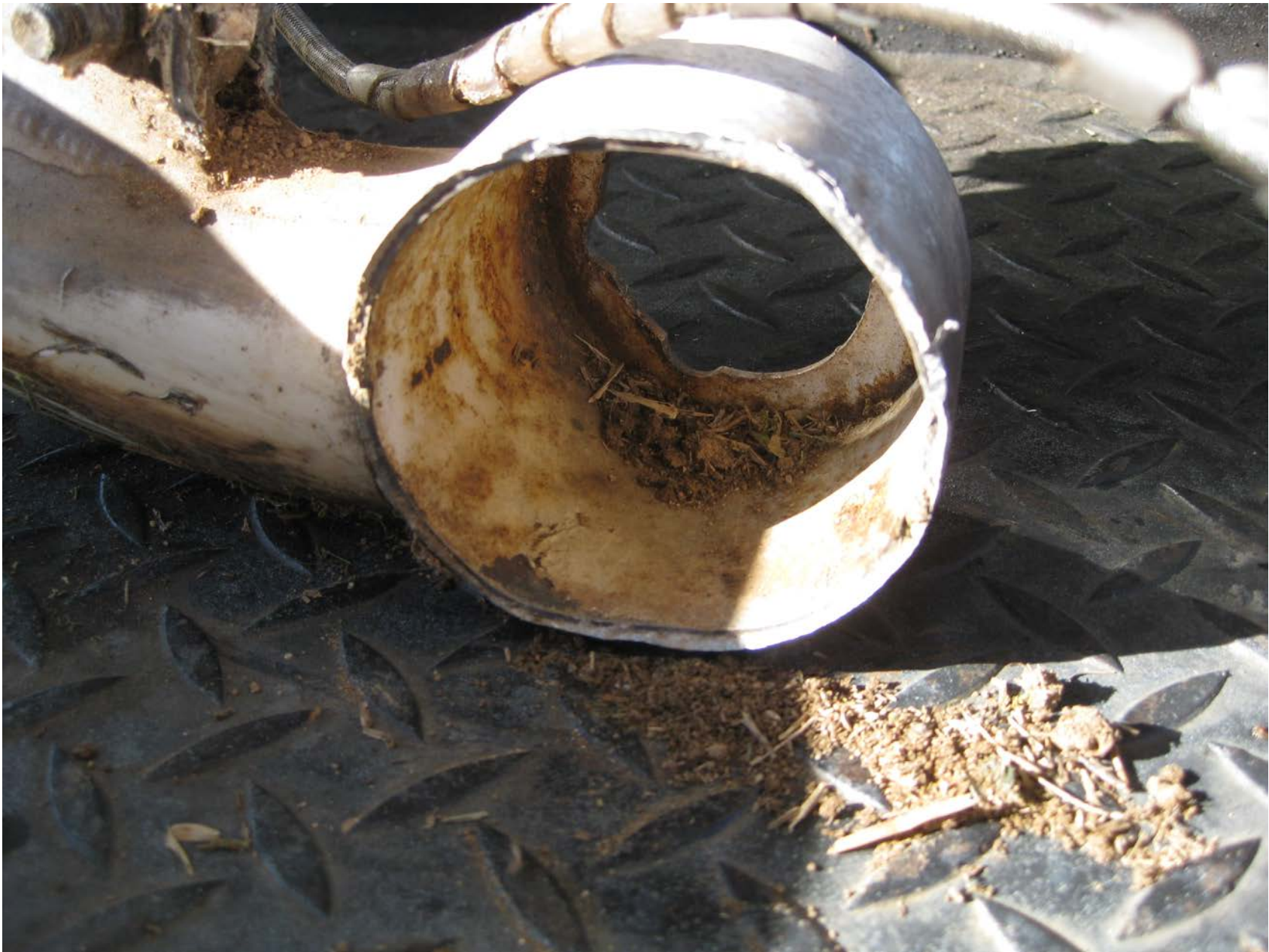
Photo 2 – View of the fractured left main landing gear assembly (courtesy of the FAA).
