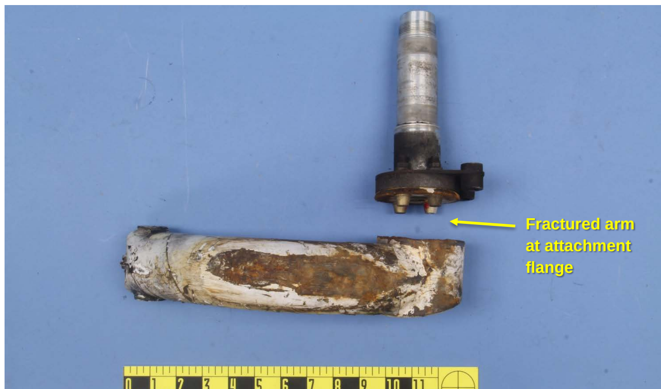
Figure 2 – The halves of the left assembly, positioned such that the fracture surfaces mate.
