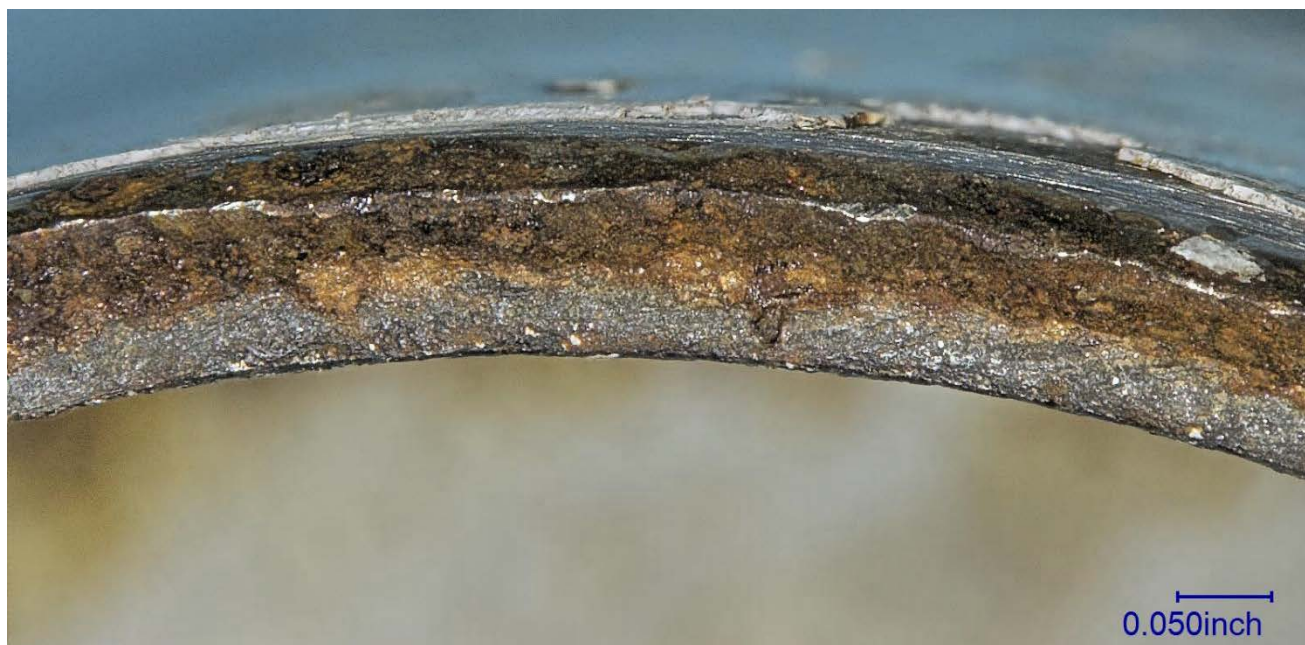
Figure 8 – A portion of the arm side fracture surface, after cleaning with acetone.
