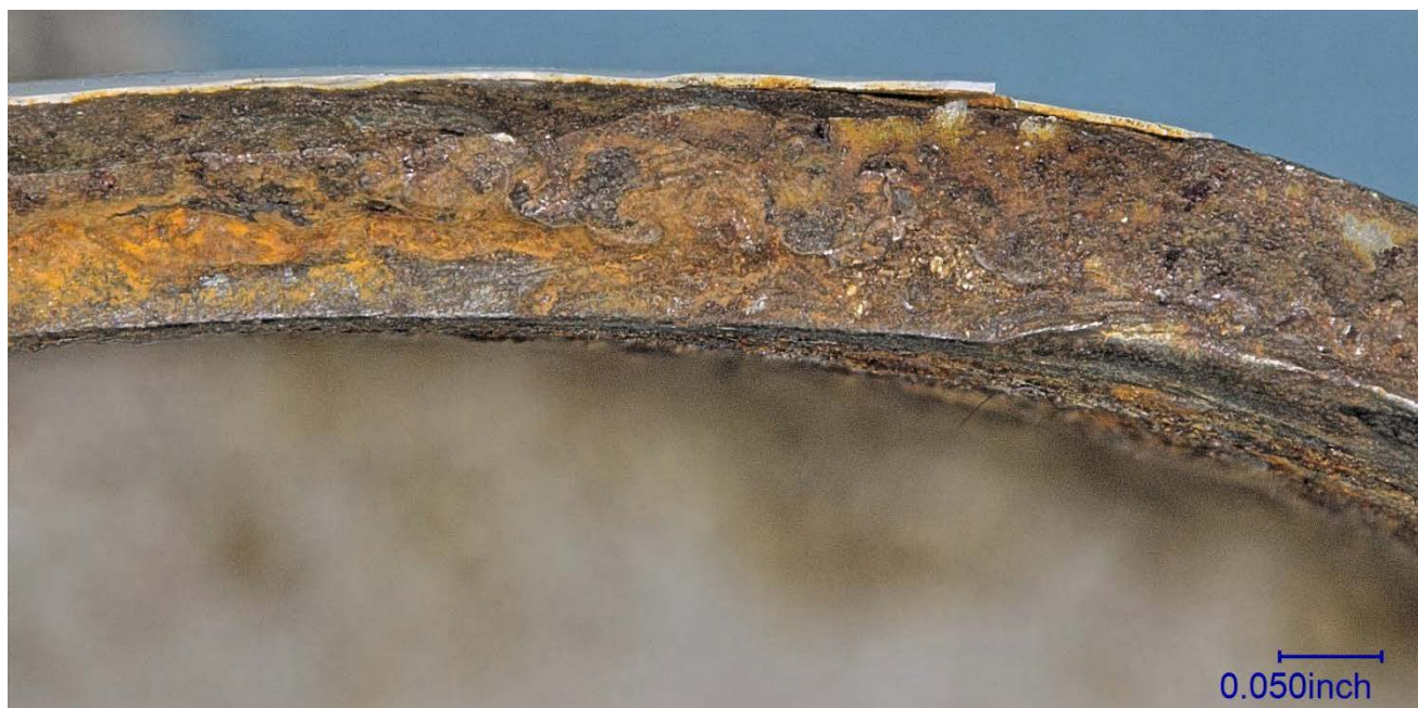
Figure 7 – A portion of the arm side fracture surface, prior to cleaning with acetone.
