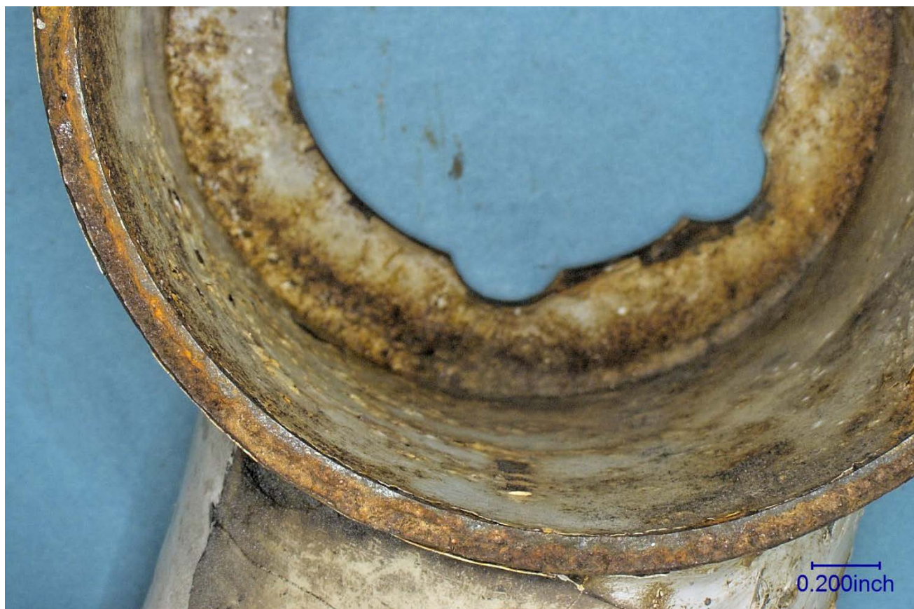
Figure 5 – Closer view of the fracture surface from the arm side.
