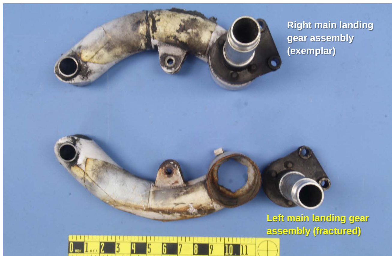
Figure 1 – The landing gear assembly components, as received.
