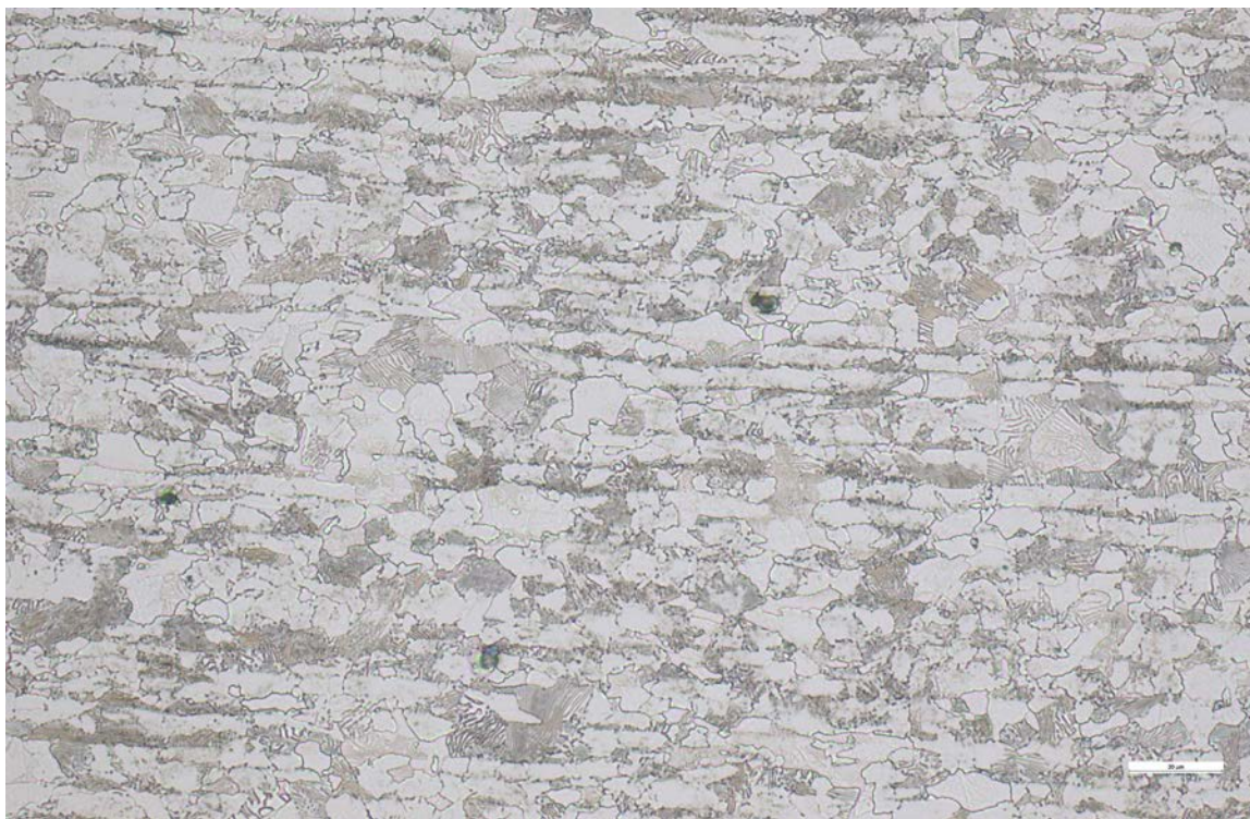
Figure 17 – BF micrograph showing a typical area of the arm flange microstructure (~200X, etched 2% Nital).
