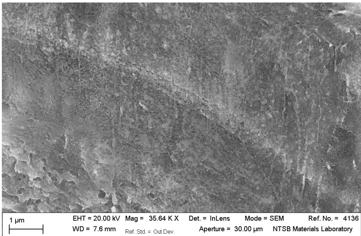
Figure 14 – SE micrograph showing a closer view of the fatigue striations in Figure 13.
