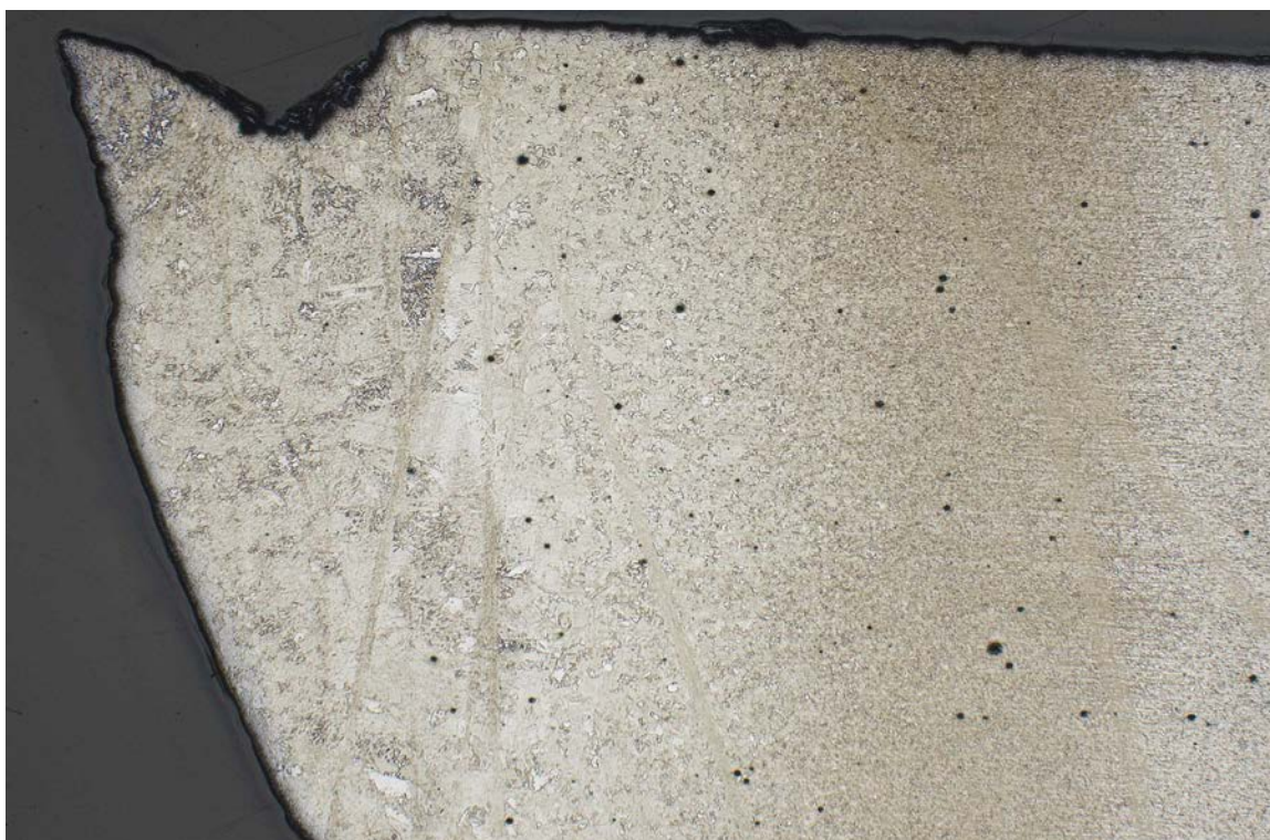
Figure 15 – Bright-field (BF) micrograph of a cross section through the fracture surface on the flange side weld (upper left) (~25X, etched 2% Nital).
