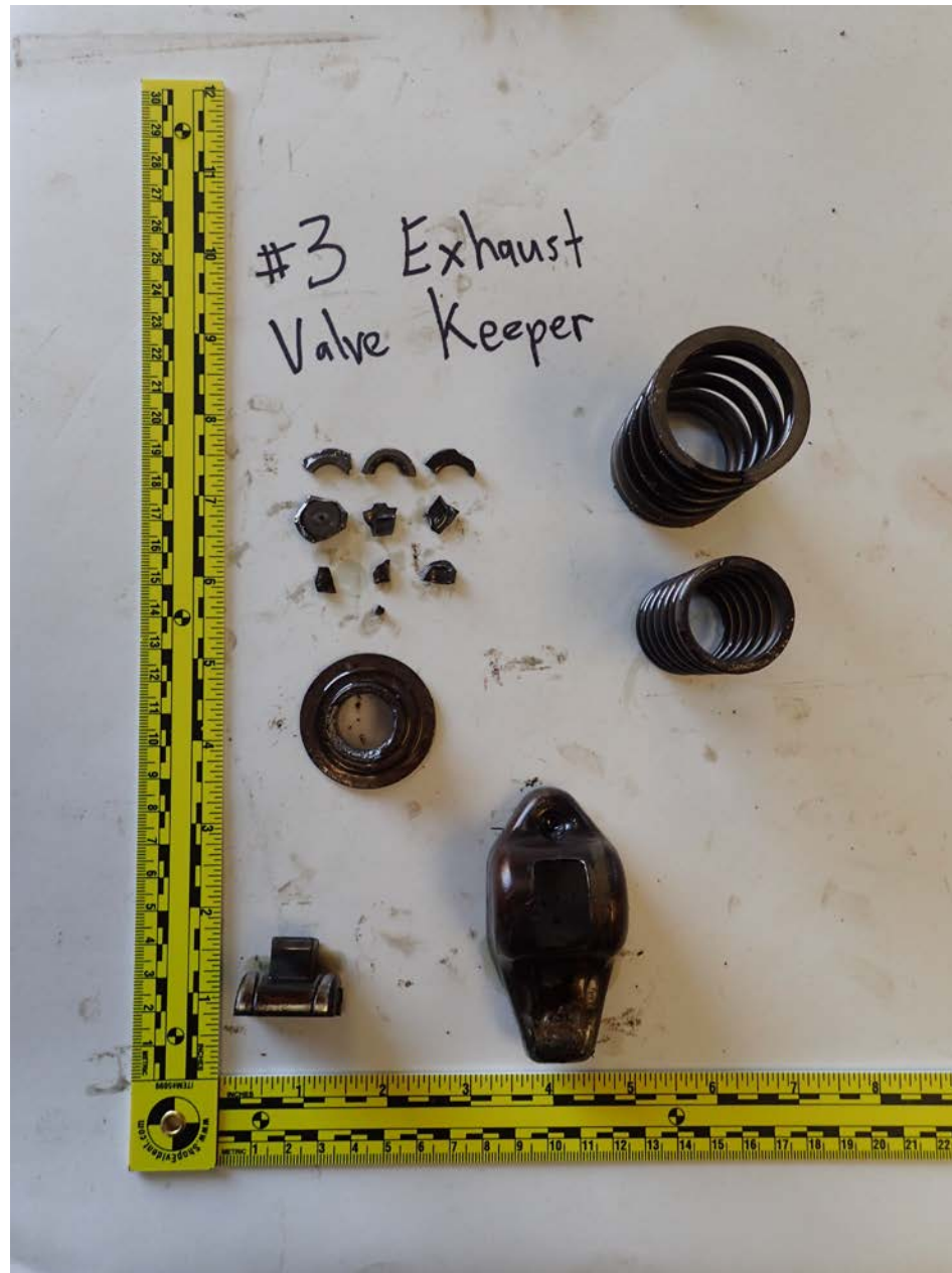
Photo 9 – View of the fractured valve key (exhaust), fractured valve stem cap (exhaust), and damaged valve spring seat (upper exhaust).
