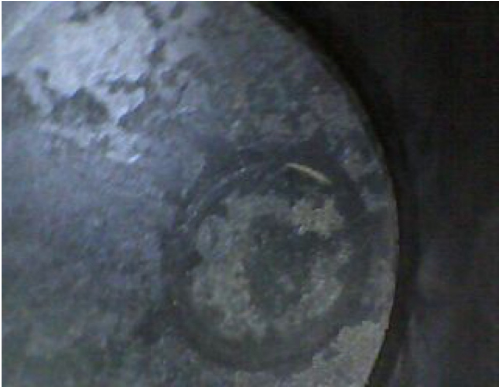
Photo 5 – Borescope image of the number 3 piston impact marks from the exhaust valve.
