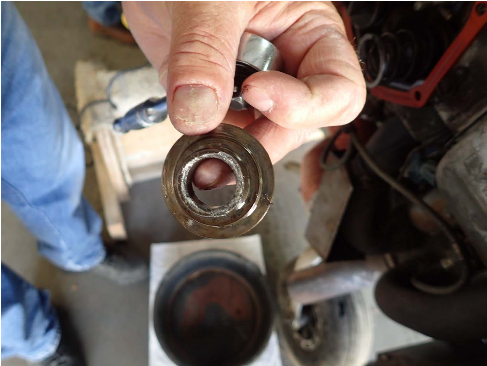
Photo 7 – View of the damaged number 3 valve spring seat (upper exhaust).
