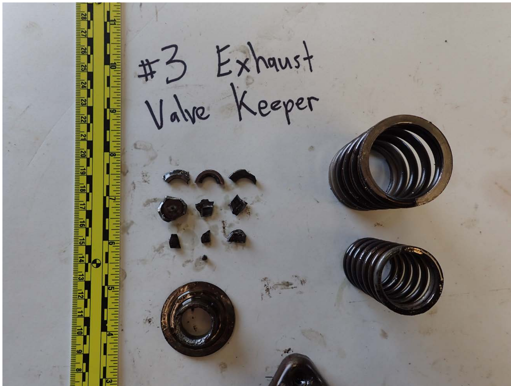
Photo 10 – View of the fractured valve key (exhaust), fractured valve stem cap (exhaust), and damaged valve spring seat (upper exhaust).
