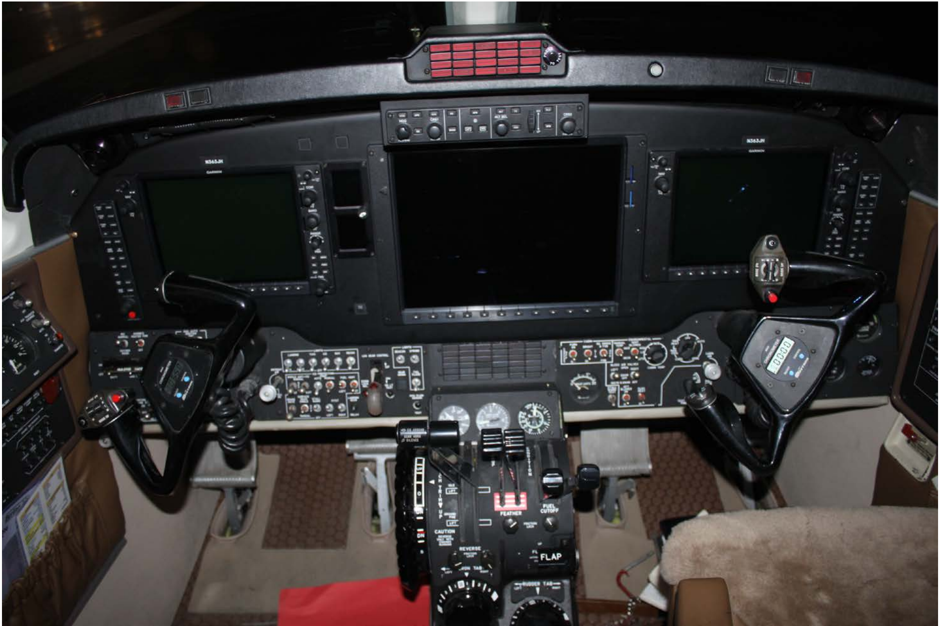
Photo 3 – View of the Garmin G1000 avionics suite.
