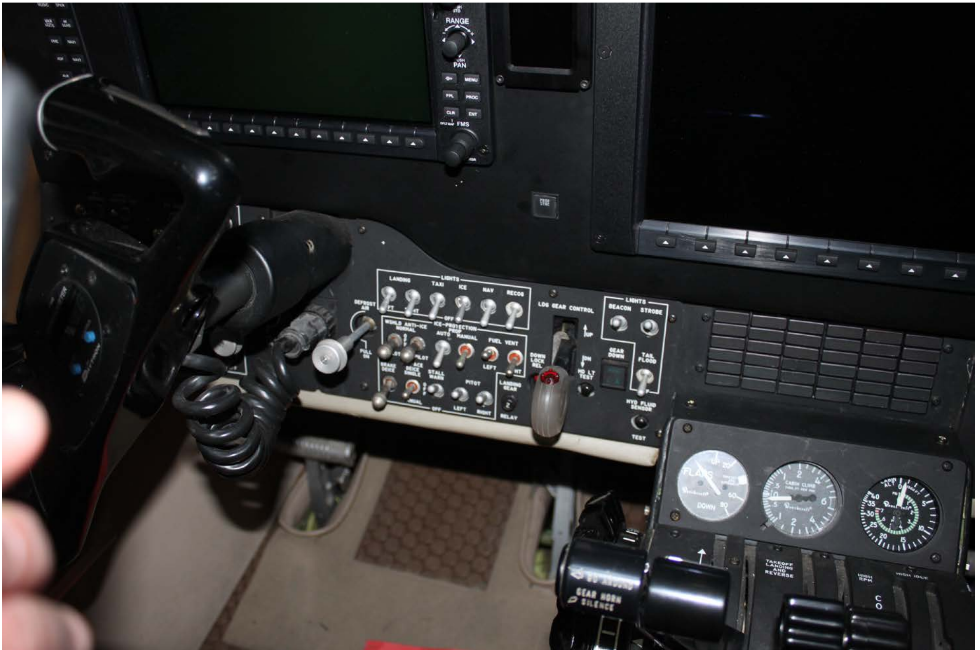
Photo 5 – View of the landing gear selector.
