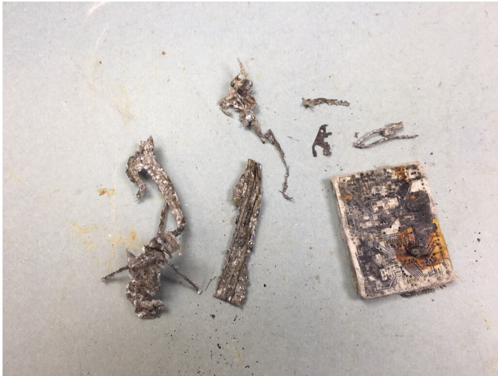
Figure 1. Burned components received from Garmin Aera device.
