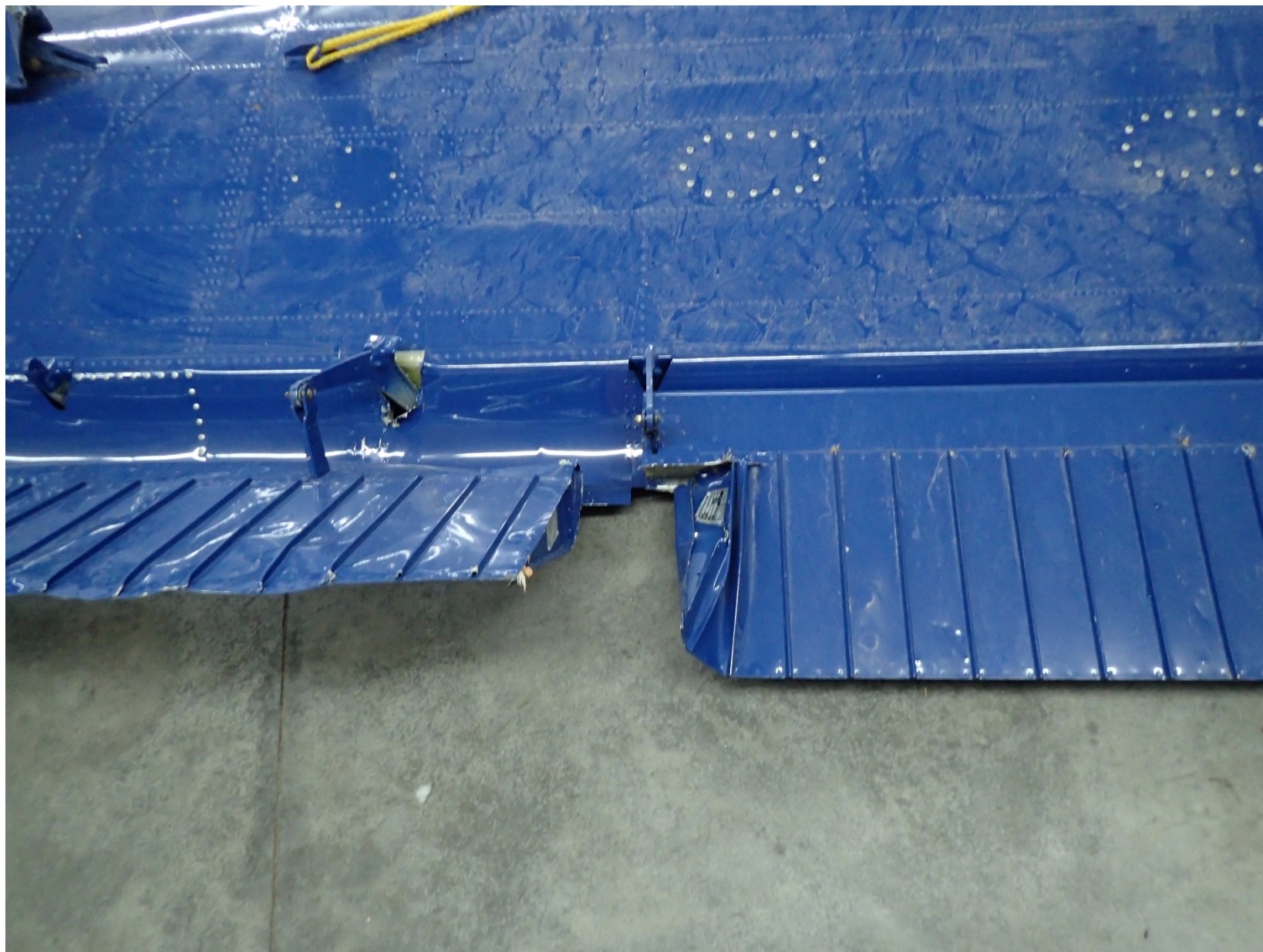
Photo 10 - Left flap and aileron indicating impact deformation.
