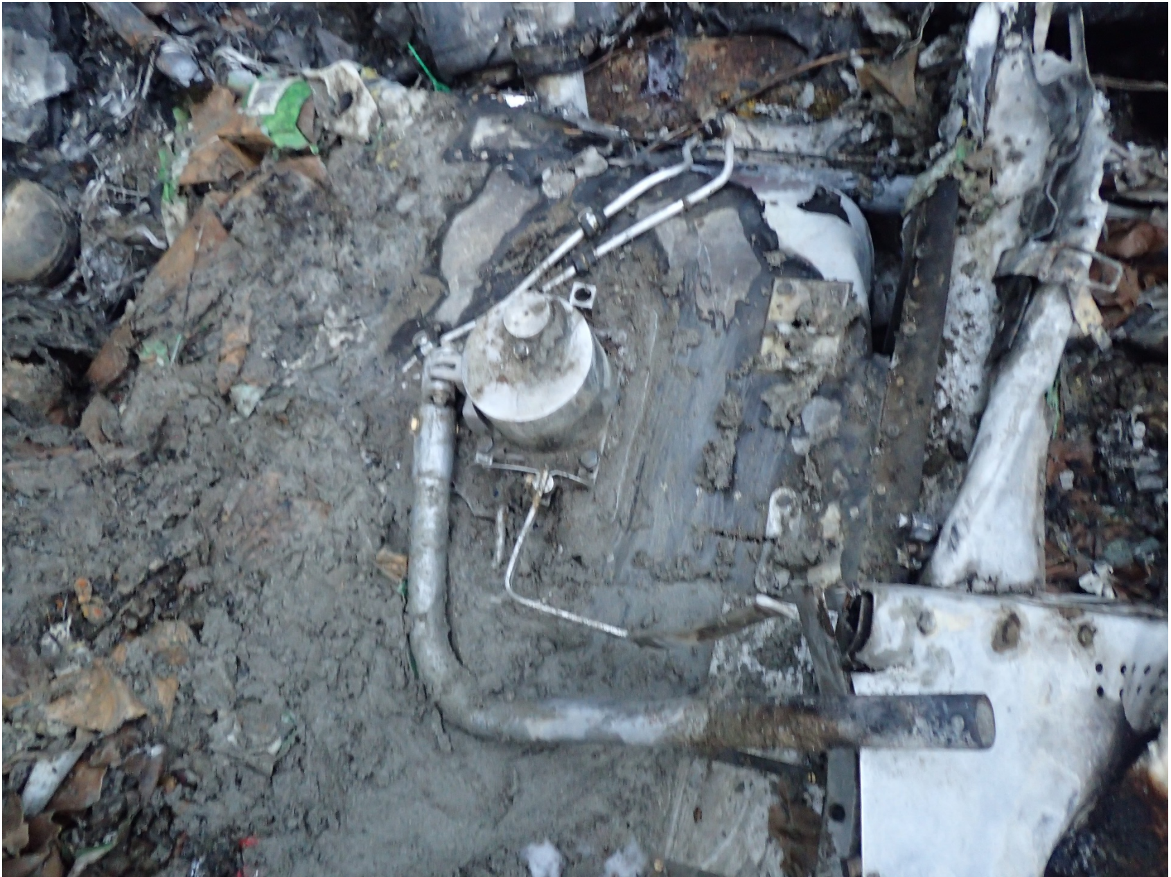
Photo 8 - Hydraulic reservoir and flap pump and flap selector indicating down positions.
