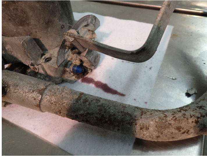
Figure 2. Hydraulic flap pump exhibiting positive flow.
