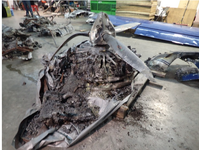
Figure 3. Pratt and Whitney R-985 engine and propeller exhibiting mechanical and thermal damage.
