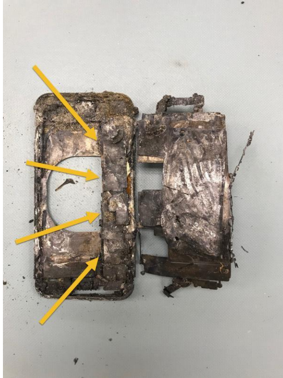
Figure 2. The device during internal examination. The region occupied by the main board is indicated by yellow arrows.
