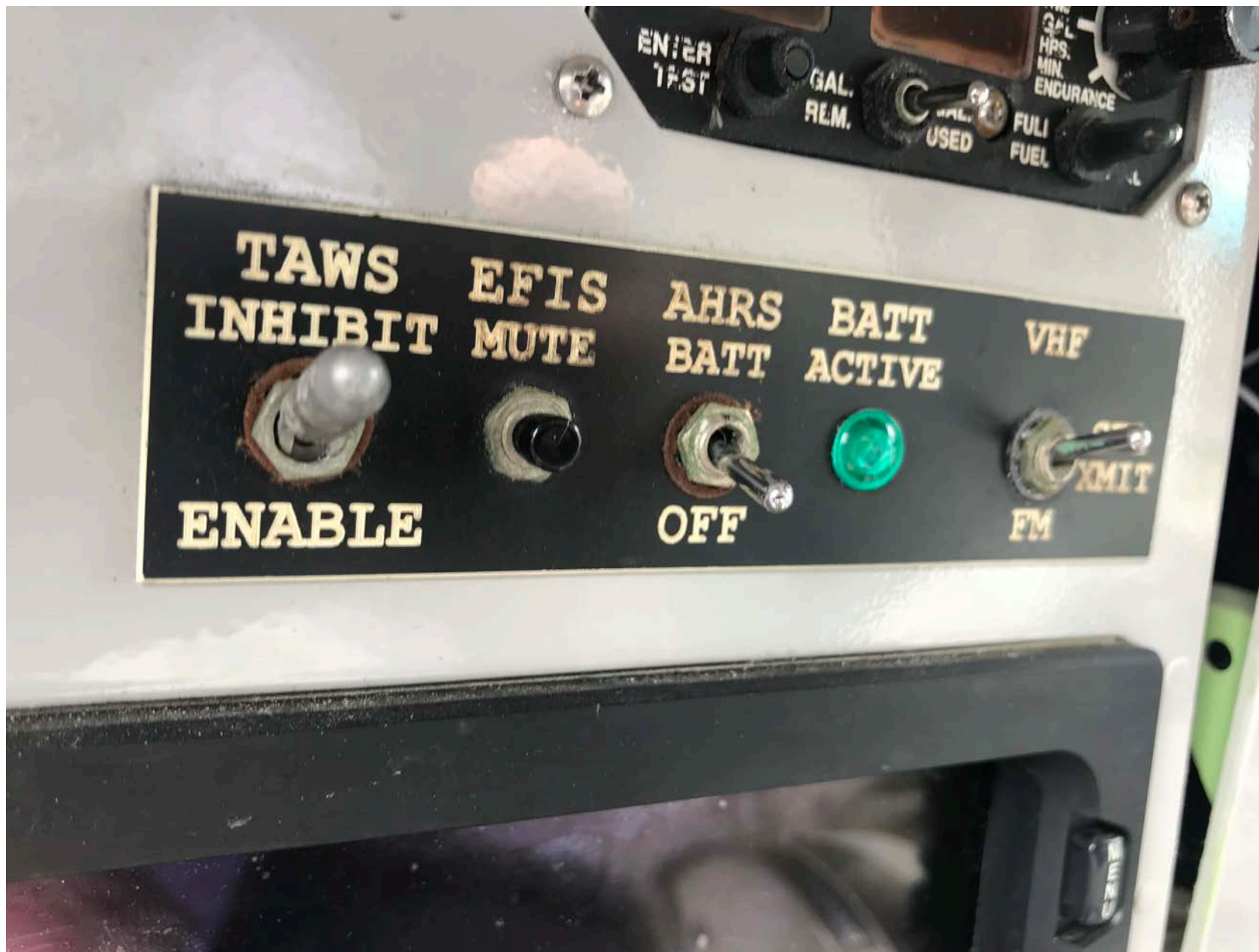
Photo 4 – TAWS inhibit switch in accident airplane in the inhibit mode.
