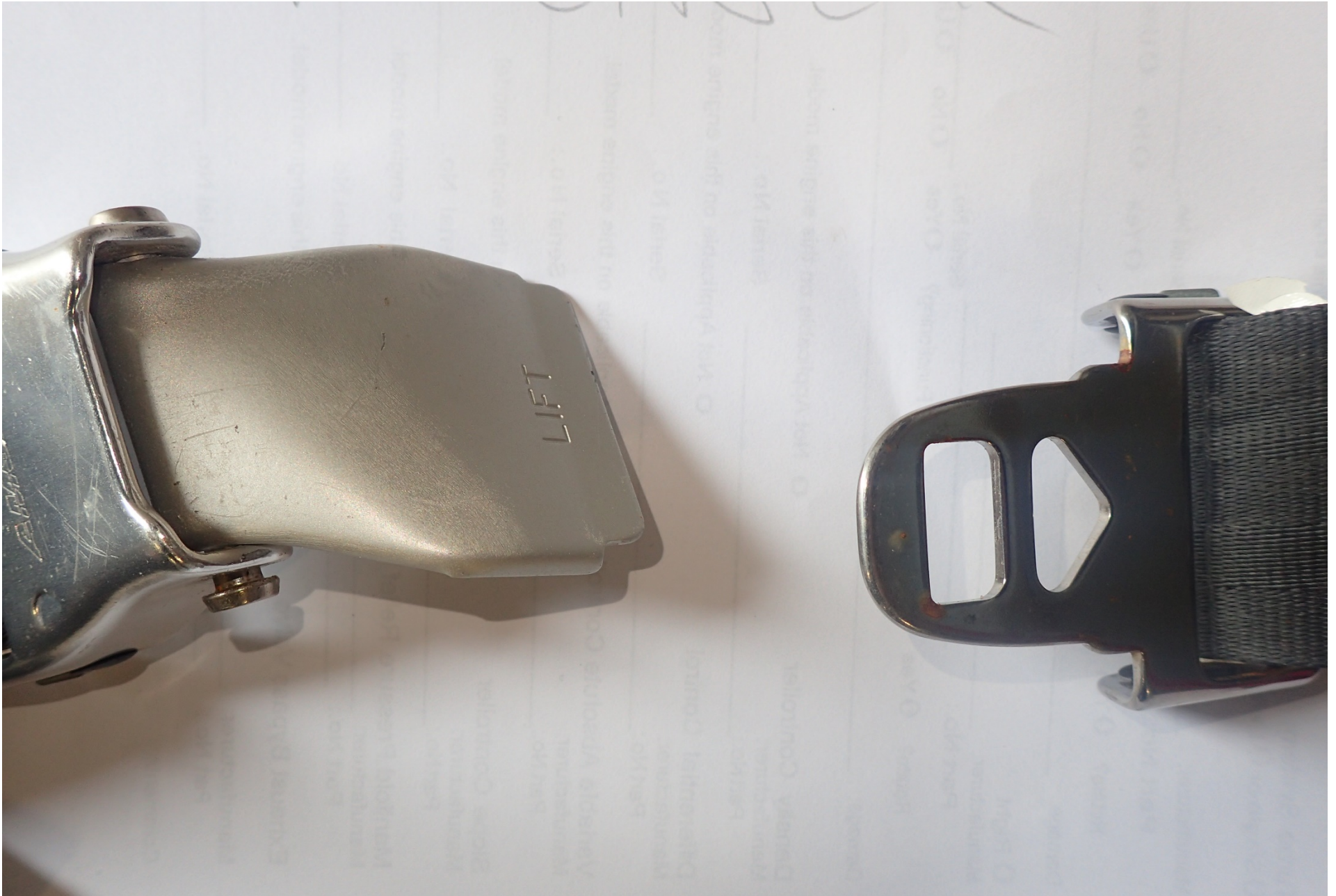
Photo 7 - Rear seat (passenger's) lap belt buckle exhibiting deformation.
