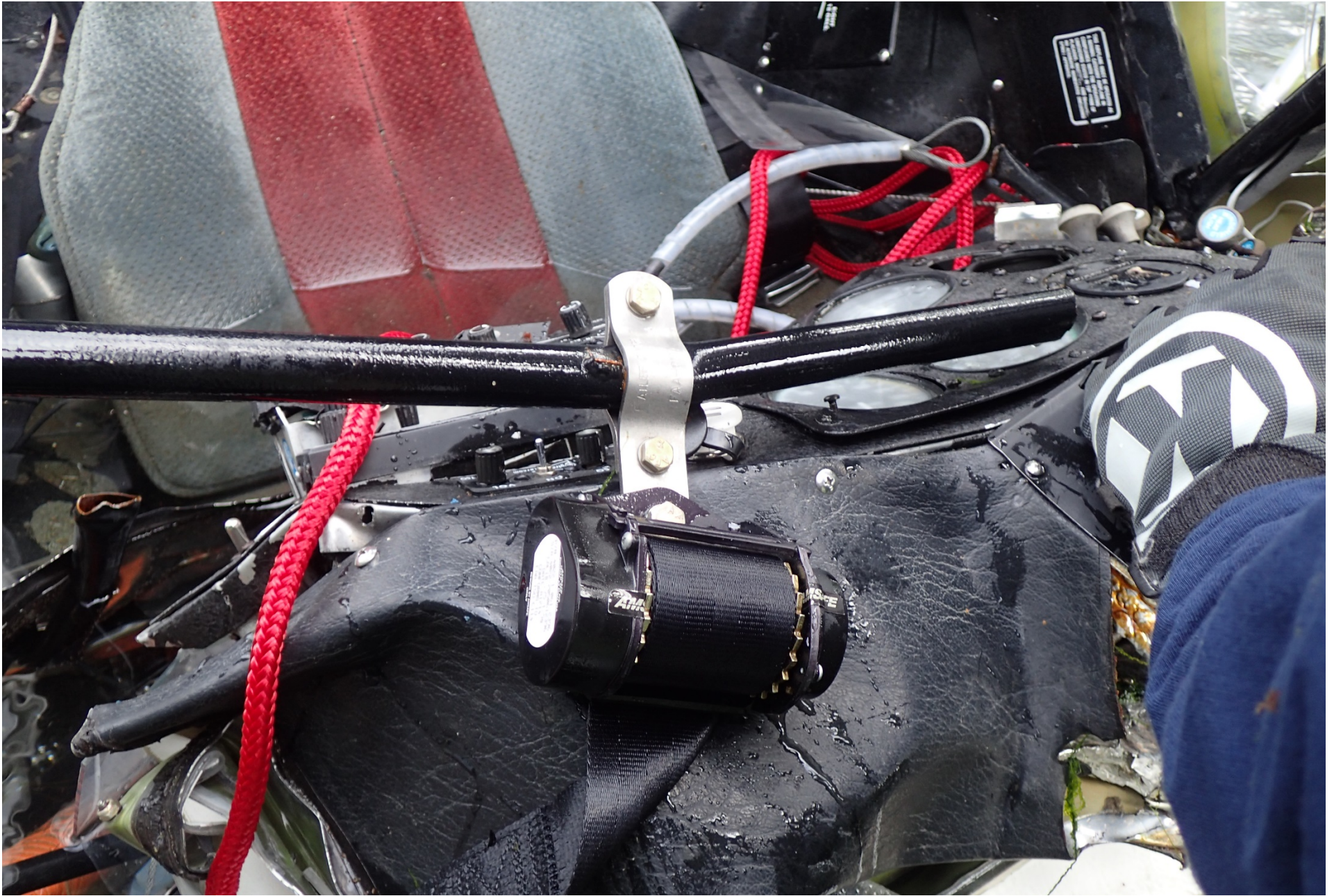
Photo 6 - Front seat (pilot's) shoulder harness inertia reel mounted on cut tube.
