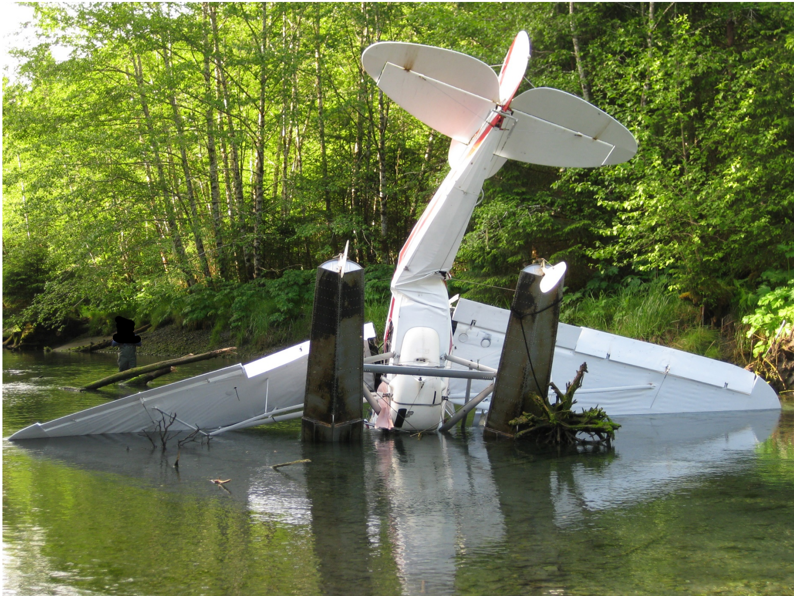
Photo 5 - Rear view of wreckage exhibiting right twist and displacement in aft fuselage.
