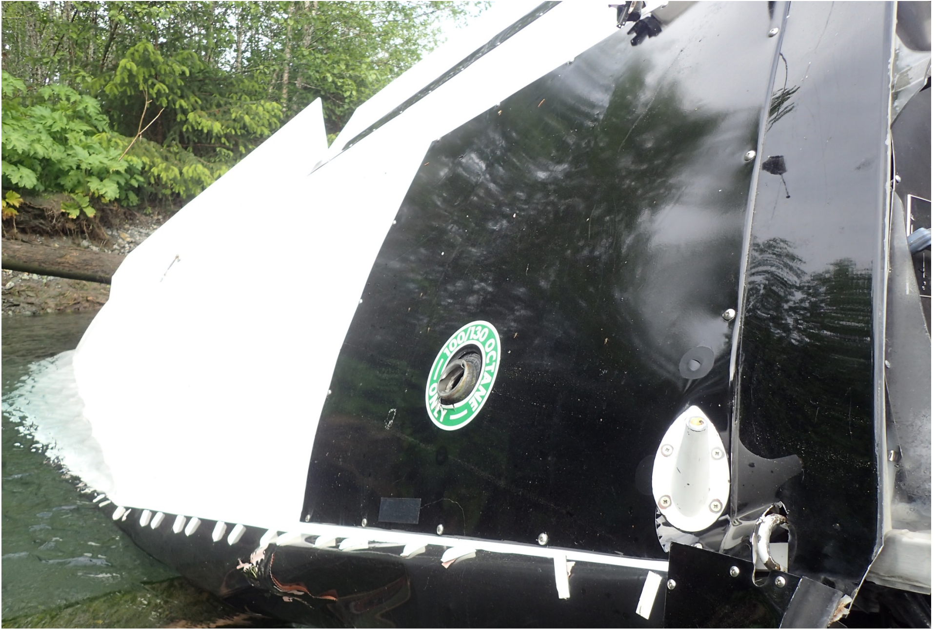
Photo 4 - Right wing with missing fuel tank cap.
