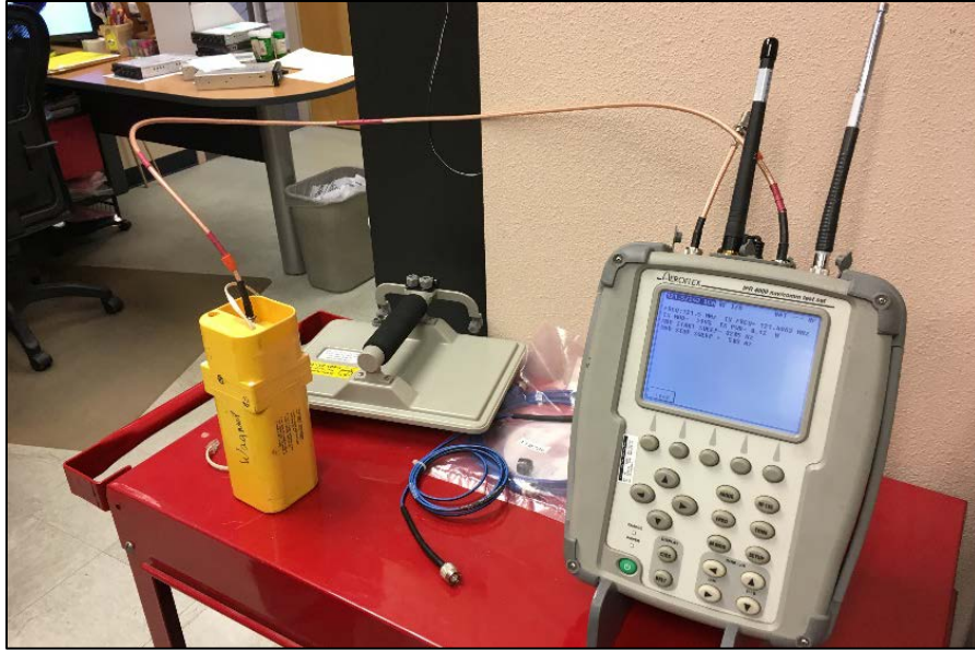
Figure 7. The ELT connected to test set during function testing.
