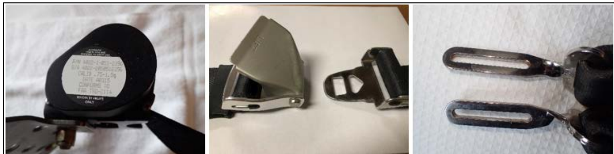
Figure 4. Rear seat restraint system with buckle deformation evident.
