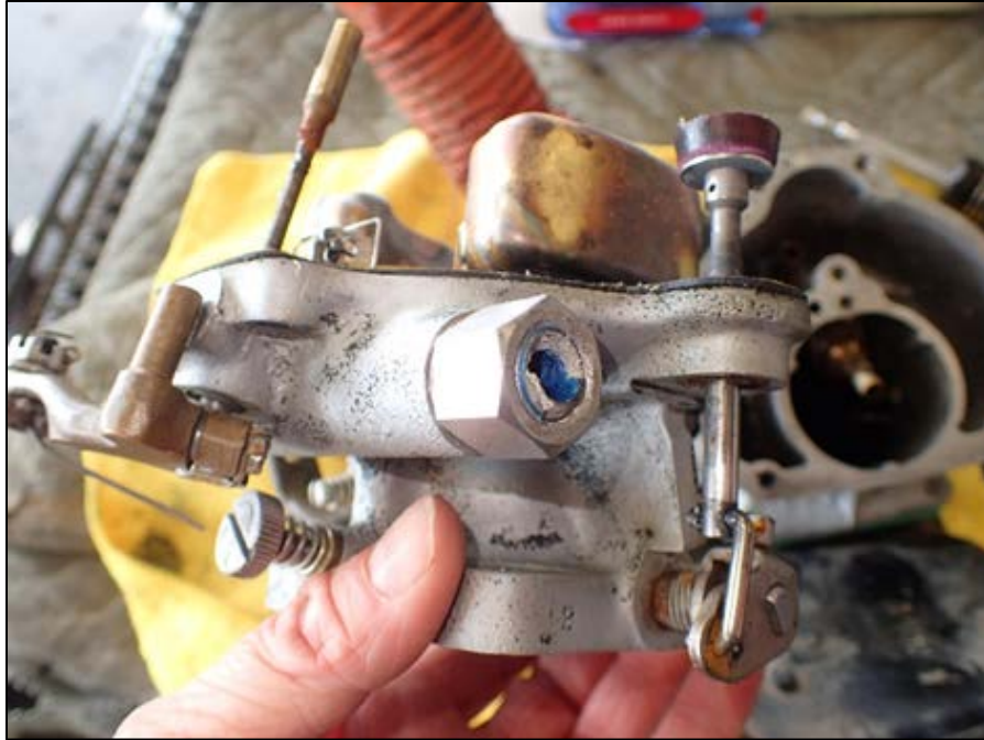
Figure 6. Carburetor indicating fractured inlet fuel line.
