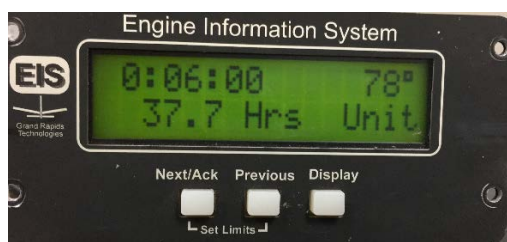
Figure 1. Screen showing a last flight time of 6 minutes and accumulated engine time of 37.7 hours.
