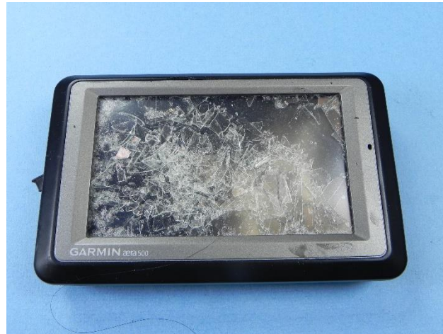
Figure 1. Photo of damaged Garmin Aera 500.
