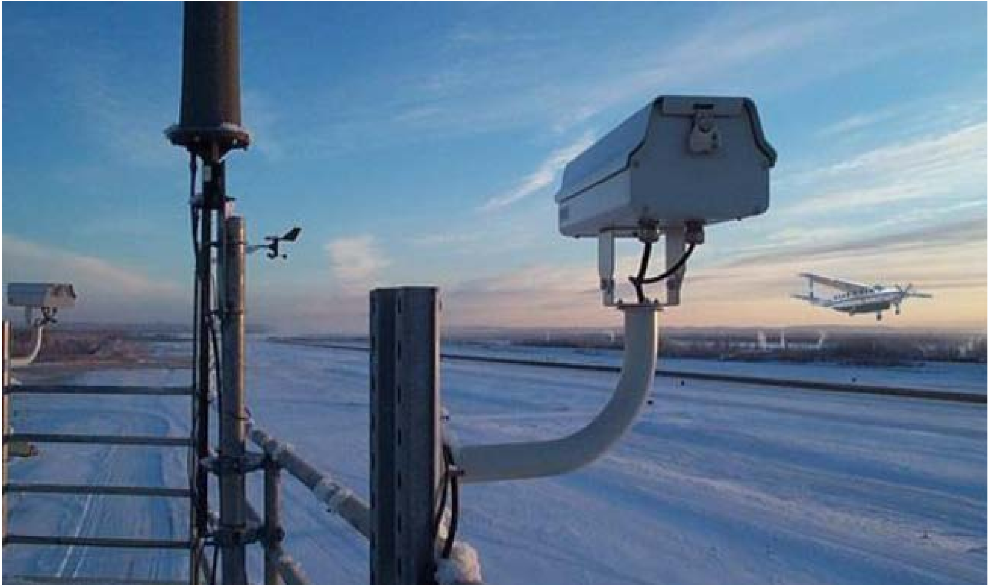
Photo 8 – Exemplar: FAA aviation weather camera in Alaska (courtesy of the FAA).
