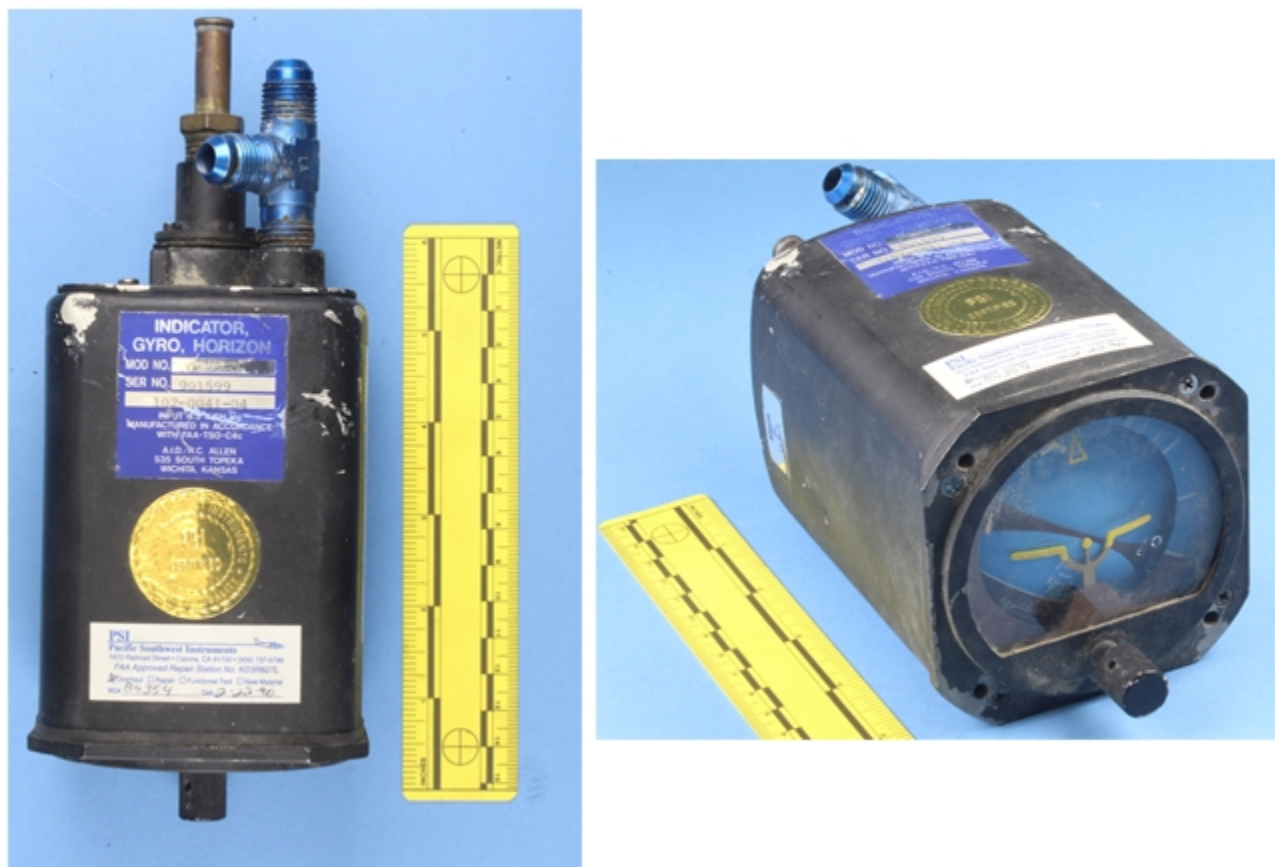
Figure 1. Two views of the as-received attitude indicator.
