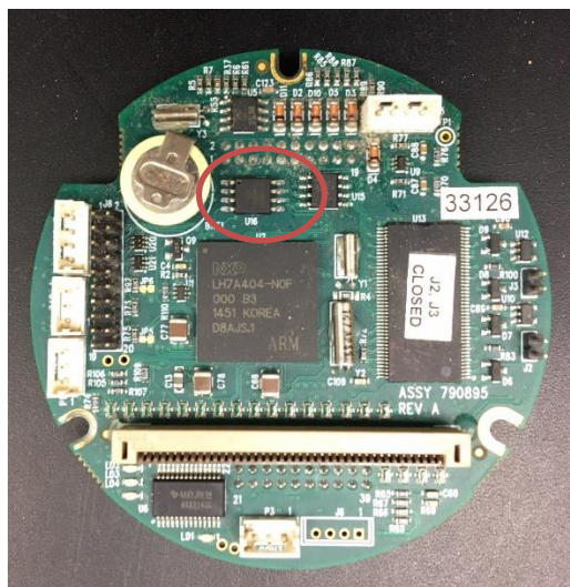
Figure 2. An internal board with the memory chip circled.
