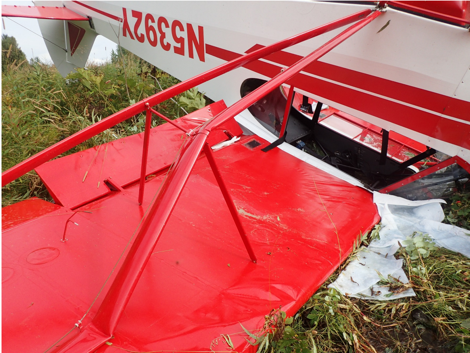
Photo 4 - Damaged left wing lift strut
