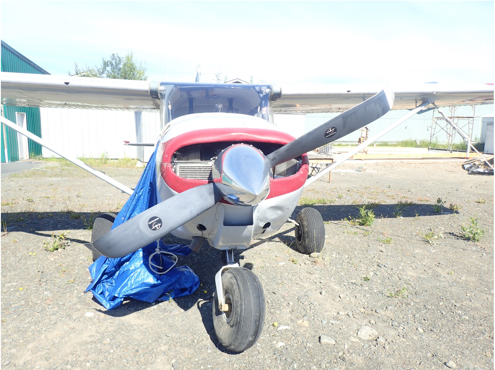
Photo 1 – N5020D propeller and fuselage damage.
