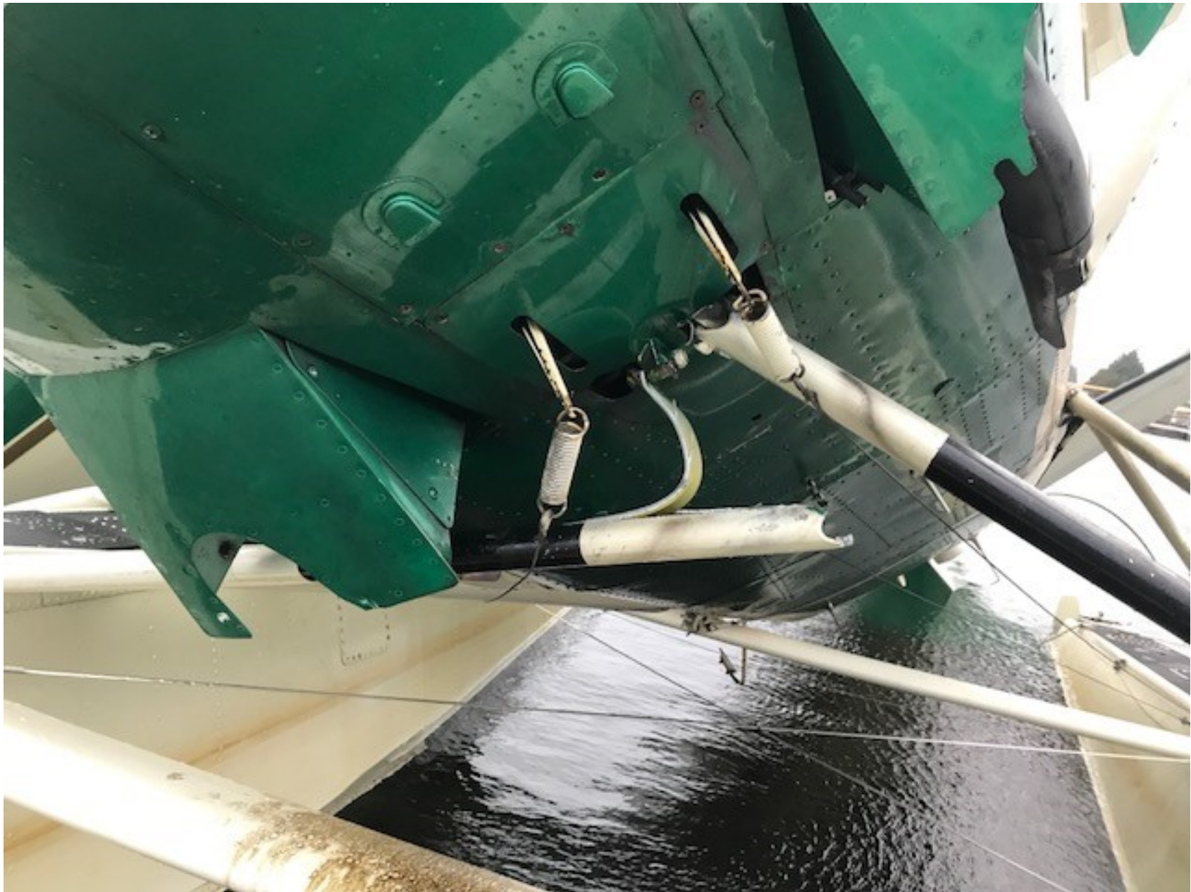
Photo 6 – Accident airplane's separated float struts.
