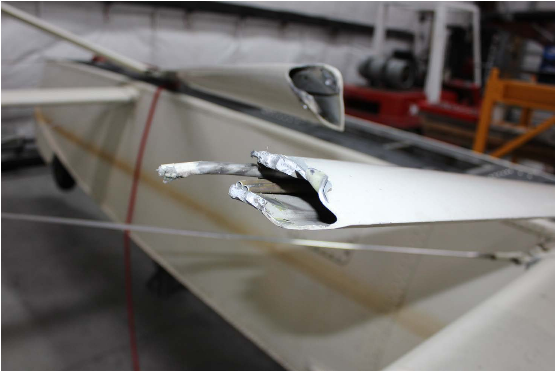
Photo 7 – Accident airplane's right rear float strut and severed hydraulic lines.
