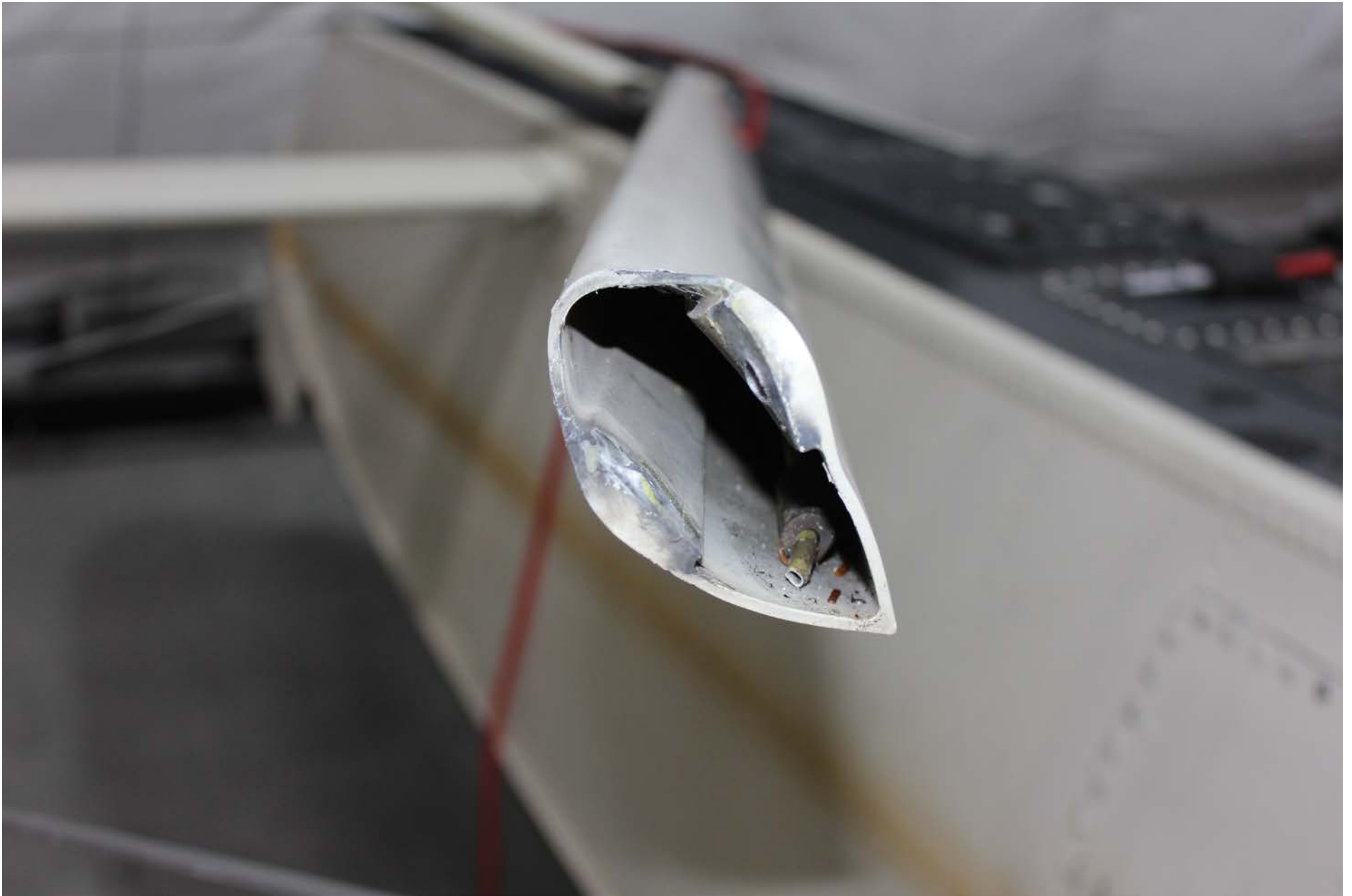
Photo 8 – Accident airplane's right middle float strut and severed hydraulic line.
