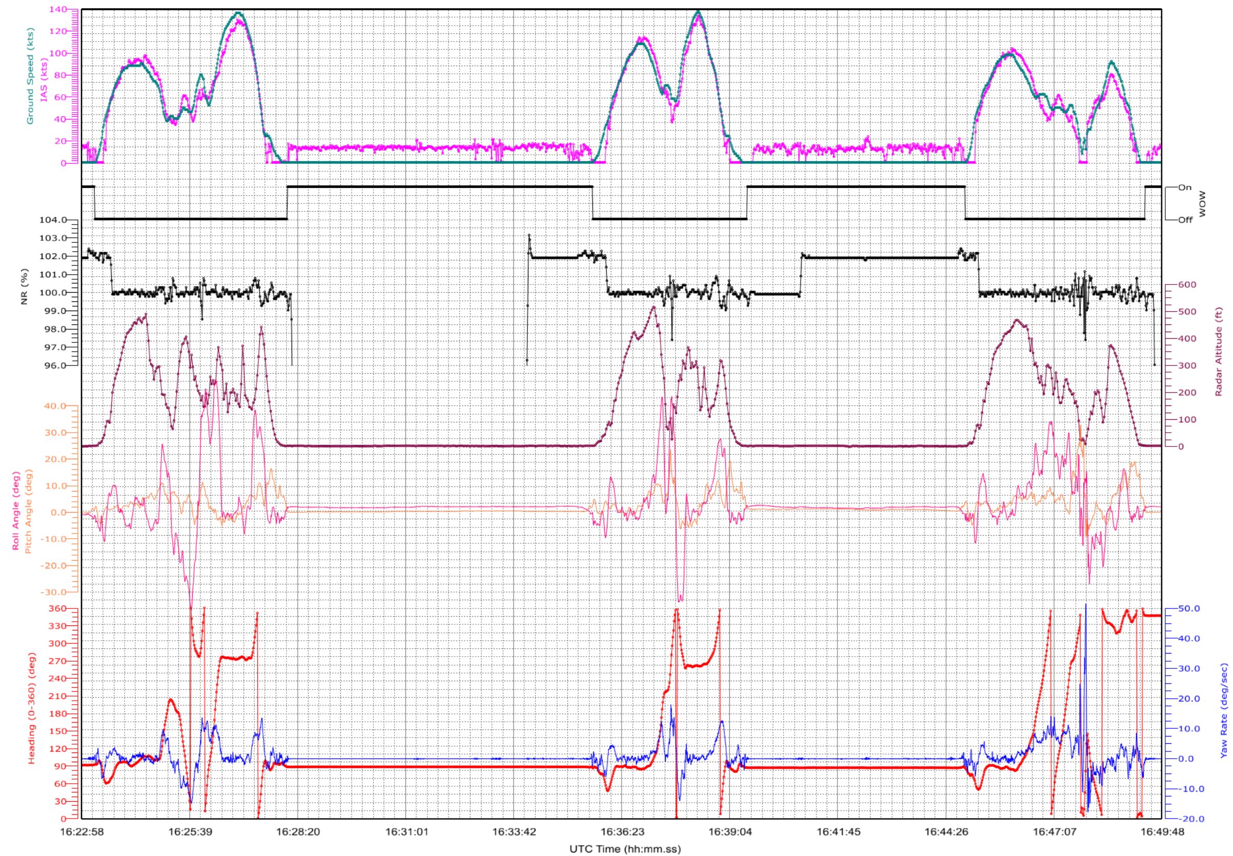
Figure 11 – Time Histories of the A/C main parameters for the last three flights (3/4)
