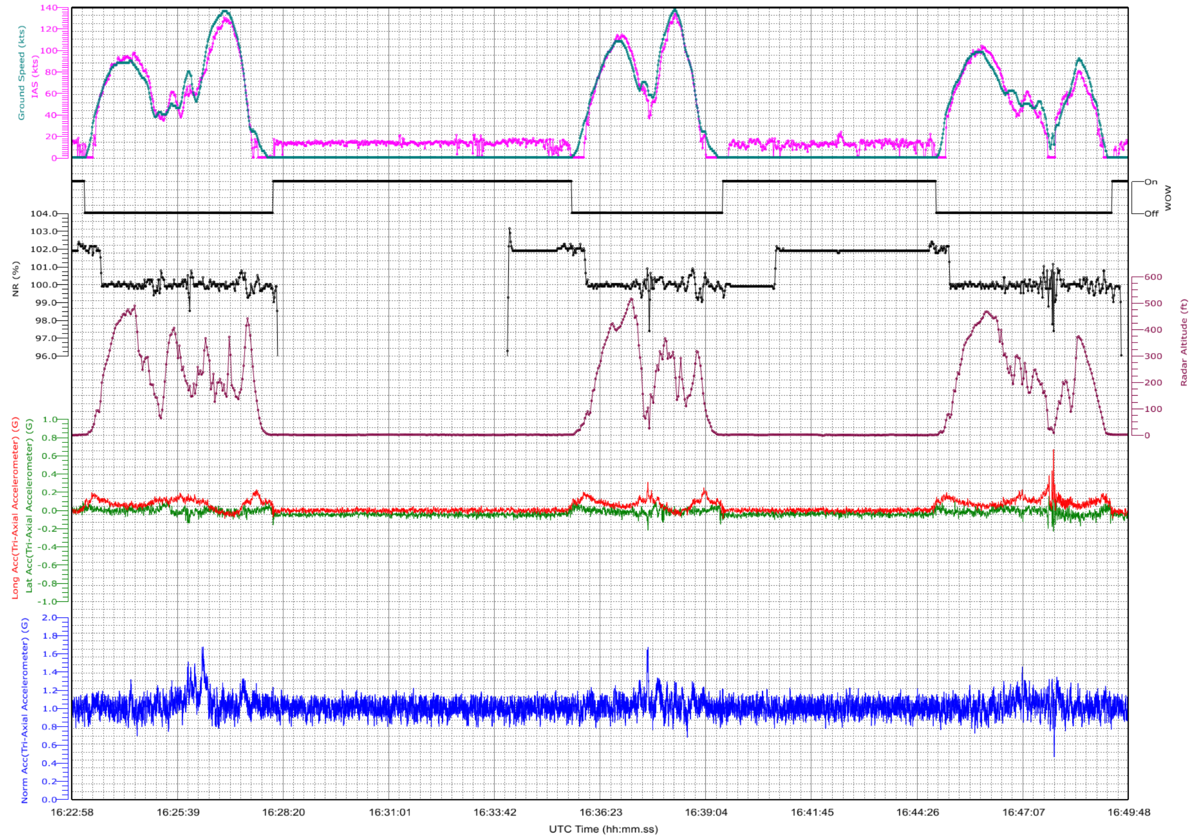
Figure 12 – Time Histories of the A/C main parameters for the last three flights (4/4)
