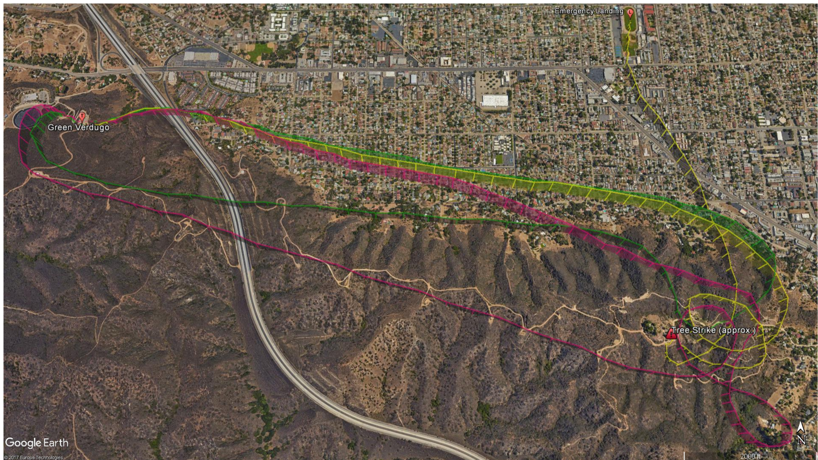
Figure 3 – Flight Path of N304FD (last 3 flights of the recordings: Yellow : Last Flight; Green : 2 nd to last Flight; Magenta : 3 rd to last Flight)
