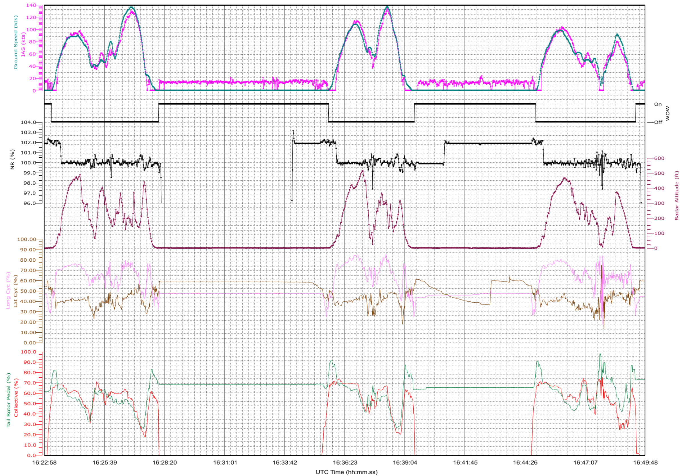
Figure 10 – Time Histories of the A/C main parameters for the last three flights (2/4)
