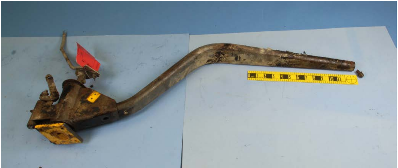
Figure 1: Tail wheel spring assembly and fractured bolt
