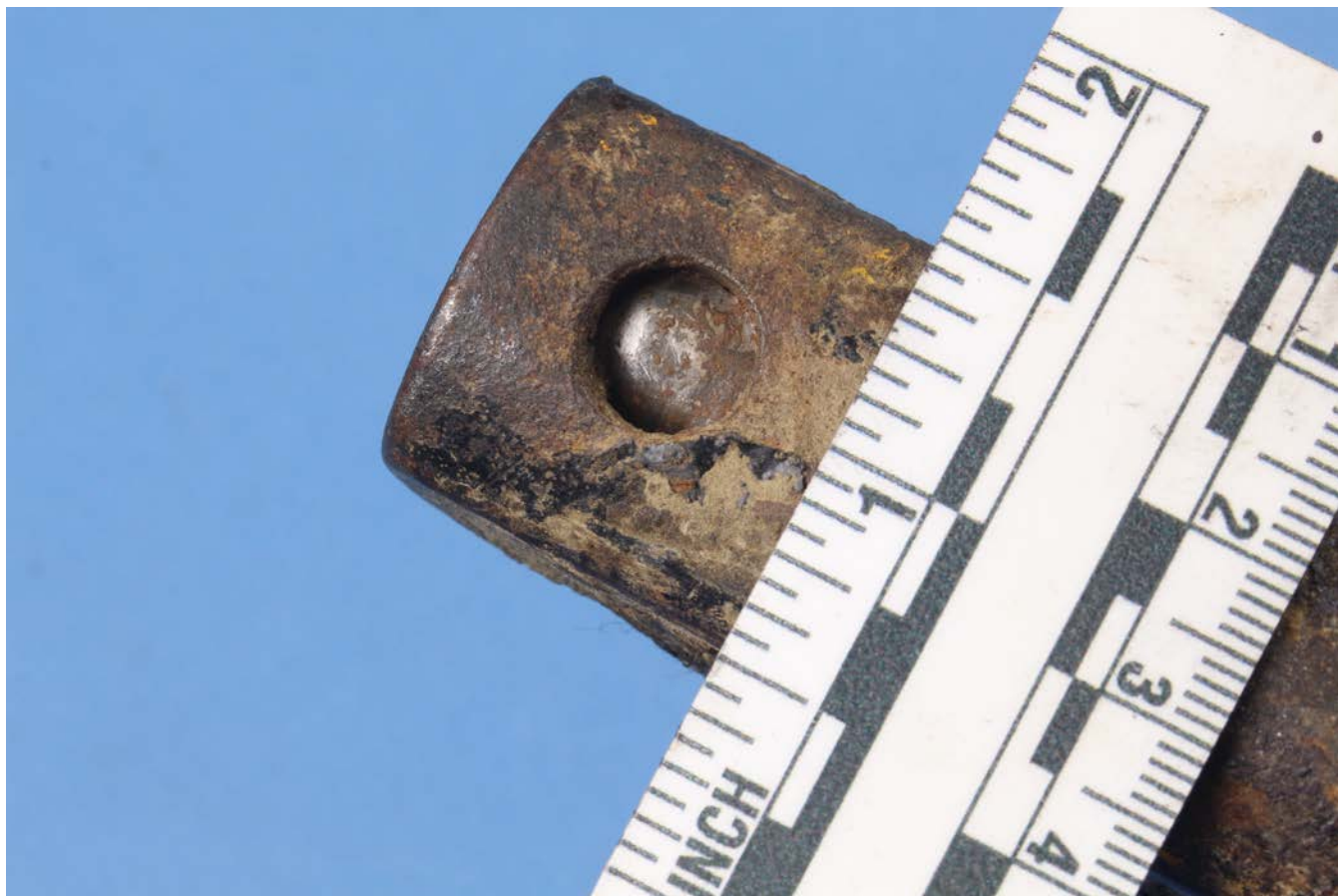
Figure 3: Bolt shank recessed in tail wheel spring's attachment bolt hole.
