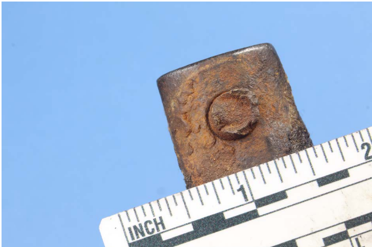
Figure 2: Portion of fractured bolt protruding from the spring's attachment bolt hole.
