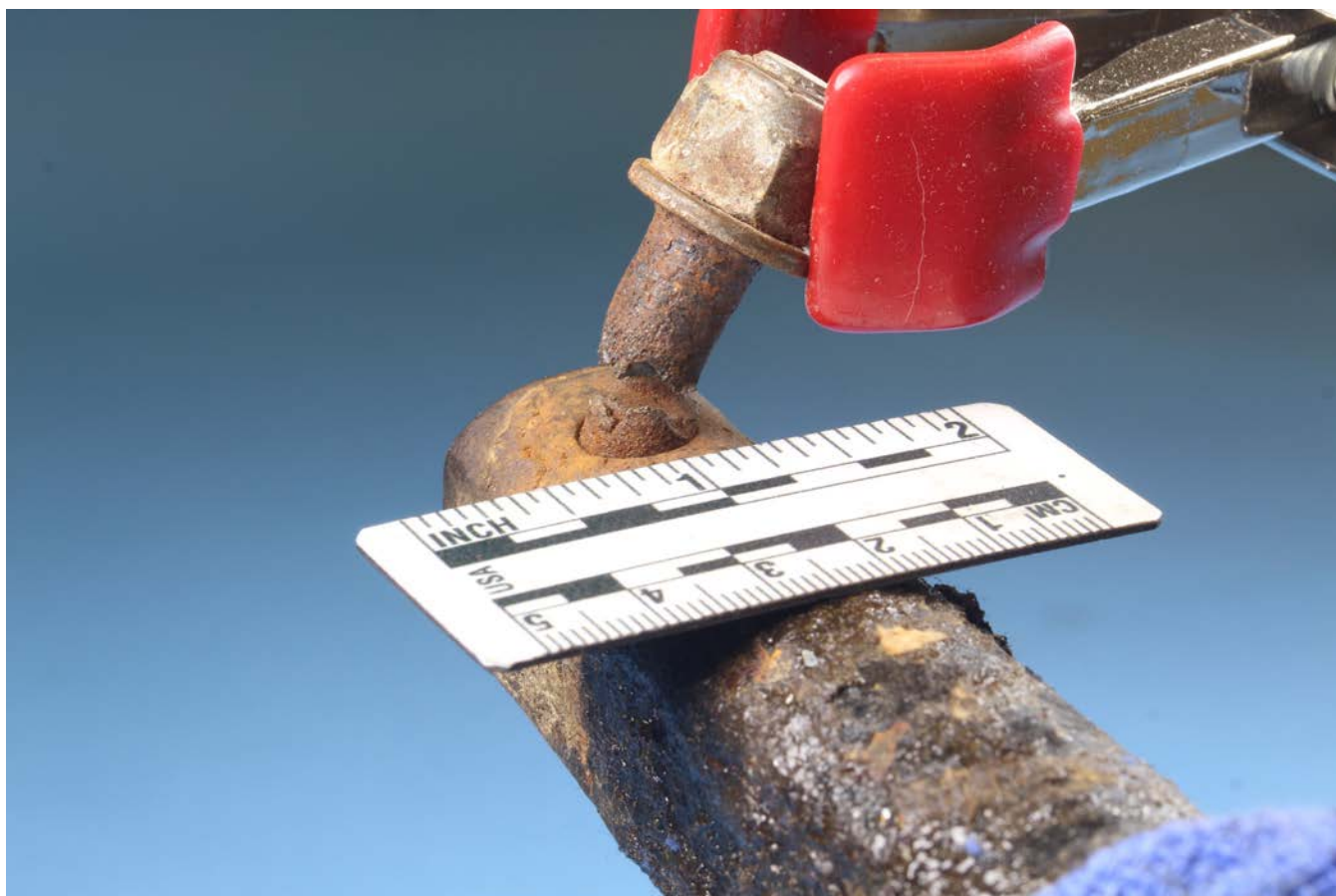
Figure 4: Alignment of protruding bolt shank and recovered portion of attachment bolt.
