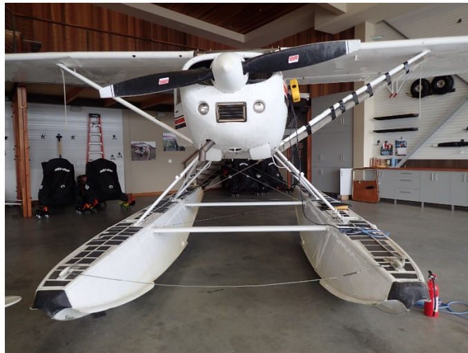
Figure 4. Airplane during the airframe examination with evident lift strut damage.
