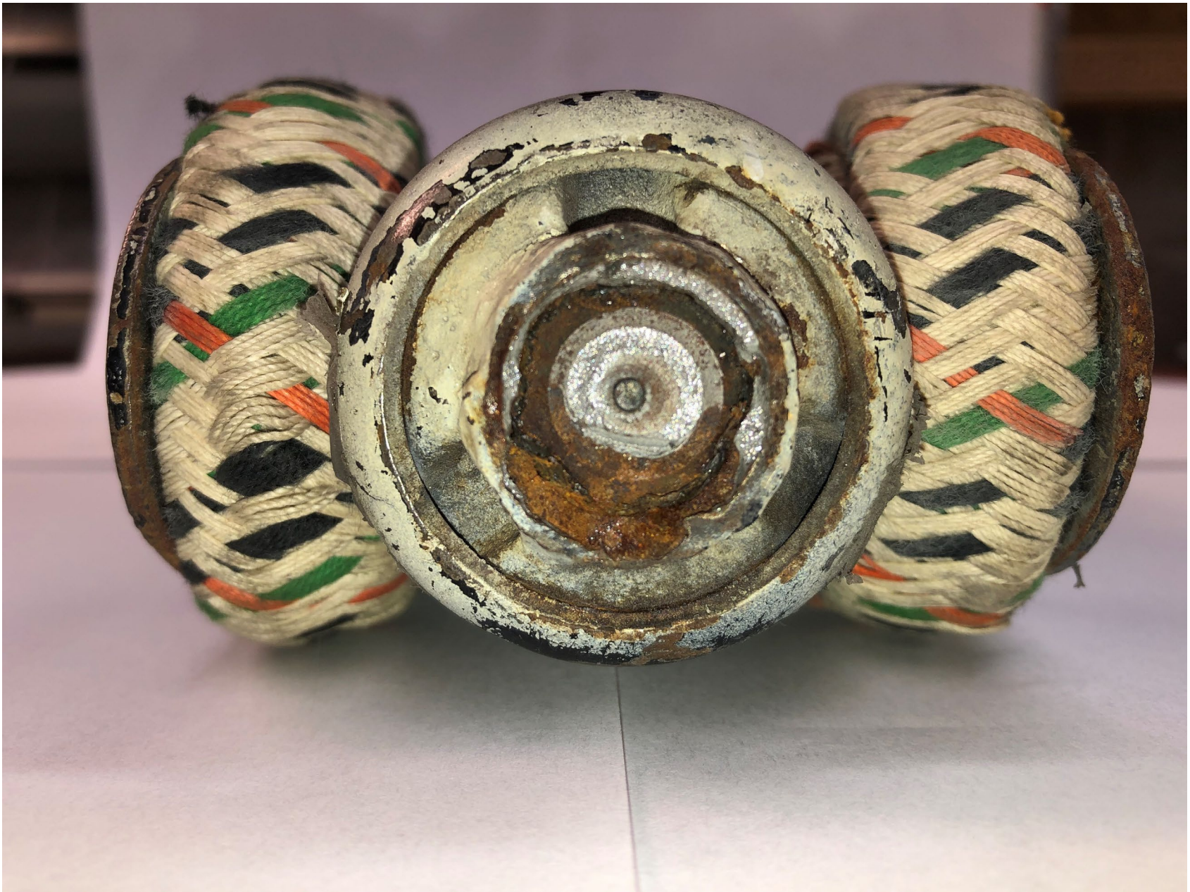
Photo 2 – Fracture Surface of Lug Fitting on Hydrasorb Side
