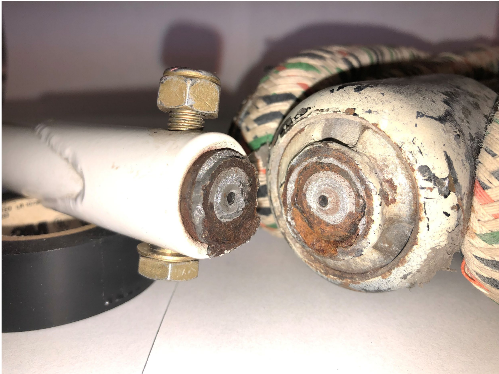
Photo 1 – Both Fracture Surfaces of Lug Fitting
