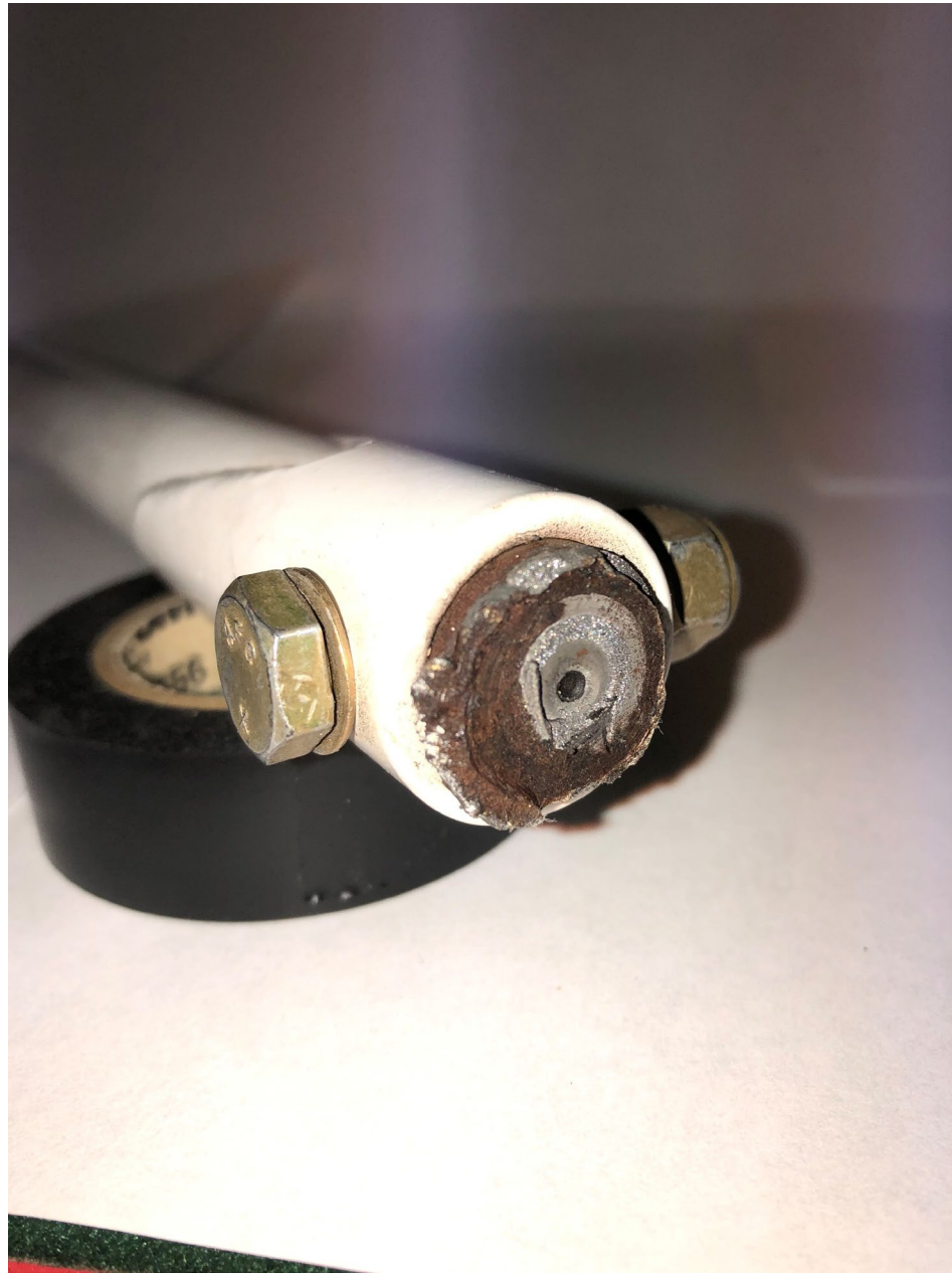
Photo 3 – Fracture Surface of Lug Fitting on Extension Tube Side
