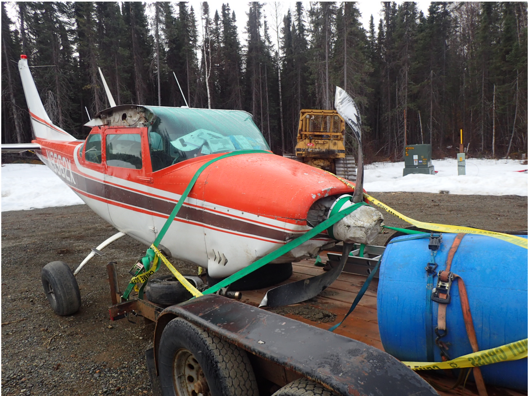
Photo 2 - Airplane at recovery facility before examination with wings removed.
